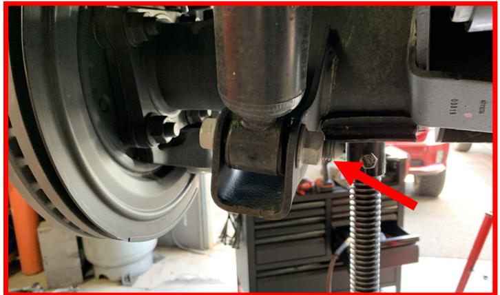
Make sure the axle is properly supported before removing U-bolt nuts.
