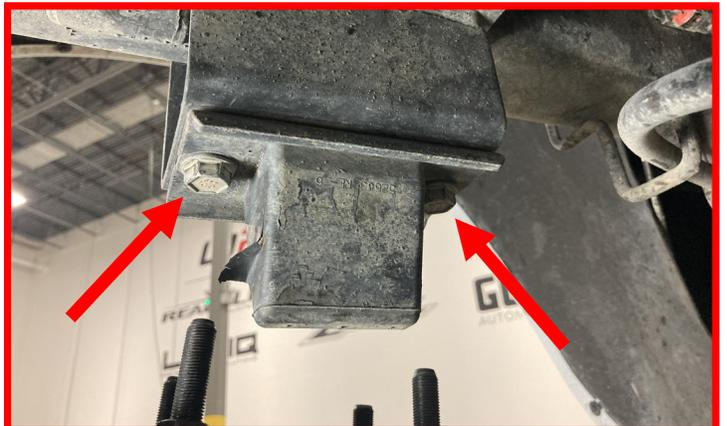
Install the provided bump stop extensions using the provided hardware.
