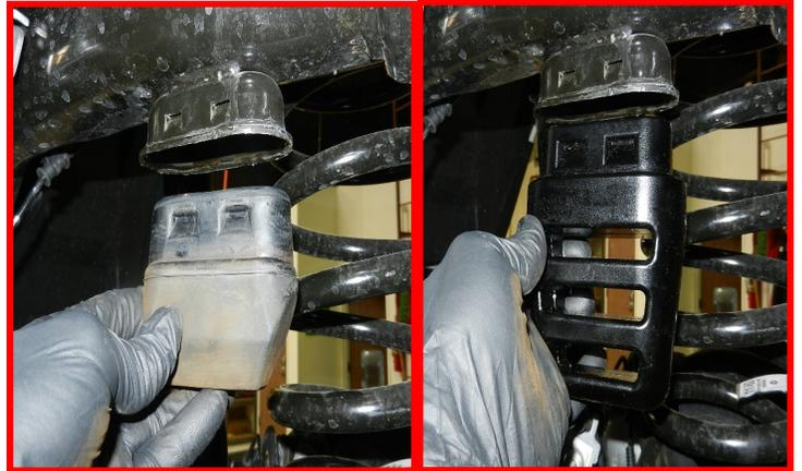
Place the spring isolator onto the **provided lift springs**.
