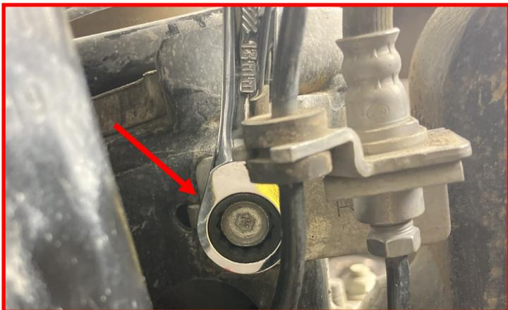
Reinstall the 13mm upper ABS and Brake line bracket bolt located above the radius arm.
