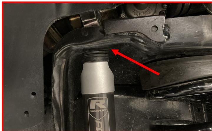
Install the **Falcon front shock** lower mount to the axle mount.
