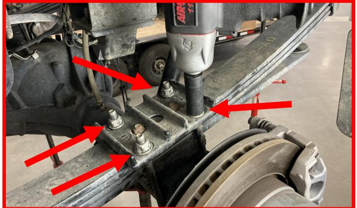
Lower the axle carefully to be able to install the **provided blocks and U-bolts**.
