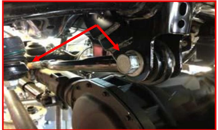
Loosen the rear radius arm bolt.
