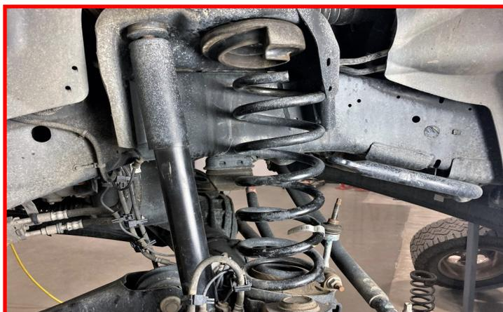
Remove the **factory spring isolator**.
