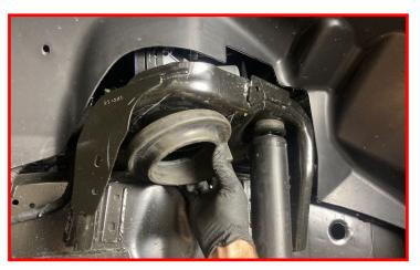
Using thread locker install the (3) supplied 5/16" bolt from the inside out on the supplied spring isolator retainer.
