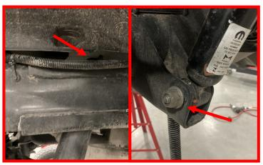
Install the provided rear shocks upper and lower mounting locations on both driver and passenger side using the factory hardware.
