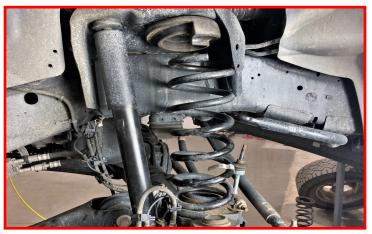
Remove the factory spring isolator.
