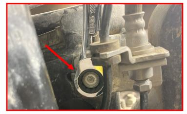
Reinstall the 13mm lower ABS and Brake line bracket bolt located on the axle.
