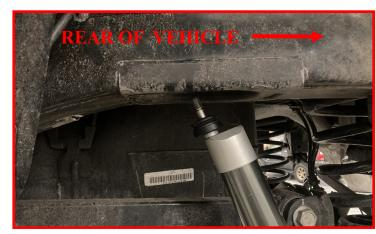
In the correct orientation of the rear shocks the Falcon label should be facing the rear of the vehicle.
