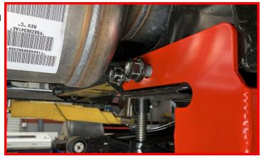
Rotate the axle and install the radius arms into the drop brackets using the provided (2) 18mm hardware.
