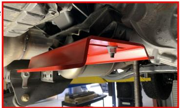
Install the front driveline onto the transfer case. Ensure the retaining clip is fully seated.
