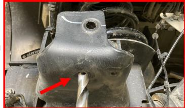
Install the provided rear track bar bracket into the factory rear track bar location using the factory hardware.
