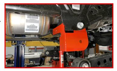
Install (4) provided M16 hardware through crossmember and radius arm drop bracket mounting holes from front to rear of the vehicle. This will aid in removal if service needs to be performed.
