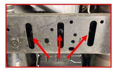
Remove the (3) transmission mounting nuts.
