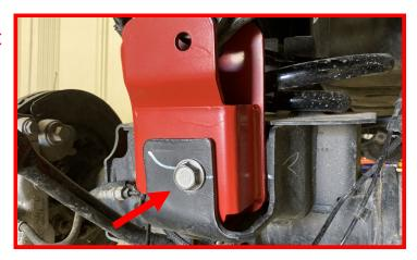
Install provided M14 hardware into the bottom of the rear track bar bracket.
