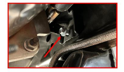
Install the (3) front exhaust hanger mounting bolts.
