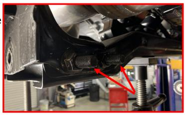
Install radius arm drop bracket using the factory hardware into the factory radius arm bolt hole. Do not tighten at this time. Repeat for the opposite side.
