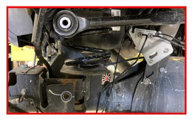
Remove the rear brake line/ wheel speed sensor bracket.
