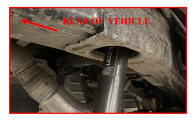
Install the rear Falcon shocks into the axle mounts using the factory hardware.
