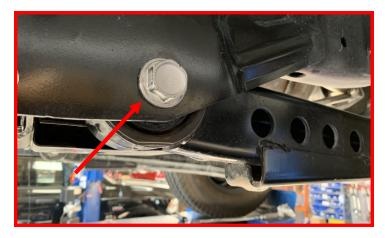
Mark the driveshaft to pinion location.
