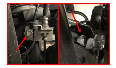
Remove the 18mm nut from the sway bar end link while holding the 8mm bolt so it does not spin.
