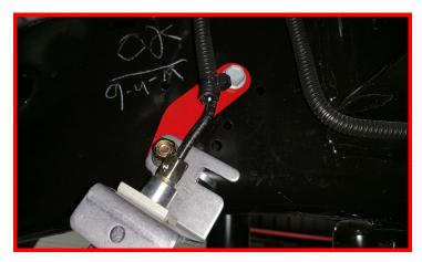
The passenger side bracket will angle around the frame gusset.
