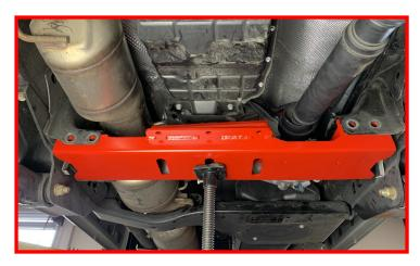
Using the factory transmission crossmember hardware, install the driver side bolts from front to rear.
