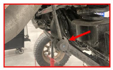
Install the provided sway bar end link upper using the provided hardware.
