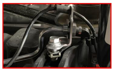
Install the (2) ABS brackets to the axle using factory hardware.
