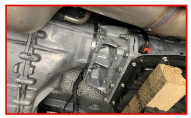
On installation of transfer case it may be necessary to rotate the shaft on the front of the transfer case to match the spline pattern for the back of the transmission.
