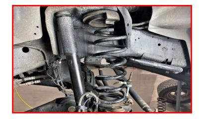
Remove the factory spring isolator.
