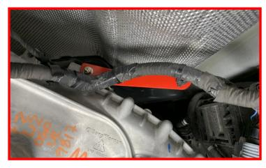
Install the transfer case shift solenoid connector.
