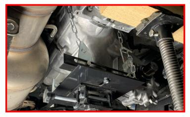
Remove the (8) transfer case mounting nuts.
