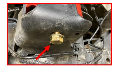
Install the track bar into the top hole on the track bar bracket using the provided M14 hardware.
