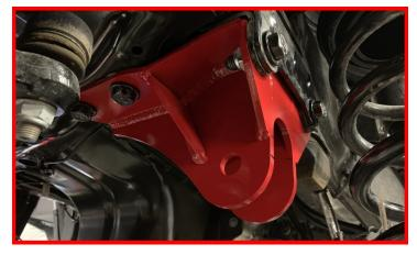
Install track bar using factory hardware.
