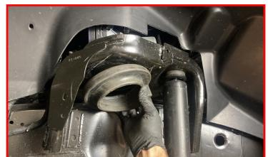
Using an appropriate cutting tool, remove the alignment tab on the coil spring isolator.
