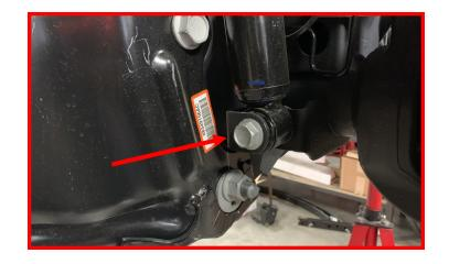
Place a jack under the axle for support. Remove the (2) radius arm bolts.
