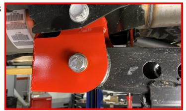
Do not torque the crossmember or radius arm bolts at this time.
