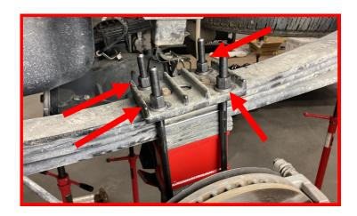
Install the provided rear brake line bracket extension using the upper slots to the factory bracket using the provided M8 hardware. Torque provided hardware to 20 ft-lbs.
