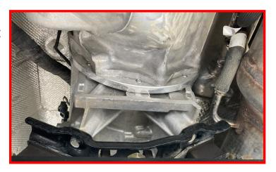
With the transfer case installed and mated back to the transmission, install the (8) provided nuts and washers.
