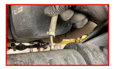
Install the provided rear shocks upper and lower mounting locations on both driver and passenger side using the factory hardware.
