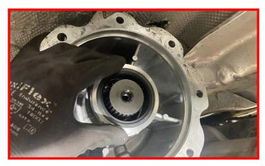
On installation of transfer case it may be necessary to rotate the shaft on the front of the transfer case to match the spline pattern for the back of the transmission.
