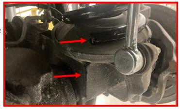
Passenger side ends up with end of the weld on the lower cup to axle/track bar mount.
