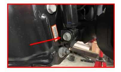
Place a jack under the axle for support. Remove the (2) radius arm bolts.
