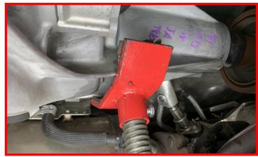
With the transfer case supported, locate the (3) transmission mounting nuts.
