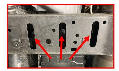
Remove the (3) transmission mounting nuts.
