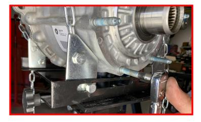
Install the (8) provided transfer clocking ring.
