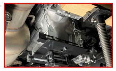
Remove the (8) transfer case mounting nuts.
