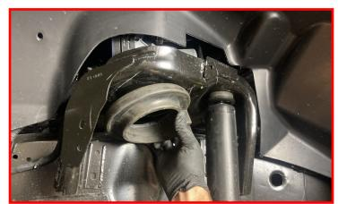
Using an appropriate cutting tool, remove the alignment tab on the coil spring isolator.
