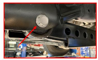
Mark the driveshaft to pinion location.
