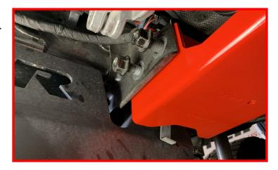
Using the (4) M16 provided hardware install the passenger side bolts from front to rear to avoid hitting the DPF. This will also aid in removal if service needs to be performed.
