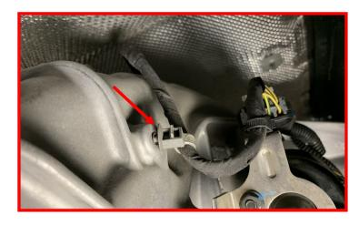
Remove the transfer case harness retaining clip located on the top of the transfer case.
