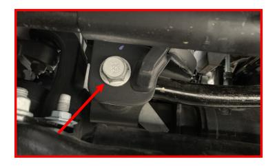
Remove (1) track bar hardware at the frame and swing track bar out of the way.
