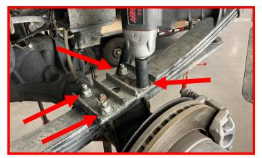
Lower the axle carefully to be able to install the included taper block.
