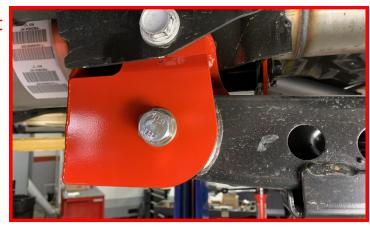
Ensure all transmission crossmember hardware or harnesses are clear and remove the transmission crossmember.
