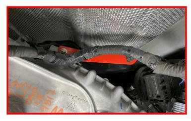
Install the transfer case shift solenoid connector.
