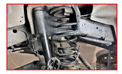
Remove the factory spring isolator.
