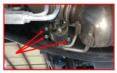
Remove the (2) center exhaust hanger mounting bolts.
