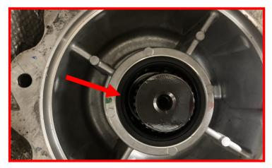
Install the provided transfer case spacer.
