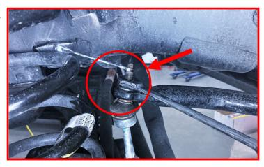
Loosen but do not remove the lower shock mounting bolts.
