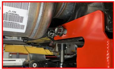
Rotate the axle and install the radius arms into the drop brackets using the provided (2) 18mm hardware. Do not tighten at this time.
