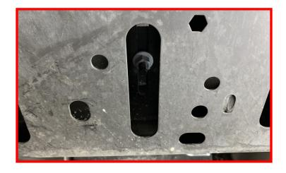
Remove the harness mounting clips attached to the front of the transmission crossmember.
