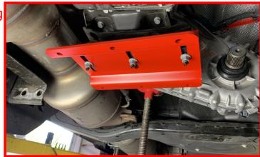
Ensure that the mount is installed with the slope facing towards the rear of the vehicle.
