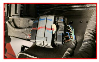
With the connector out of the way, install the connector relocation bracket using the supplied M6 x 20mm bolt, locking nut and washers.
