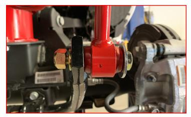
Install the parking brake cable bracket using the factory hardware.
