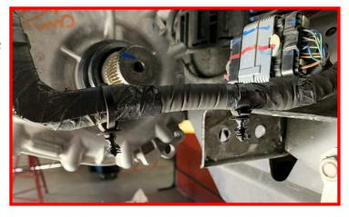
Using a suitable jack, support the transfer case.
