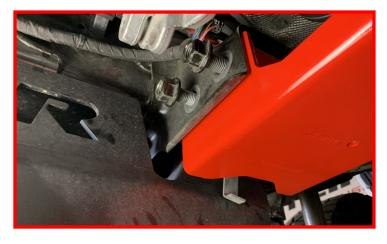
Using the factory transmission crossmember hardware install the passenger side from front to rear. This will aid in removal if service needs to be performed.
