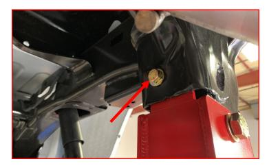
Drill hole on outside of factory track bar mount using 3/8" drill. Install the 3/8" bolts, washers and c lock nut on the outside hole. Tighten 3/8" hardware and torque to 45 ft-lbs. Torque the factory hardware to 100 ft-lbs.
