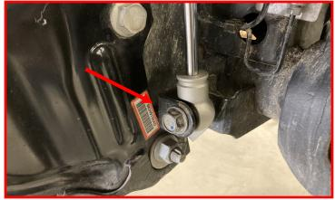
You will now be able to install the sway bar end link while lifting the axle into place.
