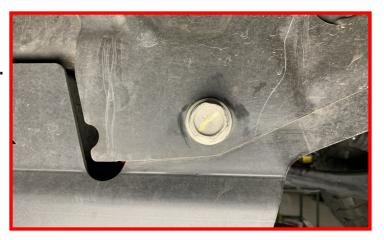
Remove the driver side transmission crossmember bolts and retain factory hardware.
