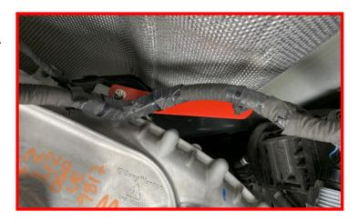
Install the transfer case shift solenoid connector.
