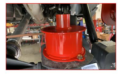
Install the replacement rear coil springs with factory isolators onto the spacers. Raise axle to hold coil springs in place.
