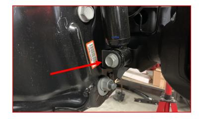
Place a jack under the axle for support. Remove the radius arm bolts. Retain factory hardware.
