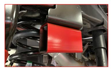
Install the bump stops using 3/8" bolts, washers and c-lock nuts.
