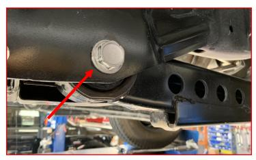
Mark the driveshaft to pinion location. Remove the front driveshaft from the axle. Let hang out of the way.
