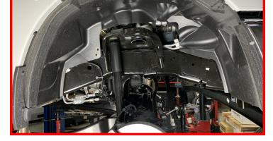
Remove the (5) factory mounting bolts from the factory track bar bracket and remove from vehicle.
