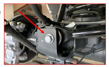
Remove the upper track bar mounting bolt.
