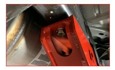
Bend the wires to align the tab nut with the front mounting holes in the bracket and frame. Install the 1/2" bolts and washers.
