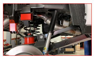
Install the sway bar end links using M12 bolts, washers, and c-lock nuts. Ensure the fender washer is installed on the outside of the bushing. Do not tighten at this time.
