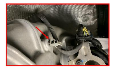
Remove the transfer case harness retaining clip located on the top of the transfer case.
