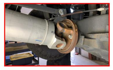
Using the factory hardware and thread locker, install the drive shaft to the pinion flange lining up the previous marks.
