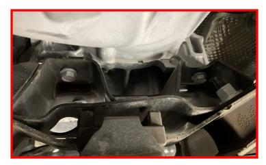
Tighten the transmission mount bolts.
