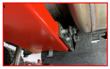
Install (3) supplied M12 bolts, (3) locking nuts and (6) flat washers through the rear holes on the transmission mounting plate, mounting plate spacer and the transmission crossmember. Do not tighten at this time.
