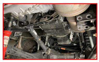
The transmission mount is attached with (4) bolts. Remove the (2) bolts located at the rear of the mount and retain the factory hardware.
