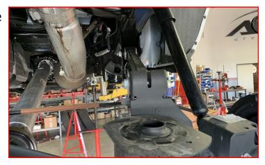
Install track bar bracket using the 14mm x 110mm bolt, washers, and c-lock nut and crush sleeve in the track bars original location.
