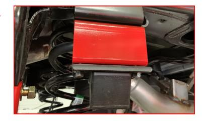
Install the provided Falcon rear shocks using the factory hardware on the bottom and the provided hardware on the top of the shock. Do not tighten at this time.
