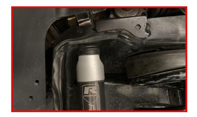
Install the Falcon front shock lower mount to the axle mount using the factory hardware.
