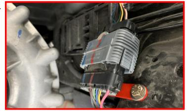
Install the harness relocation bracket using the supplied M6 x 25mm bolt, locking nut and washers into the hole that the retaining clip was removed from.
