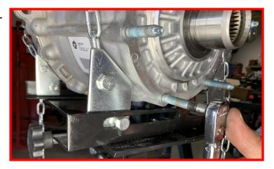
Install the supplied transfer clocking ring. It may be necessary to rotate the ring until all the mounting holes align.
