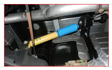
Install the rear wheels and lower vehicle to the ground. Torque the lug nuts to the wheel manufacturer specs. Torque the upper shock stem to 30 ft-lbs, lower shock bolts to 90 ft-lbs, sway bar end links to 45 ft-lbs, bump stop extension to 30 ft-lbs, parking brake bracket 10 ft-lbs, track bar mounting bolts to 100 ft-lbs and the upper and lower control arm bolts to 200 ft-lbs.
