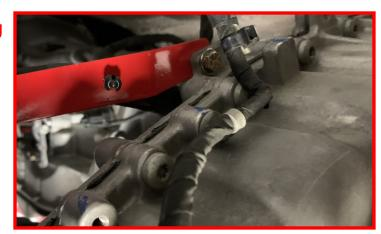
Using a suitable jack, support the transfer case again. Be sure to allow yourself ample room around the transfer case.
