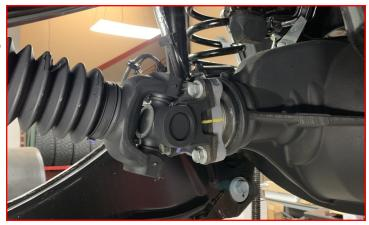
Rotate the axle to release radius arms from the mounting location.
