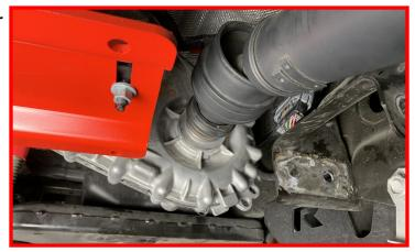
Slide the dust boot back over the front output splines.
