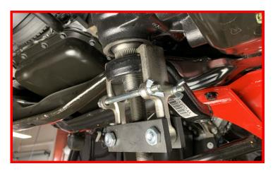
Note: Be sure to thoroughly clean splines prior to installing pitman arm replacement.
