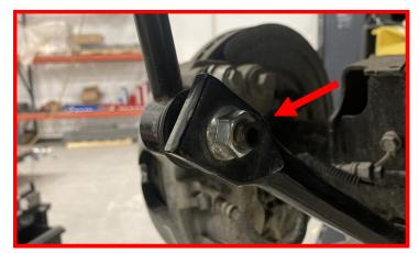
Drill out existing factory track bar bracket lower left hole using a 9/16" drill bit.
