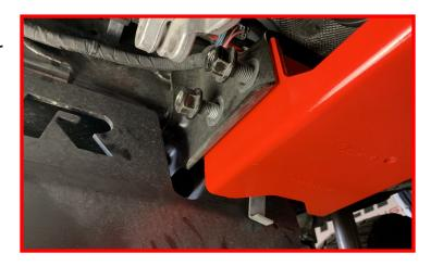
Using the factory hardware bolts install the passenger side bolts from front to rear to avoid hitting the DPF. This will also aid in removal if service needs to be performed.
