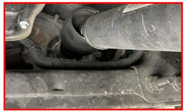
Support the transmission crossmember with a suitable jack stand. Working on one side at a time, Loosen and remove two transmission crossmember bolts.
