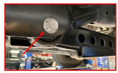
Mark the driveshaft to pinion location.
