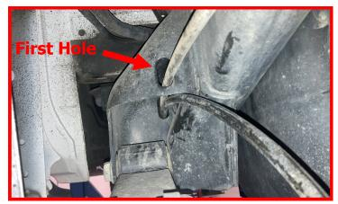
Reinstall the cable housing connector and then re-attach the cable hook.
