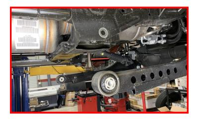
Locate and install the provided radius arm drop brackets using the factory hardware at the main mounting locations.
