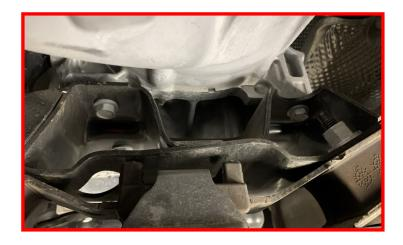
Tighten the transmission mount bolts.
