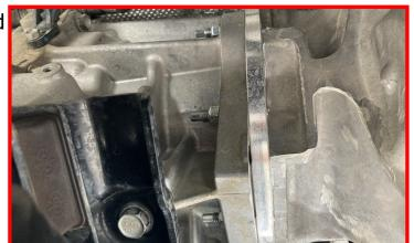
Remove the transfer case harness clip that is located on the driver side of the transmission.
