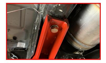
Rotate the axle until the radius arms are lined back up into the drop brackets. Install using the provided M18 hardware.
