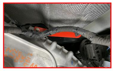
Install the transfer case shift solenoid connector.
