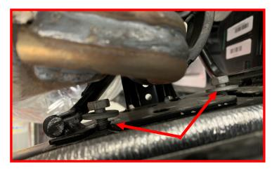
Install the (2) center exhaust hanger mounting bolts.
