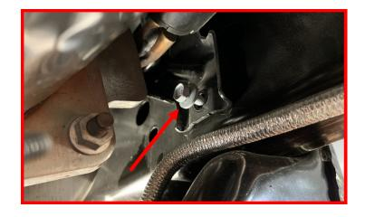
Install the (3) front exhaust hanger mounting bolts.
