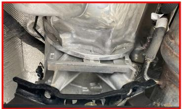
With the transfer case installed and mated back to the transmission, install the (6) provided nuts and washers.
