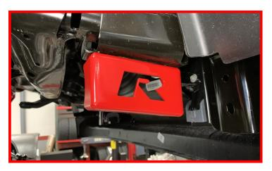
Install the sway bar to the drop brackets using the provided 7/16" hardware.
