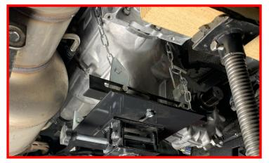
Remove the (6) transfer case mounting nuts.
