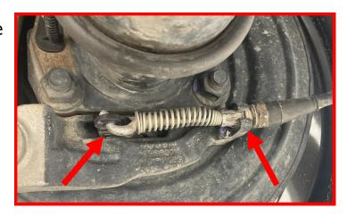
Once the cable is loose you will be able to back-feed the cable through the first frame rail hole you see.
