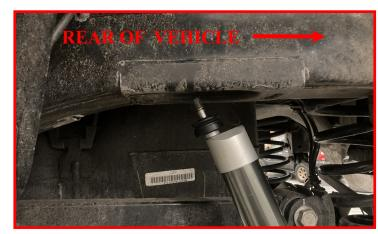
In the correct orientation of the rear shocks the Falcon label should be facing the rear of the vehicle.
