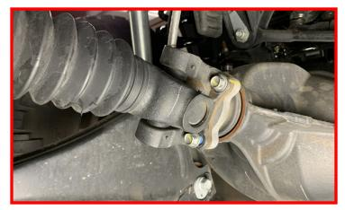
Install the front wheels. Lower the vehicle to the ground. Torque the lug nuts to the wheel manufacturers specs. Torque the lower shock hardware to 90 ft-lbs., the radius arms and track bar hardware to 200 ft-lbs.
