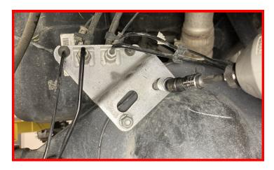
Remove the (2) brake line clips on the back side of the axle.
