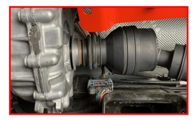
Install the provided clamp onto the dust boot and joint housing.
