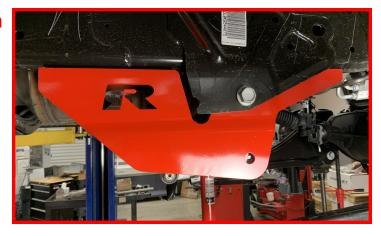
Locate the (4) provided wire flag nuts and the (4) holes on the outside of the frame. Bend the wires to align the tab nut with the rear mounting holes in the bracket and frame.
