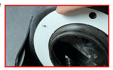
Center punch the marks and using an appropriate tool, drill the 1/2" holes through the spring tower.
