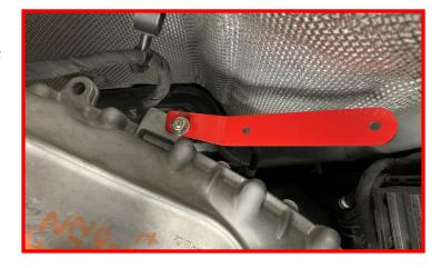
Install the harness that was attached to the top of the transmission crossmember onto the harness relocation bracket.
