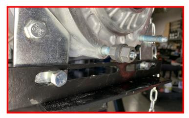
Option 2: Using the splines and an appropriate socket, unthread the stud.
