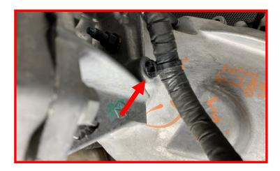
Remove the harness connection from the driver side transmission crossmember mounting.
