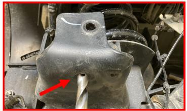
Install the provided rear track bar bracket into the factory rear track bar location using the factory hardware.
