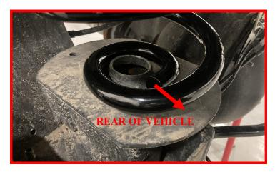
Install the provided Falcon rear shocks into the upper mounts and make sure they are positioned in the correct orientation shown in the picture.
