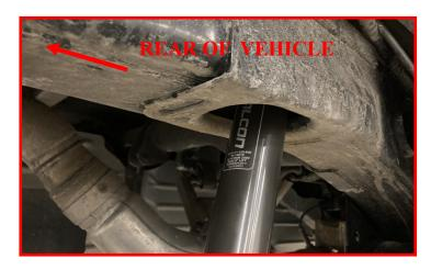
Install the rear Falcon shocks into the axle mounts using the factory hardware.
