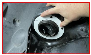
Using a marker or paint marker, Mark the location of the small hole. This is to be where you will drill the new mounting hole.
