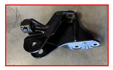
Install provided track bar drop bracket using factory hardware and provided M14 hardware.
