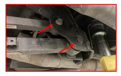
Loosen the (4) axle side control arm bolts.
