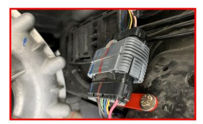
Install the harness relocation bracket using the provided M6 hardware into the hole that the retaining clip was removed from.
