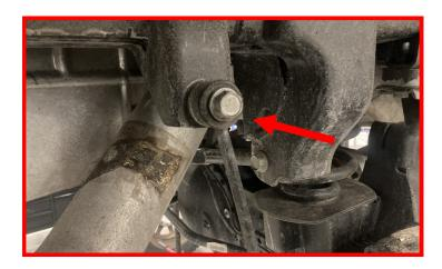
Remove the factory sway bar end link lower hardware.
