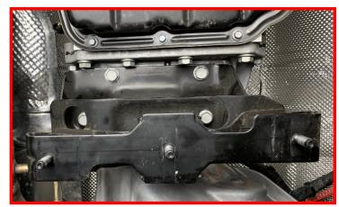
Install the provided transmission mounting plate using the (3) factory transmission mount nuts.
