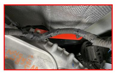
Install the transfer case shift solenoid connector.
