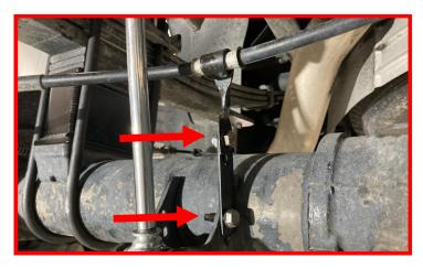
Remove the tree connector holding the top of the axle breather tube and secure it in a lower position using the factory connector and the provided hardware.
