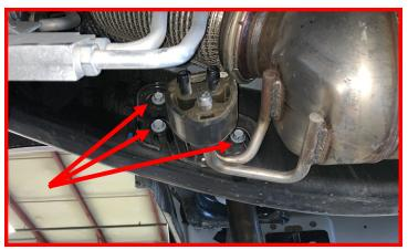
Remove the (2) center exhaust hanger mounting bolts.
