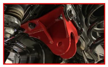
Install track bar using factory hardware.
