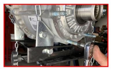
Install the provided transfer clocking ring. It may be necessary to rotate the ring until all the mounting holes align. Install the provided M10 flat head bolts using thread locker.
