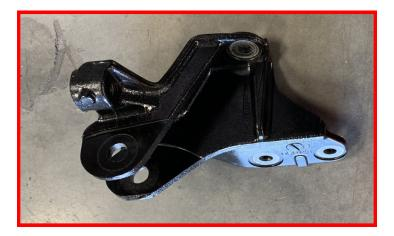
Install provided track bar drop bracket using factory hardware and provided M14 hardware.
