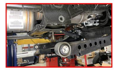
Locate and install the provided radius arm drop brackets using the factory hardware at the main mounting locations.
