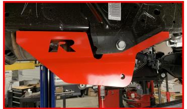
Locate the (4) provided wire flag nuts and the (4) holes on the outside of the frame. Bend the wires to align the tab nut with the rear mounting holes in the bracket and frame.
