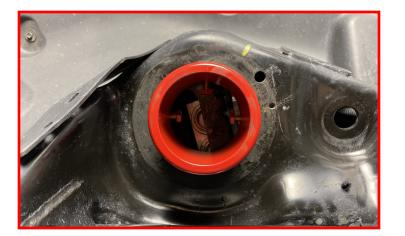
Install spring isolator over the retainer, ensure the alignment tab is installed into new clocking hole.
