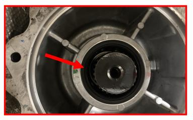
Install the provided transfer case spacer.
