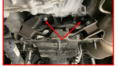
The remaining (2) bolts are located at the front of the mount. Remove the (2) bolts and remove the mount.
