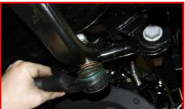
Loosen but do not remove track bar bolt at the axle.
