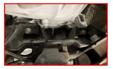
Tighten the transmission mount bolts.
