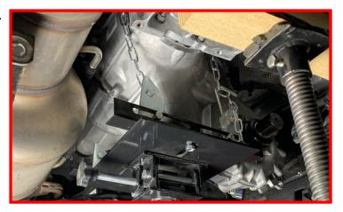
Remove the (8) transfer case mounting nuts.
