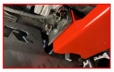
Using the (2) provided hardware bolts install the passenger side bolts from front to rear to avoid hitting the DPF. This will also aid in removal if service needs to be performed.
