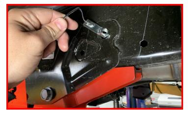
Tighten the provided 1/2" bolts first, ensure the drop bracket is resting flush against the frame rail when doing so.
