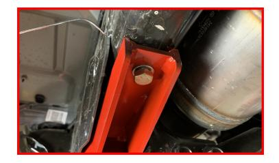
Rotate the axle until the radius arms are lined back up into the drop brackets. Install using the provided M18 hardware.
