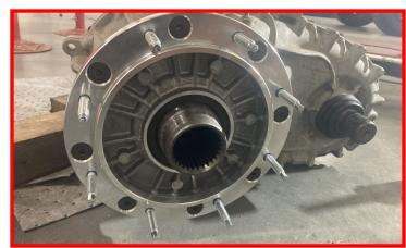
Remove the factory seal inside the transmission housing.
