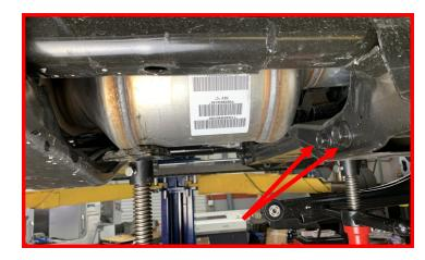
Lower jack and install the (2) Diesel Exhaust Fluid (DEF) tank crossmember exhaust hanger bolts.
