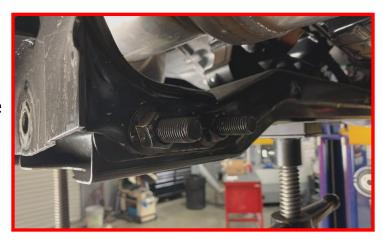
Remove the (3) front exhaust hanger mounting bolts. Retain factory hardware.
