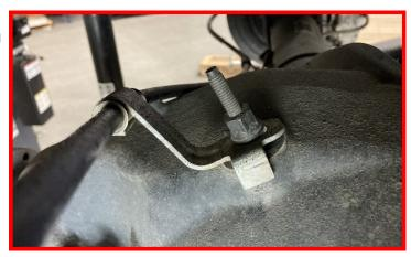
Remove the e-brake cable bracket near the passenger lower shock mount.
