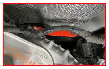
Install the transfer case shift solenoid connector.
