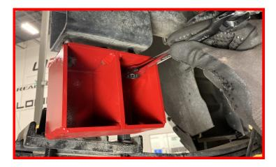
Install the bump stops using the provided hardware.
