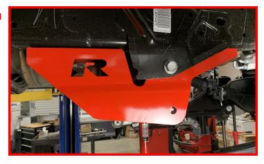
Locate the (4) provided wire flag nuts and the (4) holes on the outside of the frame. Bend the wires to align the tab nut with the rear mounting holes in the bracket and frame.
