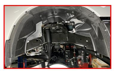
Remove the (5) factory mounting bolts from the factory track bar bracket and remove from vehicle.
