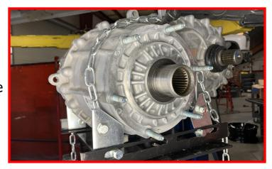
Once the transfer case is removed from vehicle, remove the factory mounting studs. There are two ways to remove the studs.
