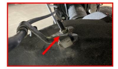
Install the provided e-brake bracket extension to the factory bracket with the provided hardware.
