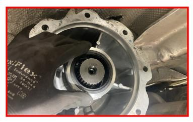
Install the transfer case. It may be necessary to rotate the shaft on the front of the transfer case to match the spline pattern for the back of the transmission.
