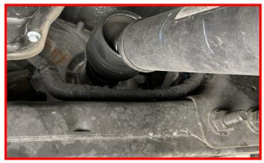
Note: For factory passenger side crossmember bolts that are facing from back to front and the dpf is in the way of removal. Although this is uncommon on most trucks, you may have to remove the dpf hanger bolts and push the dpf up carefully to remove the bolts. Do not reinstall the hanger bolts until crosmember is installed.
