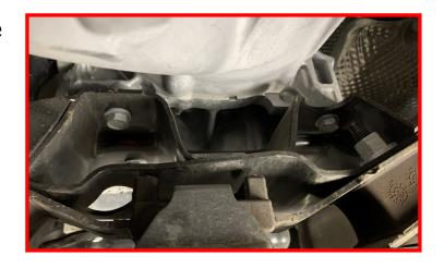
Tighten the transmission mount bolts.
