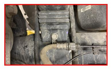
Remove the e-brake cable stud located on top of the differential housing. Once the cable is free re-install the stud.
