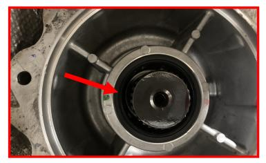
Install the provided transfer case spacer.
