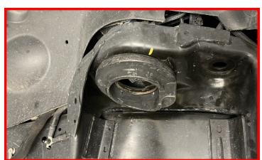
Install the provided coil springs with factory isolators on top. Make sure the isolator is positioned on the flat end of the coil spring. Lower the axle low enough to set both springs in place.
