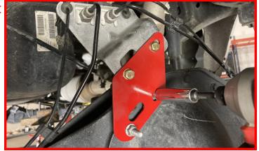
Install the brake line brackets into the back of the tapered block using the factory hardware.
