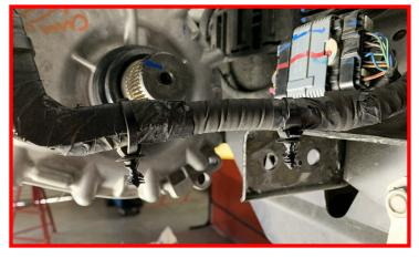
Using a suitable jack, support the transfer case.
