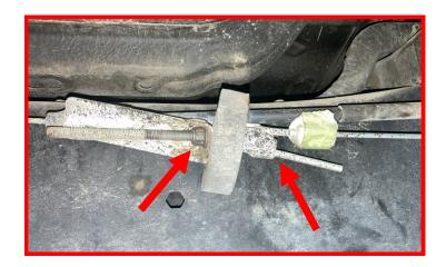
Remove the e-brake cable setup from the back of the rear driver side hub. You will need to unhook the cable hook attachment and also undo the clip that retains the cable housing itself.
