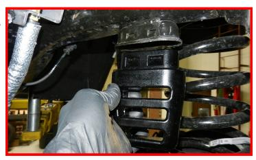
Using the supplied drill template, align the corresponding hole with the correct side. "D" will line up with the factory driver side hole and the "P" will line up with the passenger side hole.
