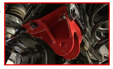
Install track bar using factory hardware.
