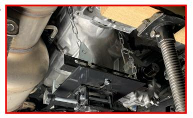
Remove the (8) transfer case mounting nuts.
