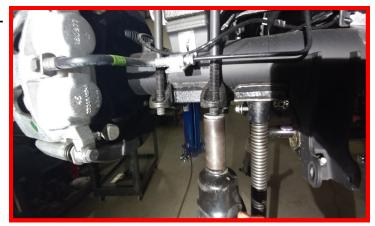
Lower the axle just enough to remove the factory block and install the ReadyLIFT block, making sure not to over extend brake and ABS lines. Adjust as necessary.
