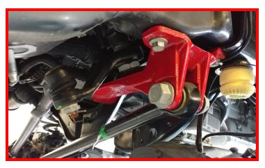
Install the ReadyLIFT sway bar drops to the frame using factory hardware.
