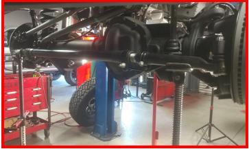
Remove the factory radius arm pivot hardware.
