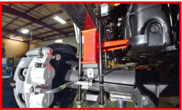
Install rear Falcon shock using factory hardware.
