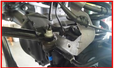
Support the axle with a suitable jack and remove the lower shock hardware from the axle mount.
