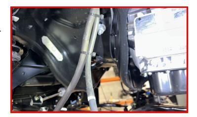
Install the brake line extensions into the factory bracket location using the factory bolt.
