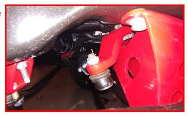
Install the factory isolator onto the provided lift springs, and then the springs onto the axle making sure to clock the dead end of the spring into the spring lock. Raise the axle enough to hold the springs into place.
