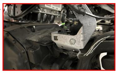
Remove the vacuum line clips from the driver side radius arm.
