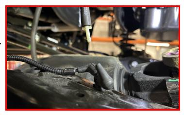
Install the supplied barbed coupler and vacuum line in between the factory line and the elbow.
