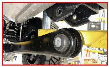
Insert the radius arm drop down brackets into the mounting pocket.
