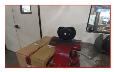
Using the supplied M8 locking nut and washer, Install bump stop mount to the ReadyLIFT extension making sure the cut edge faces to the inside of the vehicle.
