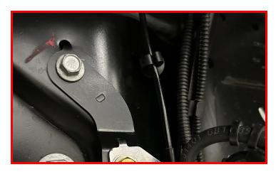
Gently pull down on the metal line until you can get the bracket to line up with the bottom two holes on the brake line drop.
