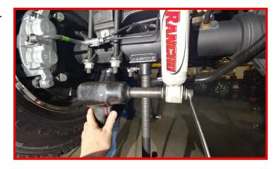
Loosen but do not remove the passenger side u-bolts. Remove the driver side u-bolts completely and lower the axle.
