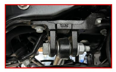
Remove the steering stabilizer from the frame.
