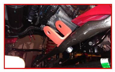
Install the steering stabilizer to the brackets using M12 x 70mm bolts, washers, and nuts. Mark the orientation of the brackets to the tie rod end and frame mount. Remove the stabilizer.
