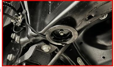
Remove the bump stop mount from the frame.
