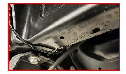
Install the ReadyLIFT bump stop extension to the frame by threading it into the existing bolt hole. Use a punch or similar tool in the holes of the mount and tighten. Install the bump stop mount to the extension using M8 nut and washer.
