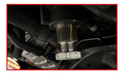
Install the drop pitman arm using the factory nut. Remove the nut, and clean off any lubricant from the sector shaft and pitman arm nut threads and apply a liberal amount of thread locker. Run tight. Use a chain or other suitable strap through the pitman arm tie rod mounting hole to the passenger side frame rail to keep gear box from turning.
