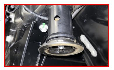
Install the factory bump stop into the cup in a factory orientation.
