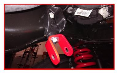
Install the ReadyLIFT steering stabilizer bracket to the tie rod using M12 x 55mm bolt, washers, cone adapter, and nut. Cone adapter will install from the bottom going up. Do not tighten at this time. The stabilizer must be test fit to establish the bracket's final orientation.
