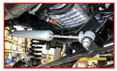
Reinstall the steering stabilizer and torque hardware to 45 ft-lbs.
