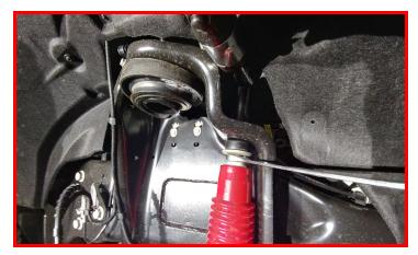
Install the ReadyLIFT track bar mount to the frame using factory hardware.
