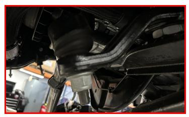
Remove the factory track bar bracket by removing the 2 vertical bolts and 3 horizontal nuts.
