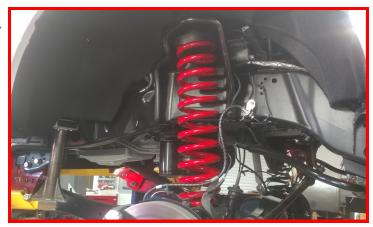
Install the Falcon Front Shock using the provided hardware on the top.
