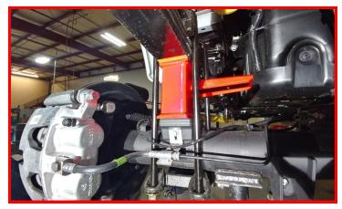
Install aftermarket rear shock using factory hardware. Do not tighten at this time.
