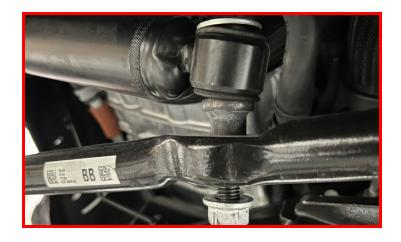
Remove the tie rod end at the pitman arm. Strike the pitman arm with a dead blow hammer to dislodge the taper.
