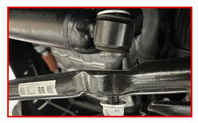
Remove the tie rod end at the pitman arm. Strike the pitman arm with a dead blow hammer to dislodge the taper.
