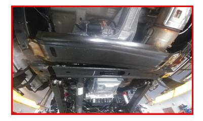
eave the axle hanging from the shocks. Place a suitable jack under the tie rod ends close to the knuckles.
