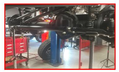
Remove the factory radius arm pivot hardware.
