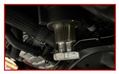
Install the drop pitman arm using the factory nut. Remove the nut, and clean off any lubricant from the sector shaft and pitman arm nut threads and apply a liberal amount of thread locker. Run tight. Use a chain or other suitable strap through the pitman arm tie rod mounting hole to the passenger side frame rail to keep gear box from turning.
