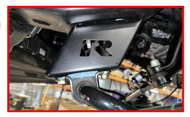
Install the front wheels. Lower the vehicle to the ground. Torque the lug nuts to the wheel manufacturers specs. Jounce the vehicle a few times to settle it to the new ride height. Install the front drive shaft using the factory hardware with a drop of thread locker. Torque to 26 ft-lbs, the lower shock hardware to 65 ft-lbs, the radius arm hardware to 200 ft-lbs, track bar at the bracket to 350 ft-lbs.
