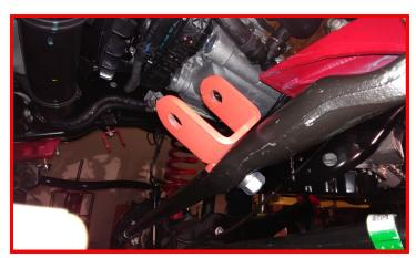
Install the steering stabilizer to the brackets using M12 x 70mm bolts, washers, and nuts. Mark the orientation of the brackets to the tie rod end and frame mount. Remove the stabilizer.
