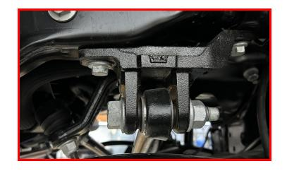
Remove the steering stabilizer from the frame.
