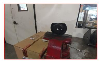
Using the supplied M8 locking nut and washer, Install bump stop mount to the ReadyLIFT extension making sure the cut edge faces to the inside of the vehicle.
