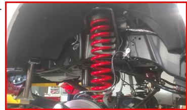
Install the Falcon Front Shock using the provided hardware on the top.
