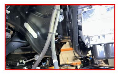
Install the brake line extensions into the factory bracket location using the factory bolt.
