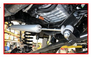
Reinstall the steering stabilizer and torque hardware to 45 ft-lbs.
