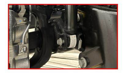
Lower the axle enough to remove the front springs. Remove the shock from the frame.
