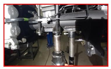
Install the ReadyLIFT driver side block (D is cut into the block under the bump stop tang) and raise the axle lining the center pins up. Install using the provided u-bolts and nuts but do not fully tighten at this time. Repeat steps for the passenger side. (P is cut into the block under the bump stop tang)
