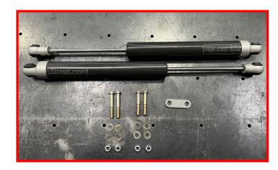
Using the M12 x 75mm bolts, washers and nuts, install the body end of the stabilizers onto the center stabilizer bracket. Stabilizer body end should be installed with the stabilizer top plate on top and the center stabilizer bracket on bottom (as shown in photo). Do not tighten at this time.
