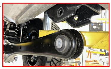
Remove the (2) radius arm axle mounting bolts.
