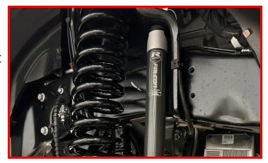
Using the factory hardware on the bottom, install into the lower shock perch.
