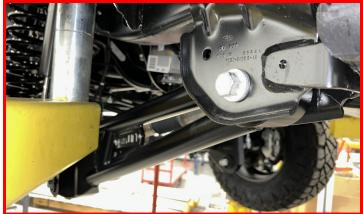
At this time, align the cam bolts as described below and torque to 200 ft-lbs. It is recommended to check alignment and make adjustments to cams before applying final torque.
