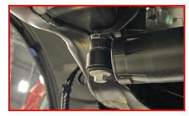
Remove the steering stabilizer nut from the tie rod. Use an air hammer or other suitable device to dislodge the taper.
