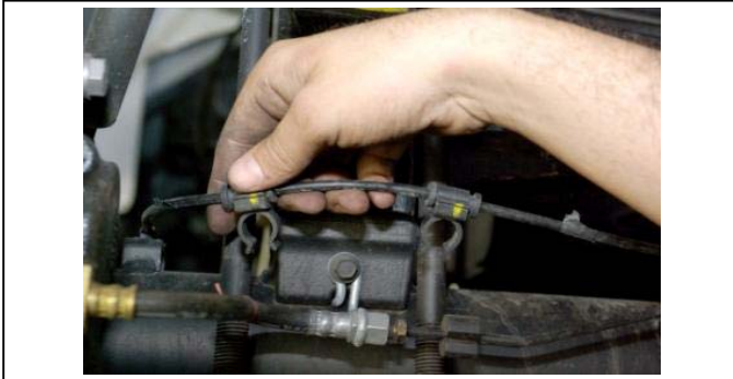
73. Disconnect the ABS line clips from the dr/pass side u-bolts.
