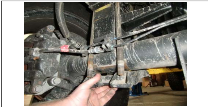
76. Remove the u-bolts and lower the axle plate.
