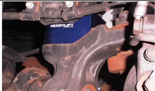
40. Install the spacer in between the axle and the spring perch plate. Use the provided longer hardware when installing. Torque.
