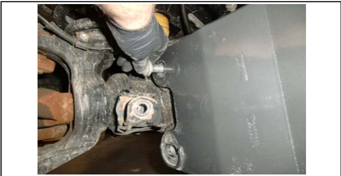
24. Stage 2: Install the new assembled radius arm with the OE bolt on top.
