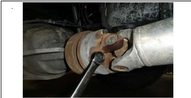
97. Install the driveshaft spacer with new provided hardware, torque.
