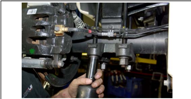
75. Loosen and remove the OE u-bolts from the axle.
