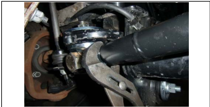
68. Tighten the jam nut at the axle mount.
