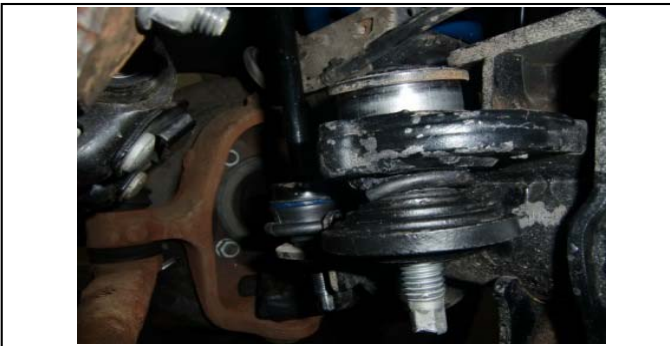
55. Remove the ball joint from the axle.
