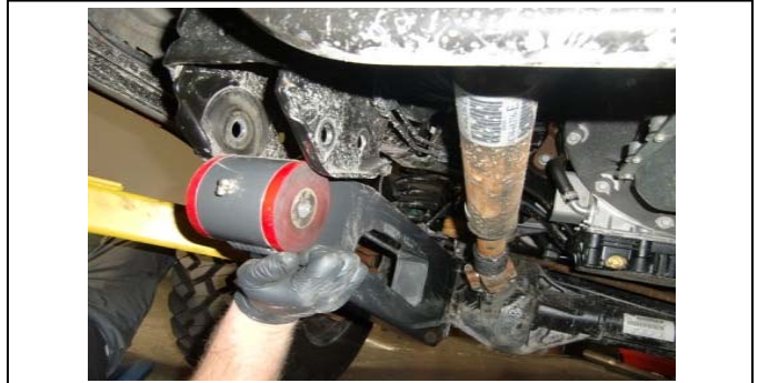
26. Stage 2: Install the radius arm into frame pocket using OE hardware.
