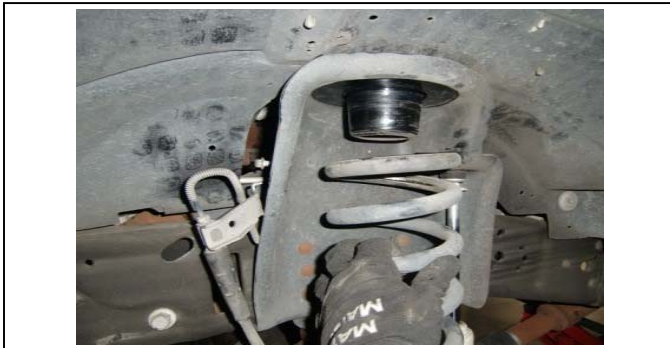
27. Raise the vehicle enough to remove the factory springs.
