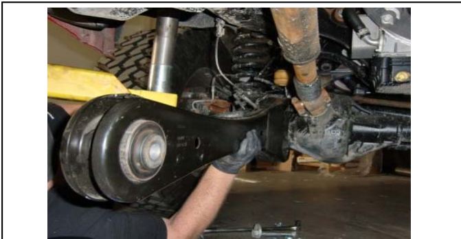
23. Stage 2: Remove the axle side radius arm hardware, then the arm.
