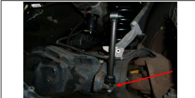
44. Install the new end link into the lower axle tab with new hardware.
