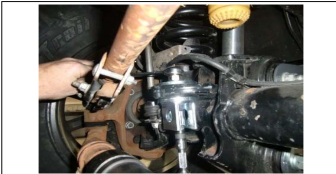
61. Tighten the hardware to spec once the clevis is fully seated.
