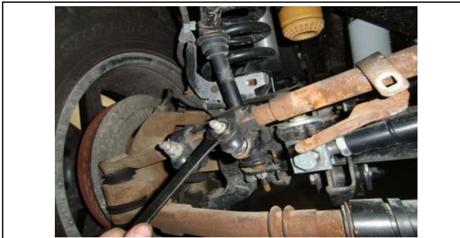
101. 3) Loosen the (2) collar bolts and lube the threads of steering linkage.
