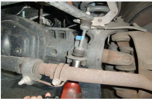
11. Disconnect and remove the factory sway bar end links.
