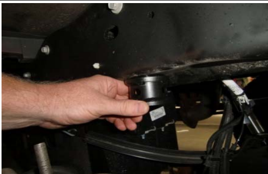
93. Install the rear bump stop extension into the OE location.
