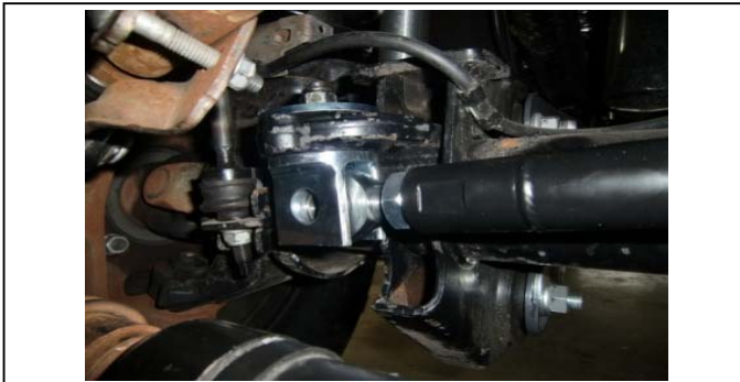
62. Insert the track bar into the clevis, check the clearance.
