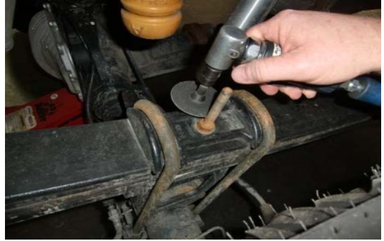
90. Cut off the excess centering pin threads on pass. side leaf pack.
