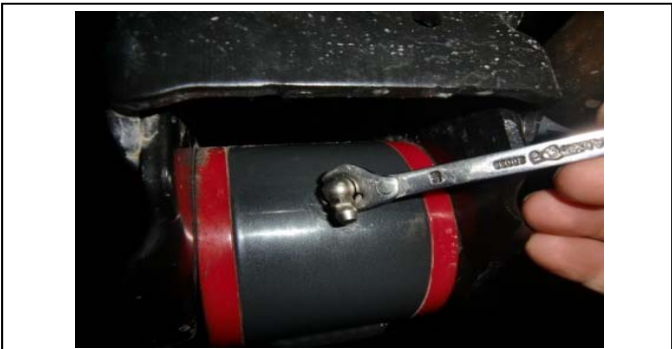
22. Stage 2: Install the provided zerk fittings.
