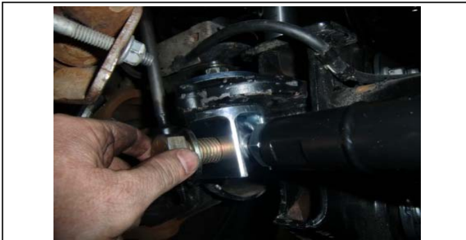
63. Attach with provided hardware, do not tighten until adjusted.
