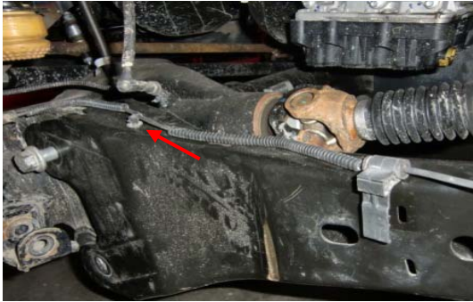
9. Remove all of the wiring clips from the radius arms.
