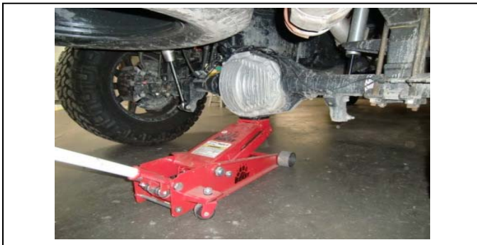
71. Rear Install: Lift the rear of the vehicle by frame and support the axle.
