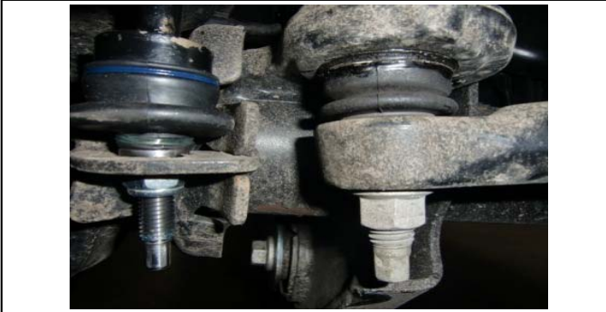
49. Stage 3: (Steps 49-69) View of track bar ball joint at axle mount.
