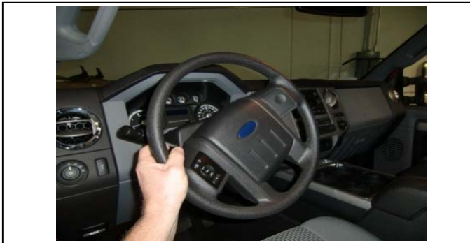
99. Straighten steering wheel steps: 1) Unlock the steering wheel.
