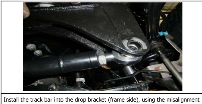
62. Insert the track bar into the clevis, check the clearance.
