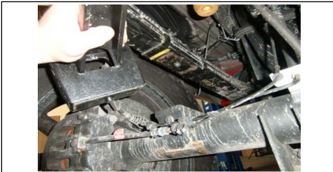
77. Lower the axle and remove the factory lift block.
