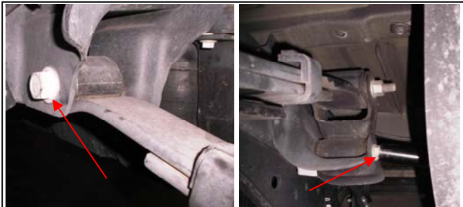
79. Unbolt the leaf spring from the truck at front and rear of the spring. Leave the shackle attached to the leaf spring until the spring has been removed from the truck.
