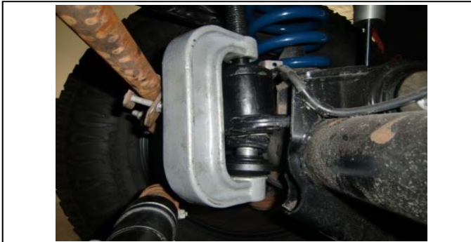
54. View of the tool positioned to remove the ball joint.
