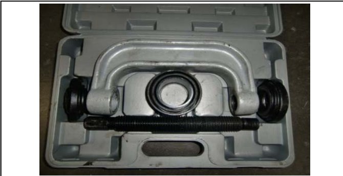
53. Use the proper heavy duty ball joint removal tool set.
