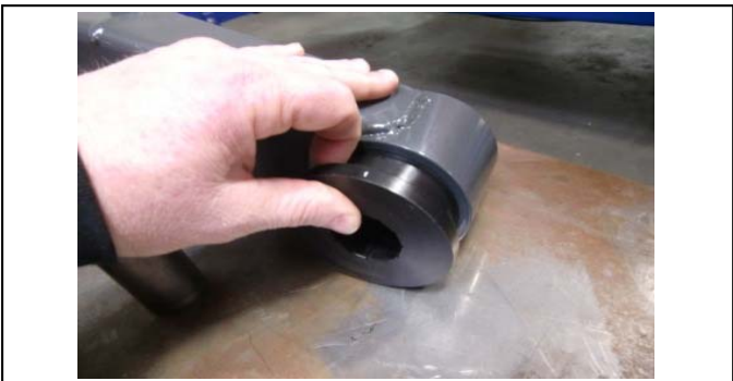
20. Stage 2: Install the bushings into the arms.
