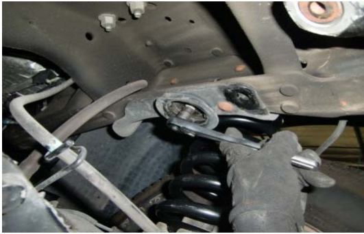
35. Unbolt the bump stop cup mount from the frame.
