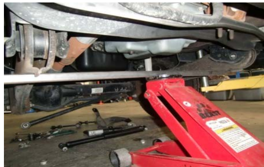
14. Support the axle. Use a floor jack & crossbar to support the radius arms.
