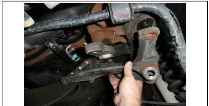
30. Remove the OE track bar bracket from the cross member and frame.
