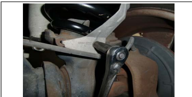
48. Re-attach the brake line hose/bracket to the lower spring perch.
