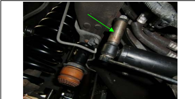
43. Install the steering stabilizer drop boss with the provided hardware.
