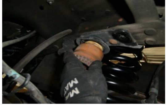
34. Remove the front bump stops from the frame.
