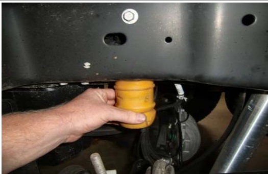
91. Remove the rear bump stops from the frame.
