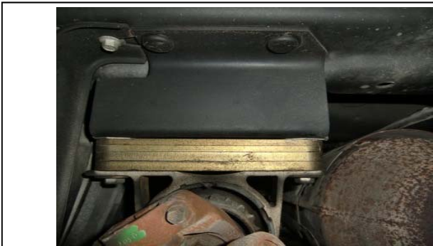
98. Vehicles with 2pc drive shafts may require drop carrier shims.
