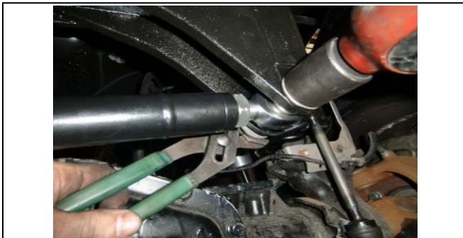
67. Tighten the other end at the frame mount to OE spec.
