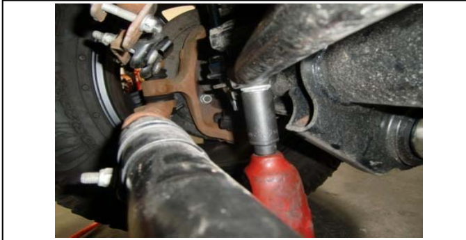
50. Loosen the ball joint nut and leave it attached.
