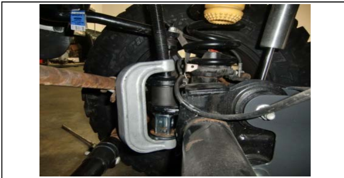
60. Use the press tool to draw clevis into position.
