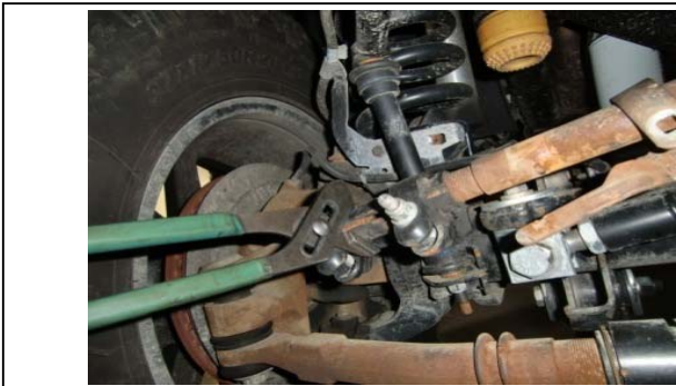
102. 4) Adjust the collar to straighten the steering wheel.
