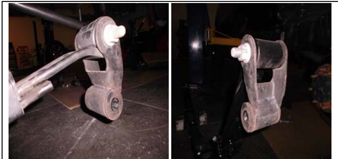
80. Unbolt the shackle from the factory leaf pack and install onto the new leaf pack. Note: the shackle mounting direction.
