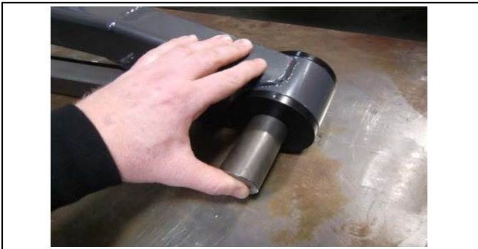
21. Stage 2: Use grease provided, lube pivot pin then install into bushings.
