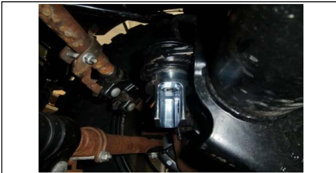
58. Align the clevis so it lines up with the track bar frame mount bracket.
