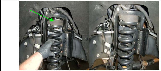
41. Re-use the OE spring isolator. Lift the vehicle enough to install the new coil springs, then lower to allow the spring to settle under the weight. Install longer front shocks after springs have been installed.
