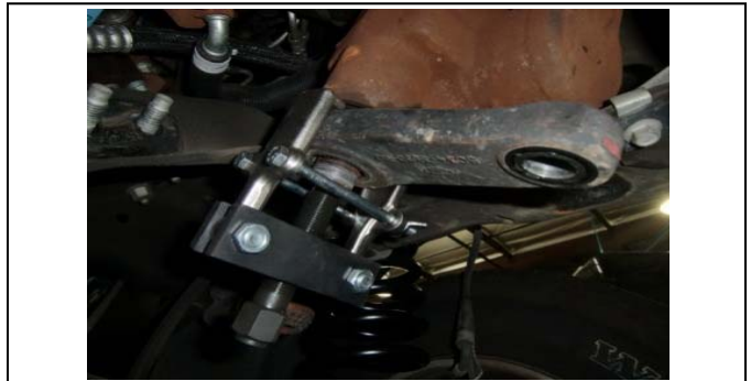
32. Use the proper pitman arm puller to remove from the steering box.
