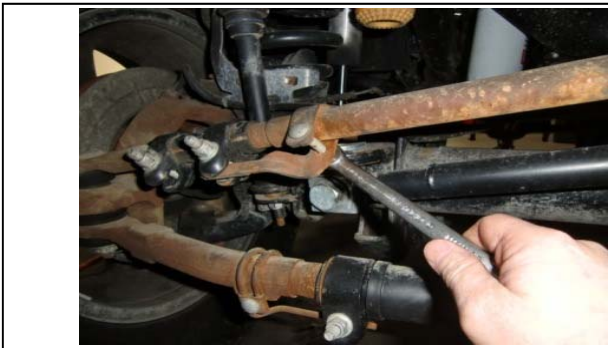
100. 2) Remove the safety keeper bolt and slide the bracket out of collar.
