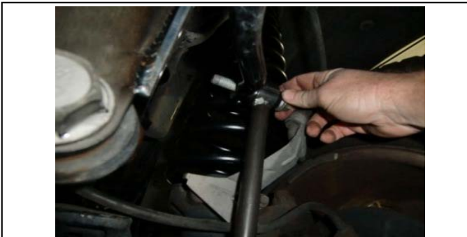
45. Attach the top sway bar end link to the sway bar.
