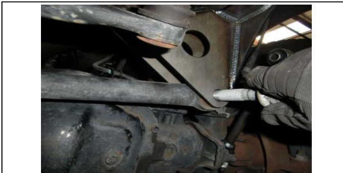
46. Reconnect the track bar to the drop bracket. Use OE hardware, torque.
