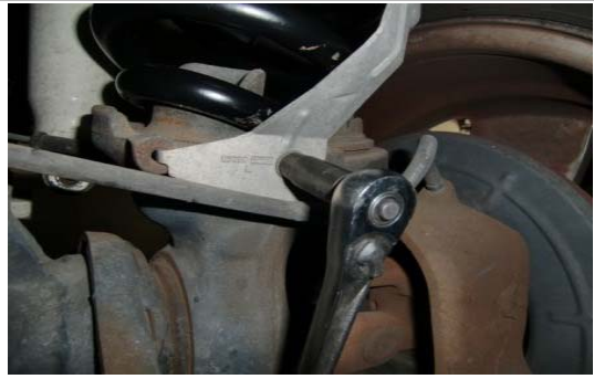
12. Disconnect the brake line bracket from the lower spring perch.
