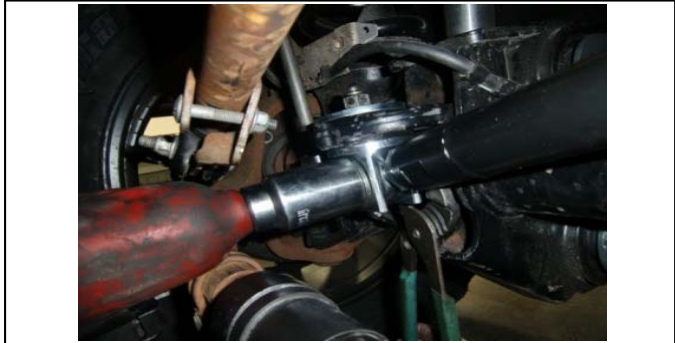
66. Once the track bar is adjusted, tighten to spec.
