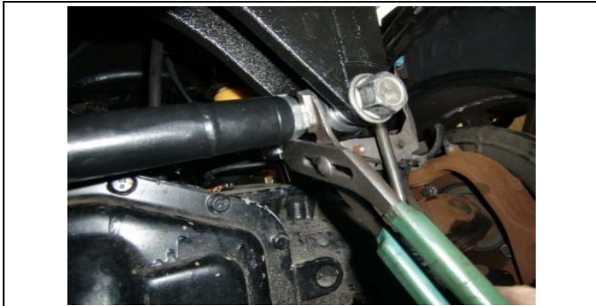
69. Tighten the jam nut at the frame mount.
