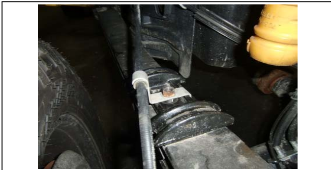
78. Drivers side: remove the e-brake bracket from upper u-bolt plate.
