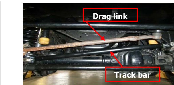
104. Reinstall the wheels and tires. Lower the vehicle to the ground and adjust the track bar if needed. Double check all work performed and the brakes must be bled before use of vehicle.
