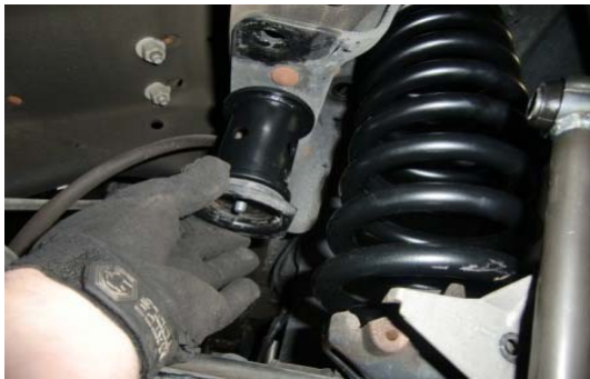
37. Reinstall and align the OE bump stop cups onto the drop bracket.
