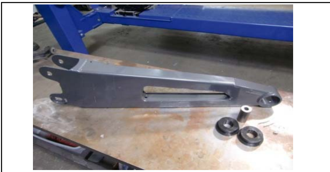
19. Stage 2: Gather the radius arms and bushing kit for assembly.
