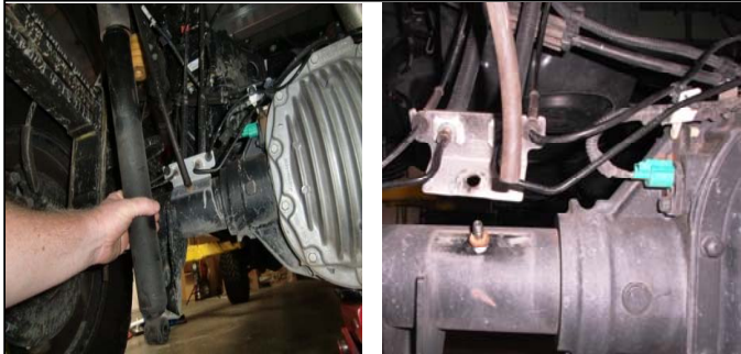
74. Unbolt and remove the rear shocks. Note: longer shocks required. Disconnect the rear brake line bracket/ vent line from the axle.
