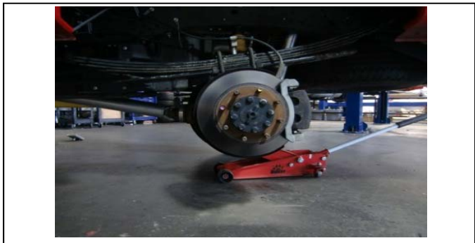
72. Remove the rear wheels from the vehicle.
