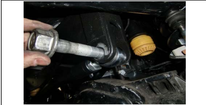
65. Attach the track bar with the original hardware.
