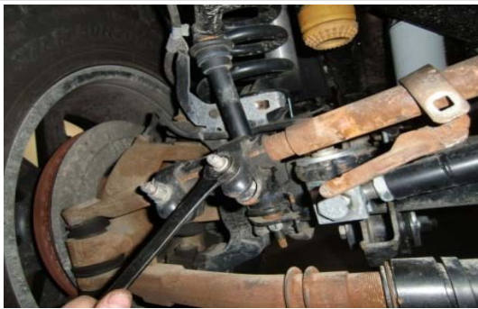
101. 3) Loosen the (2) collar bolts and lube the threads of steering linkage.
