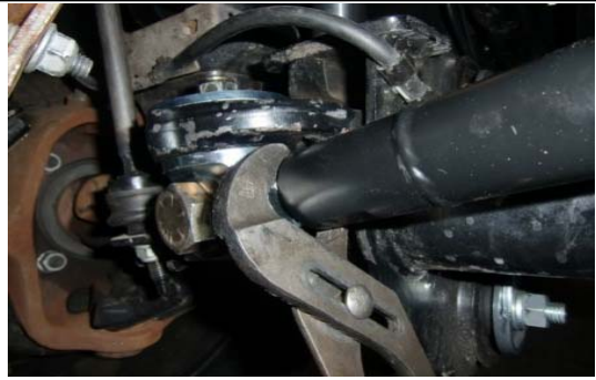
68. Tighten the jam nut at the axle mount.
