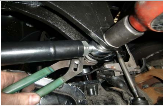
67. Tighten the other end at the frame mount to OE spec.
