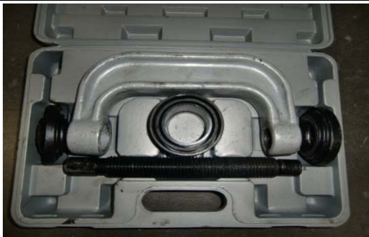
53. Use the proper heavy duty ball joint removal tool set.
