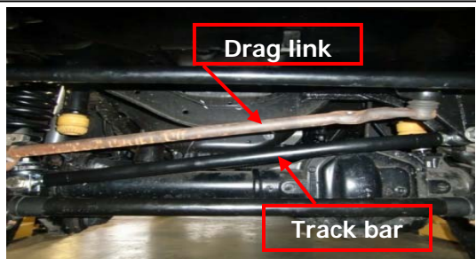
104. Reinstall the wheels and tires. Lower the vehicle to the ground and adjust the track bar if needed. Double check all work performed and the brakes must be bled before use of vehicle.
