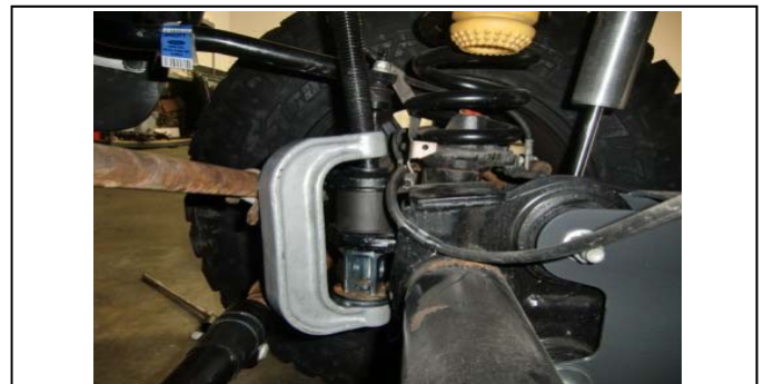
60. Use the press tool to draw clevis into position.
