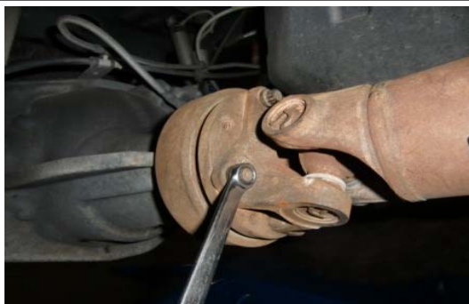
95. Vehicles w/1pc drive shaft: Remove the (4) bolts at the differential.
