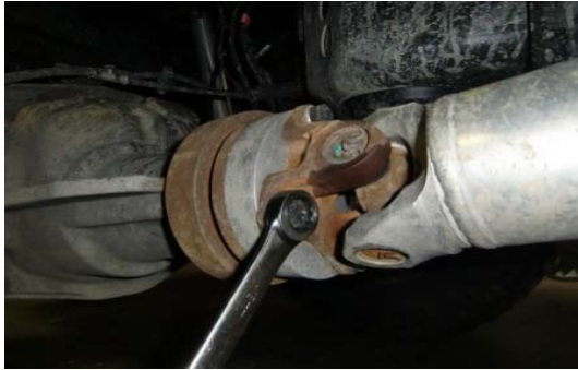
97. Install the driveshaft spacer with new provided hardware, torque.
