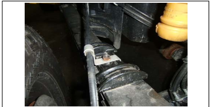
78. Drivers side: remove the e-brake bracket from upper u-bolt plate.
