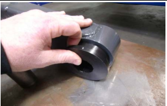
20. Stage 2: Install the bushings into the arms.
