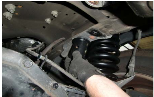
36. Screw the bump stop drop bracket into the OE frame location.
