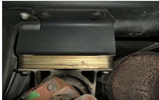
98. Vehicles with 2pc drive shafts may require drop carrier shims.
