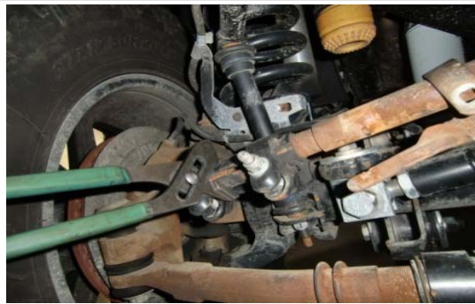
102. 4) Adjust the collar to straighten the steering wheel.
