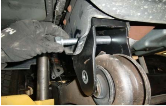
17. Stage 1: Install new radius arm drop brackets.
