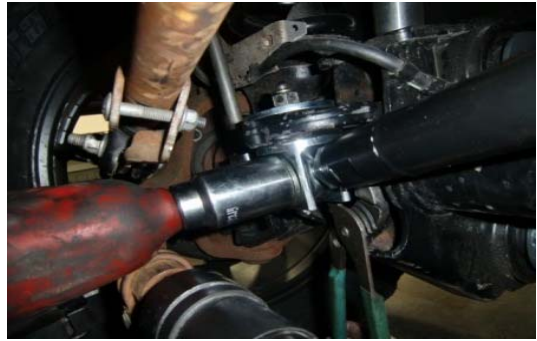
66. Once the track bar is adjusted, tighten to spec.
