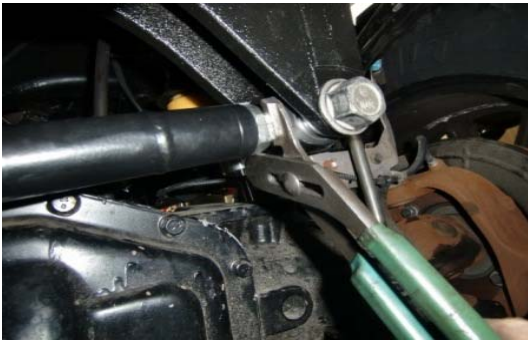
69. Tighten the jam nut at the frame mount.
