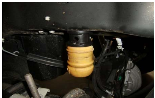
94. Reinstall the OE bump stop into the drop bracket.
