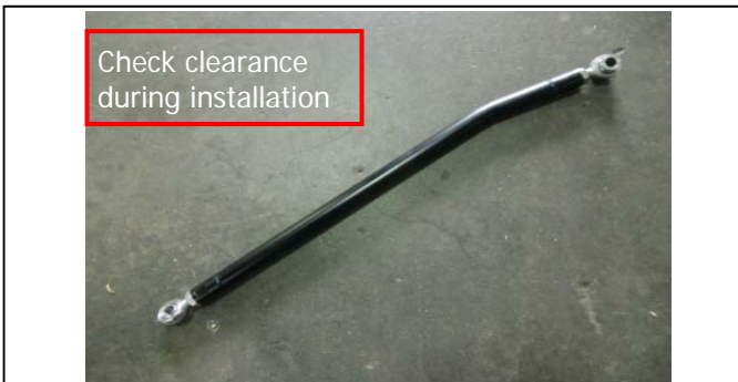
59. Use the assembled track bar as a guide to ensure proper position.
