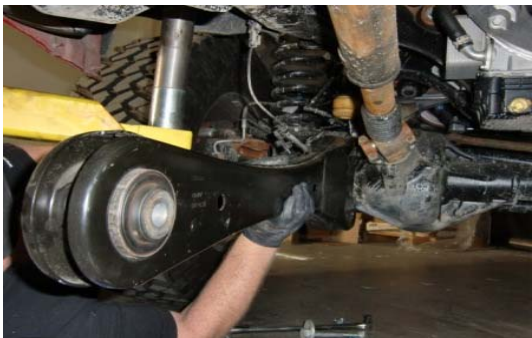
23. Stage 2: Remove the axle side radius arm hardware, then the arm.
