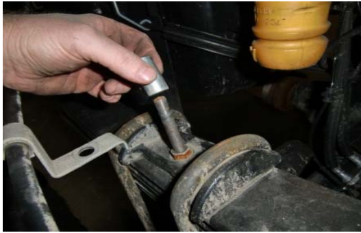
89. Install the spacer and OE bracket over drivers side centering pin. Torque
