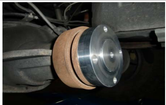
96. Clean off the mounting surface and ensure that the spacer fits flush.
