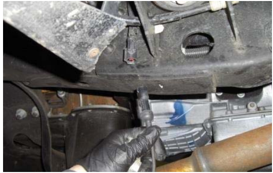
10. Disconnect the ABS line plug above the radius arms.
