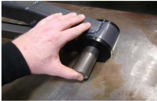
21. Stage 2: Use grease provided, lube pivot pin then install into bushings.
