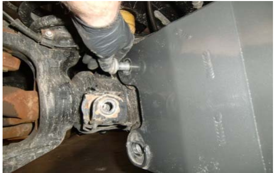
24. Stage 2: Install the new assembled radius arm with the OE bolt on top.
