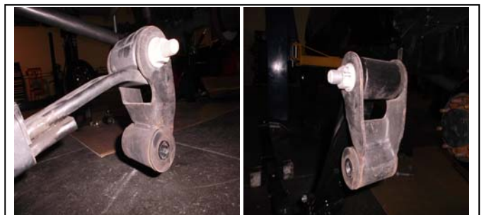
80. Unbolt the shackle from the factory leaf pack and install onto the new leaf pack. Note: the shackle mounting direction.
