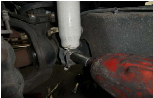
13. Remove the front factory shocks. Note: Longer shocks required.
