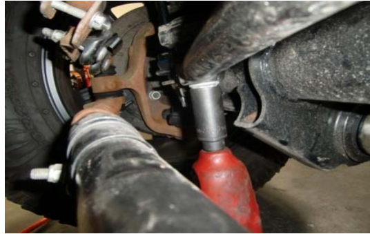
50. Loosen the ball joint nut and leave it attached.
