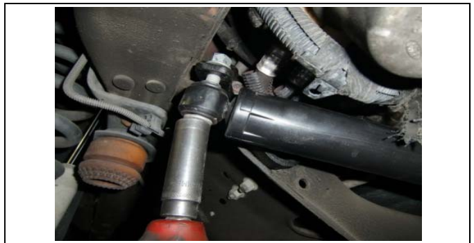
28. Disconnect the steering stabilizer from the frame.
