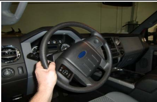
99. Straighten steering wheel steps: 1) Unlock the steering wheel.
