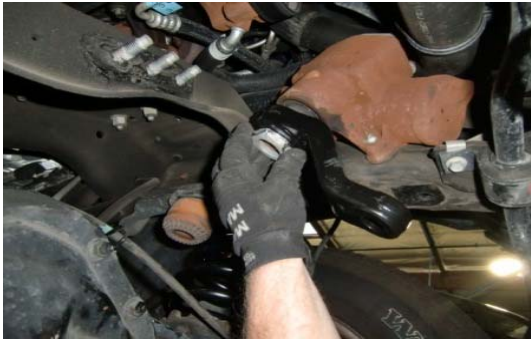
33. Install the new drop pitman arm with OE nut and torque to spec.
