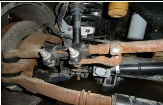
103. 5) Tighten up the hardware and replace the keeper bolt.
