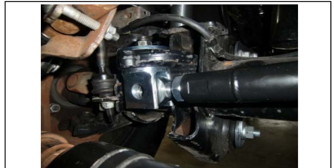
62. Insert the track bar into the clevis, check the clearance.
