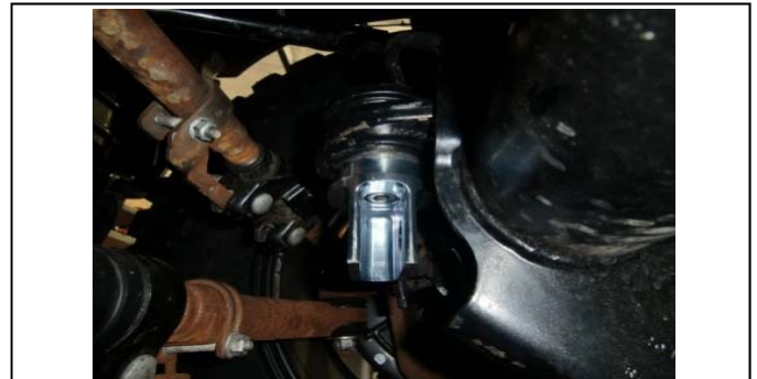
58. Align the clevis so it lines up with the track bar frame mount bracket.
