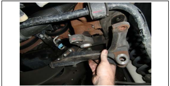
30. Remove the OE track bar bracket from the cross member and frame.
