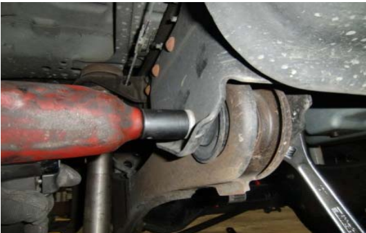
15. Unbolt both of the radius arms at the frame.
