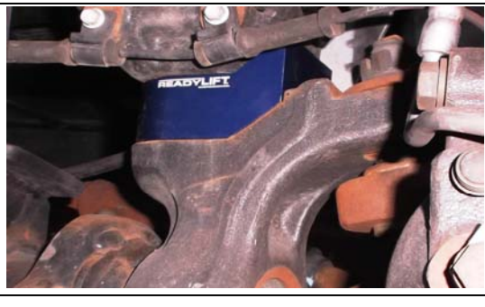
40. Install the spacer in between the axle and the spring perch plate. Use the provided longer hardware when installing. Torque.
