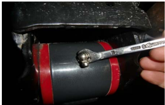
22. Stage 2: Install the provided zerk fittings.
