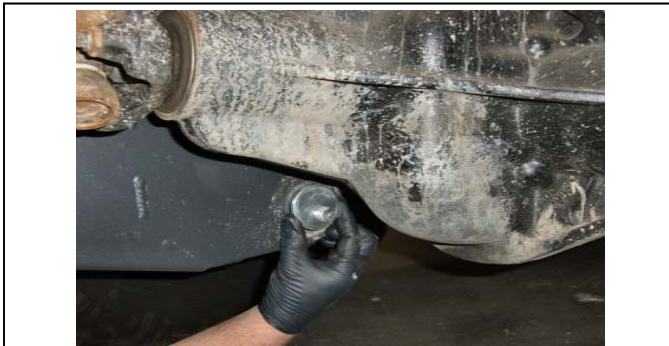
25. Stage 2: Install the new offset cam bolts into the lower mount.
