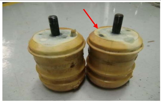
92. Note: The locating tab must be trimmed from the bump stop.
