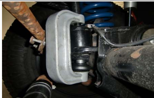
54. View of the tool positioned to remove the ball joint.
