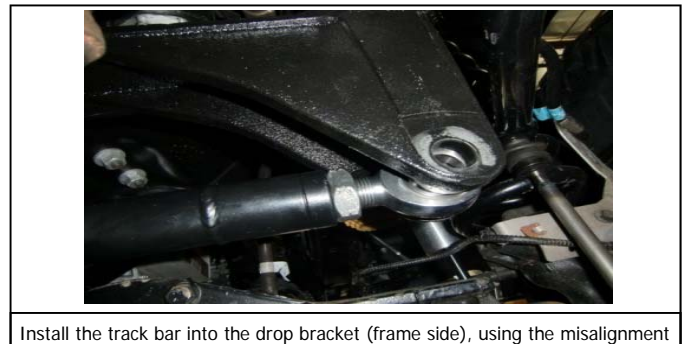
62. Insert the track bar into the clevis, check the clearance.
