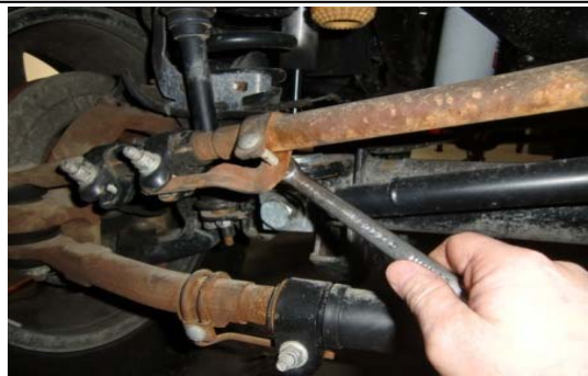
100. 2) Remove the safety keeper bolt and slide the bracket out of collar.
