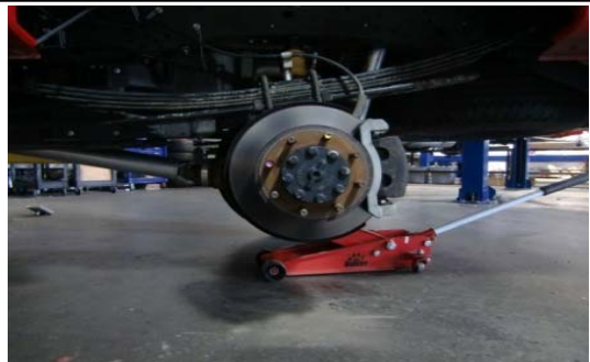
72. Remove the rear wheels from the vehicle.
