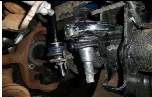
52. View of the ball joint to be removed.
