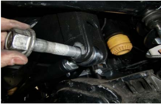
65. Attach the track bar with the original hardware.
