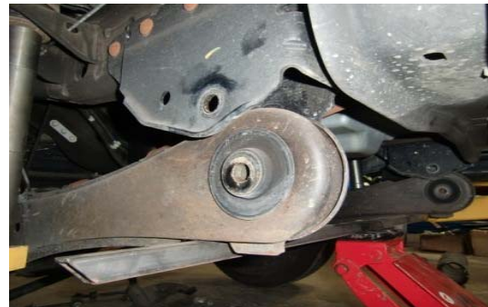
16. Lower the radius arms enough to install the drop brackets.
