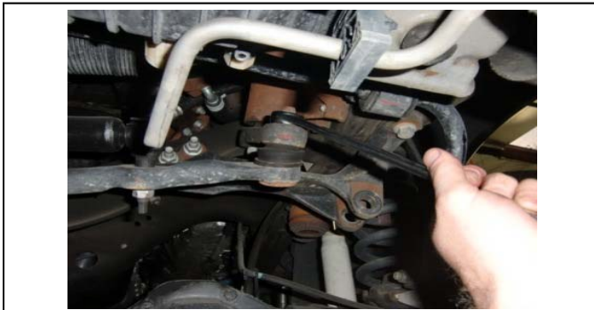
29. Remove the cotter pin and disconnect the drag link from pitman arm.
