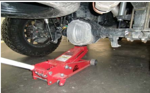
71. Rear Install: Lift the rear of the vehicle by frame and support the axle.
