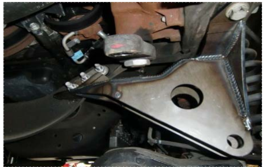
38. Install the new track bar drop bracket with OE hardware.
