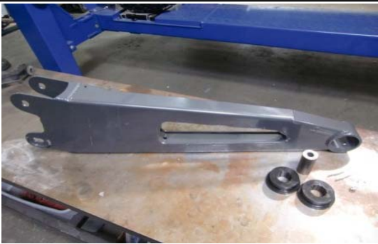
19. Stage 2: Gather the radius arms and bushing kit for assembly.
