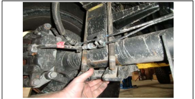
76. Remove the u-bolts and lower the axle plate.
