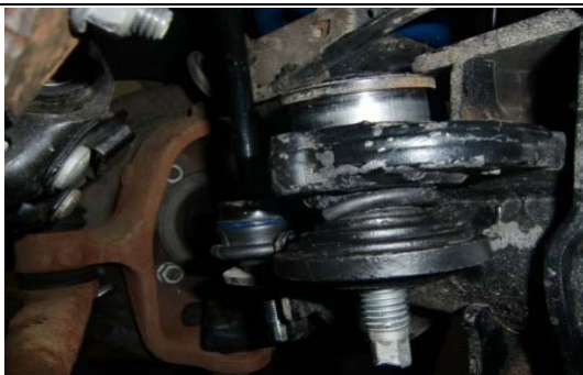
55. Remove the ball joint from the axle.
