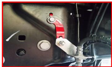
Reattach the factory brake line bracket at the axle using factory hardware. Torque to 5 ft-lbs.
