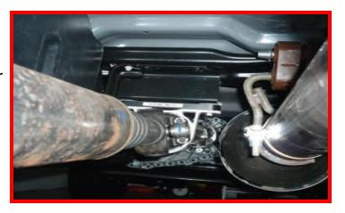
Prior to installing wheels, complete all installation steps on the opposite side. Install the wheels and lower the vehicle to the ground. Torque the lug nuts to the wheel manufacturers specs. Jounce the vehicle to settle the suspension to the new ride height. Torque the radius arm hardware to 200 ft-lbs, track bar to track bar bracket hardware to 250 ft-lbs, u-bolts to 110 ft-lbs and all shock hardware to 65 ft-lbs.
