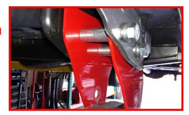
Rotate the axle until you can line up the radius arms into the ReadyLIFT drop brackets. Install using factory hardware. Tighten Radius arm drop to frame hardware to 200 ft-lbs. DO NOT TIGHTEN RADIUS ARM PIVOT BOLT AT THIS TIME.
