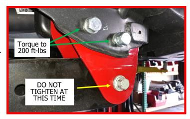
Install the track bar into the track bar bracket using factory hardware. Do not tighten at this time.
