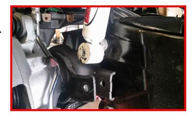
Remove the upper shock hardware from the frame and remove shock from the vehicle. Properly discard the shock.
