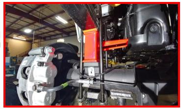
Install rear Falcon shock using factory hardware. Do not tighten at this time.
