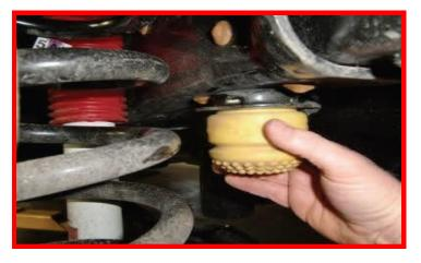
Install the ReadyLIFT bump stop spacer and factory bump stop mount to the frame using M8 x 70 mm bolt and washer. Torque to 5 ft-lbs. Install the bump stop to the factory mount by pressing it back into place.
