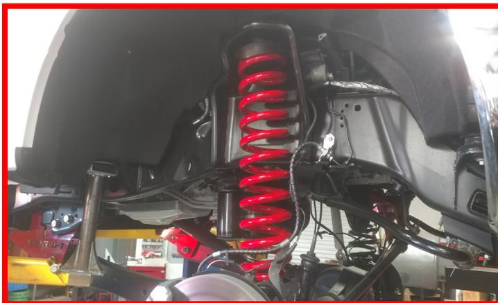
Install the **Falcon front shock** using the provided hardware on the top and the factory hardware on the bottom attachment.
