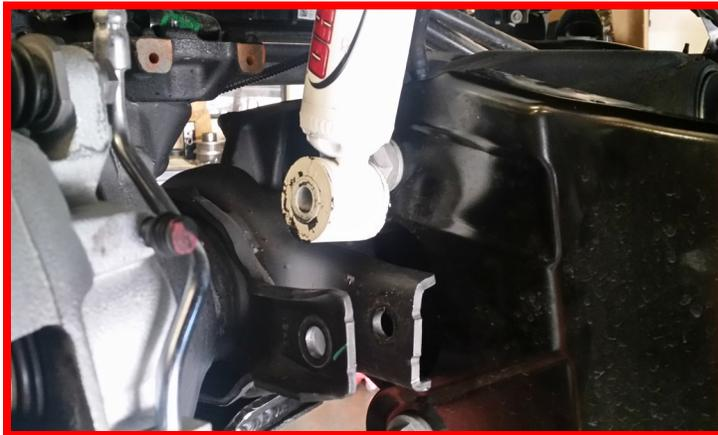
Remove the **upper shock hardware** from the frame and remove shock from the vehicle.
