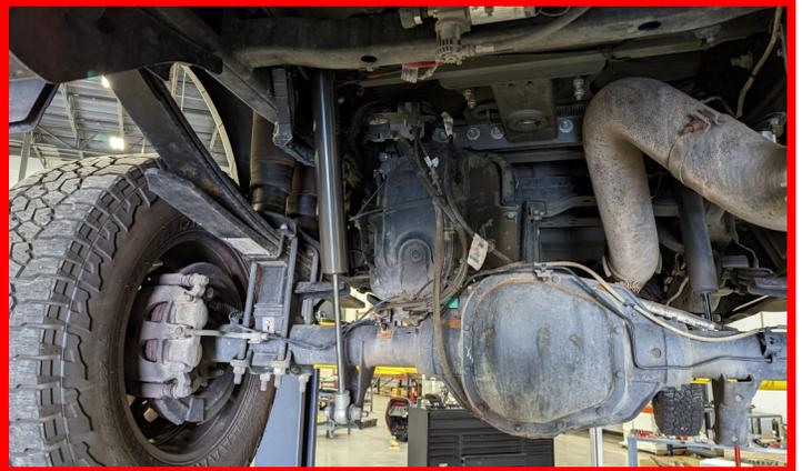
If equipped with a 2 piece driveline, remove the bolts holding the carrier bearing to the frame. Install the ReadyLIFT carrier bearing spacer between the carrier bearing and frame using **7/16" bolts, washers and nuts**.
