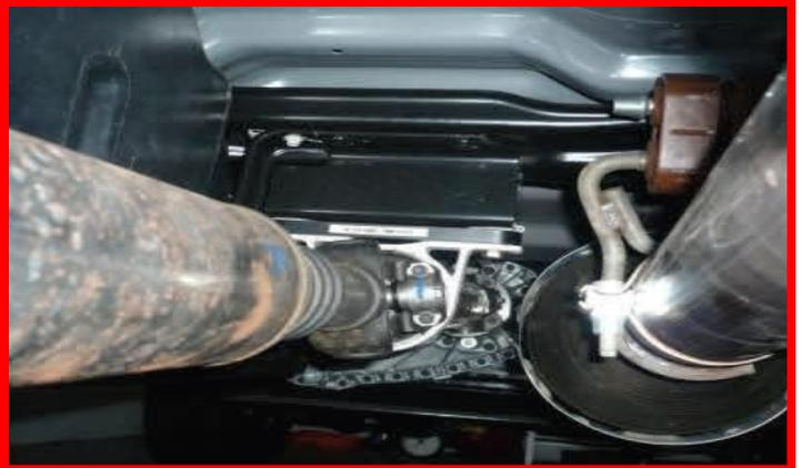
Prior to installing wheels, complete all installation steps on the opposite side. Install the wheels and lower the vehicle to the ground. Torque the lug nuts to the wheel manufacturers specs. Jounce the vehicle to settle the suspension to the new ride height. Torque track bar to track bar bracket hardware to **450 ft-lbs**, u-bolts to **110 ft-lbs** and all shock hardware to **65 ft-lbs**.
