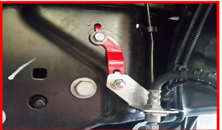
Reattach the factory brake line bracket at the axle using **factory hardware**.
