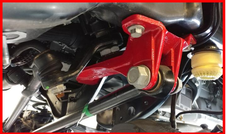
Install the ReadyLIFT sway bar drops to the frame using factory hardware.
