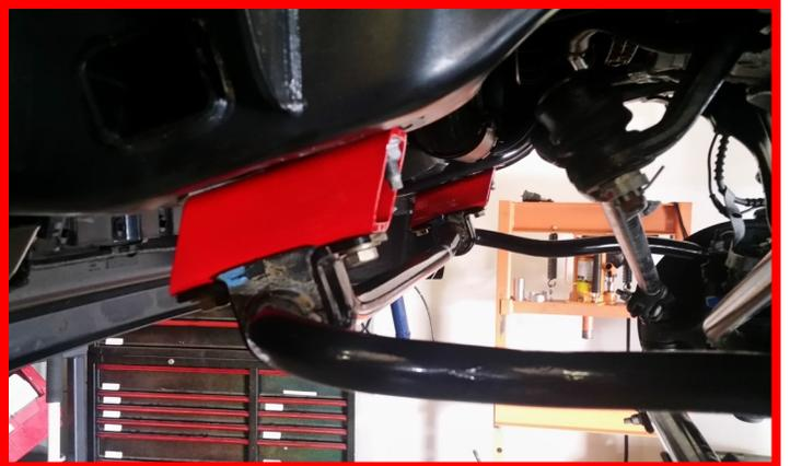
Install the ReadyLIFT brake line bracket to the factory brake line using **5/16" x 3/4" bolts, washers, and nuts**. Install the bolt facing outwards.
