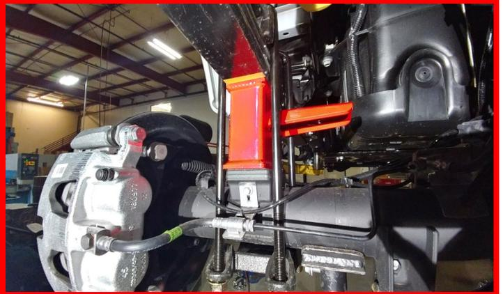
Install **rear Falcon shock** using factory hardware.
