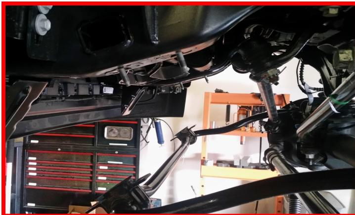
Remove track bar from the track bar bracket. Let the track bar hang out of the way.
