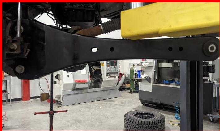
Install **ReadyLIFT radius arms** into axle using factory hardware for the upper bolt and provided cam bolt for the lower.
