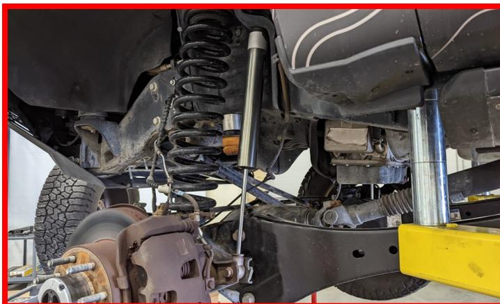
Remove the jack stands from under the axle and let the axle hang. Place those jack stands under the tie rods as shown in the image.
