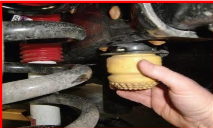
Install the ReadyLIFT bump stop spacer and factory bump stop mount to the frame using **M8 x 70 mm bolt and washer**.
