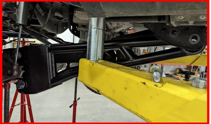
Install the track bar into the track bar bracket using factory hardware.
