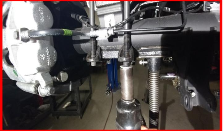
Lower the axle just enough to remove the **factory block**, making sure not to over extend brake and ABS lines. Adjust as necessary.
