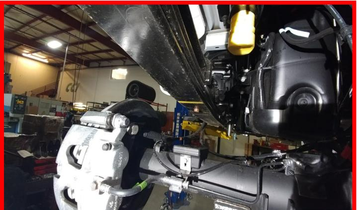
Locate the **driver side lift block** (Has a D cut into it under the bump stop tang). Raise the axle and the block up to the spring while aligning the center pin. Install the **provided u-bolts, and nuts**. Snug the u-bolt nuts but **do not fully tighten at this time**. Repeat steps for passenger side.
