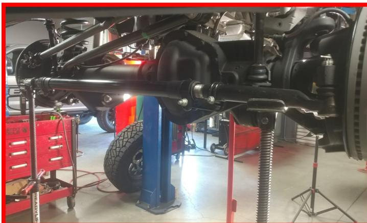
Unbolt the radius arm from the pivot point on the frame and raise the jackstands so the radius arm swings out of the way of the frame mount.
