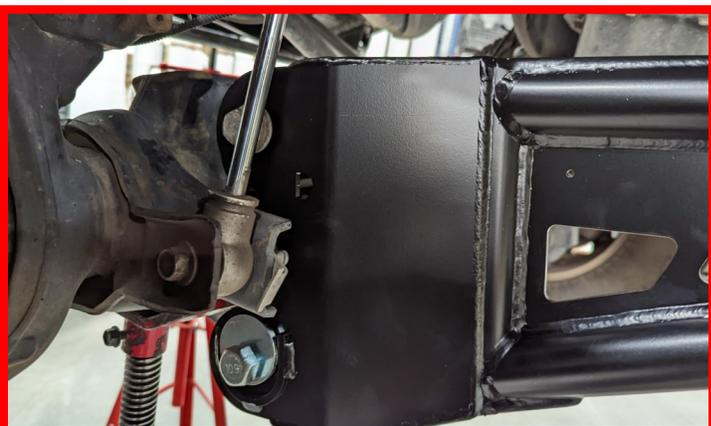
Rotate the axle until you can line up the ReadyLIFT radius arms with the factory hole. Install using **factory hardware**.
