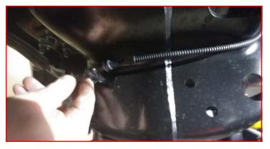
Mark the drive shaft to pinion orientation, then remove the drive shaft from the front differential. Tape the u joint caps to keep them from falling off / damage while working.
