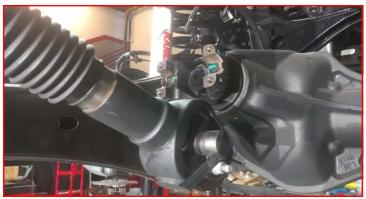
Remove the transfer case skid plate.
