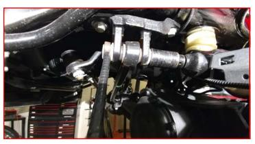
Remove the shock from the axle.
