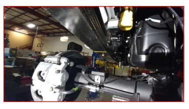
Install the ReadyLIFT driver side block (D is cut into the block under the bump stop tang) and raise the axle lining the center pins up. Install using the provided u-bolts and nuts but do not fully tighten at this time. Repeat steps for the passenger side. (P is cut into the block under the bump stop tang)
