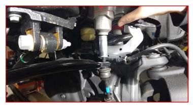
Remove the sway bar from the frame. Note orientation of the bar for re-installation.
