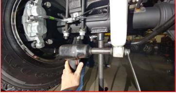
Loosen but do not remove the passenger side u-bolts. Remove the driver side u-bolts completely.
