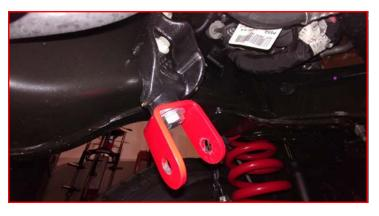
Install the ReadyLIFT steering stabilizer bracket to the tie rod using M12 x 55mm bolt, washers, cone adapter, and nut. Cone adapter will install from the bottom going up. Do not tighten at this time until the stabilizer has been test fit as to establish the brackets correct orientation.
