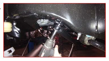
Remove the steering stabilizer nut from the tie rod. Use an air hammer or other suitable device to dislodge the taper.
