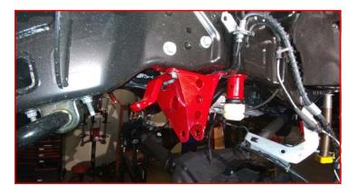
Install the track bar into the ReadyLIFT track bar mount using the factory hardware. Do not tighten at this time.
