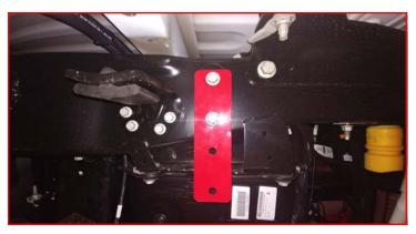
Install the factory sway bar bracket to the ReadyLIFT drop bracket using M12 x 35mm bolts, washers, and nuts. Torque to 45 ft-lbs.
