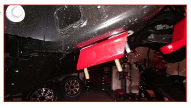
Install the factory sway bar to the ReadyLIFT brackets using 7/16" x 1.5" bolts, washers, and nuts. Torque to 55 ft-lbs.
