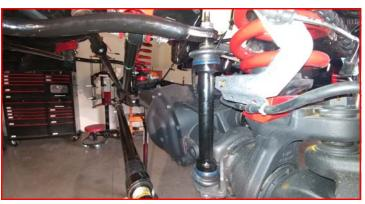
Loosen the tie rod adjuster and flip the tie rod 180 degrees and install to the ReadyLIFT pitman arm using factory hardware. Torque to 70 ft-lbs. Install the safety keeper and cotter pin.
