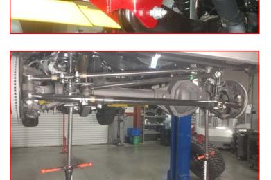
Remove the sway bar end links from the sway bar and axle.
