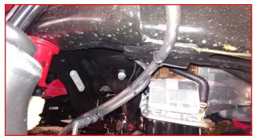
Install the ReadyLIFT brake line extensions to the factory brackets using 5/6" x 3/4" bolts, washers, and nuts. Install bolts from the frame side out.
