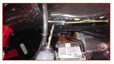
Zip tie the driver side vacuum line to the vent tube making sure that it can not be pinched by the bump stop when the suspension cycles.
