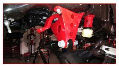
Install the factory isolator onto the ReadyLIFT springs, and then the springs onto the axle making sure to clock the dead end of the spring into the spring lock. Raise the axle enough to hold the springs into place. Install the front extended length shock to the frame using provided hardware and to the axle using factory hardware. Do not tighten at this time.
