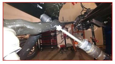
Remove the factory bump stop by grabbing and pulling it out of its mount using a twisting/ pulling motion.
