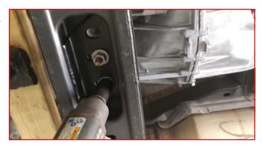
8" lift kit step only: Install the ReadyLIFT cross member using the factory bolts to hold cross member in place. Lower the transmission mount into the cross member and remove jack and wooden block. Install the transmission mount hardware. Do not tighten at this time. Support the cross member with the jack and remove one side cross member bolts. Install the wiring harness clip into the cross member.
