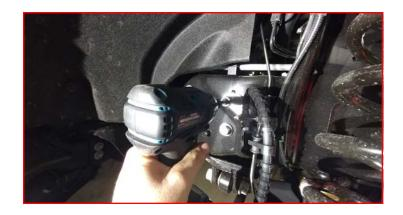
Remove the brake line bracket at the axle.
