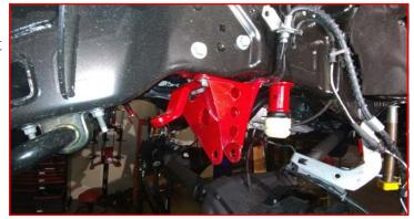
Install the track bar into the ReadyLIFT track bar mount using the factory hardware and the ReadyLIFT offset square washers. If installing the 6.5" lift, make sure the offset is closest to the driver side, and if installing the 8" lift the offset is closet to the passenger side. Do not tighten at this time. (8" lift orientation shown)
