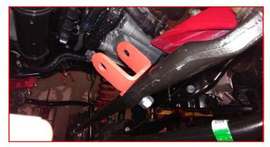
Install the steering stabilizer to the brackets using M12 x 70mm bolts, washers, and nuts. Mark the orientation of the brackets to the tie rod end and frame mount. Remove the stabilizer. Torque the mount hardware to 45 ft-lbs. Reinstall the steering stabilizer and torque hardware to 45 ft-lbs.
