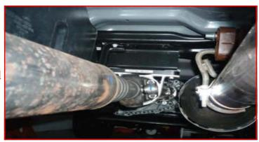
Install the extended length rear shocks using factory hardware. Make sure to install in the proper orientation for the shock that you have (inverted or standard mount). Do not tighten at this time. Install the wheels and lower the vehicle to the ground.
