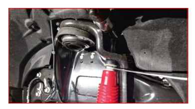
Remove the tie rod end at the pitman arm. Strike the pitman arm with a dead blow hammer to dislodge the taper.
