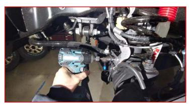
Remove the vacuum line clips from the driver side radius arm.
