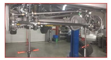
Remove the sway bar end links from the sway bar and axle.
