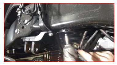
Install the ReadyLIFT bump stop extension to the frame by threading it into the existing bolt hole. Use a punch or similar tool in the holes of the mount and tighten. Install the bump stop mount to the extension using M8 nut and washer. Mark a line across the edge of the outer lip of the bump stop mount parallel to the frame.
