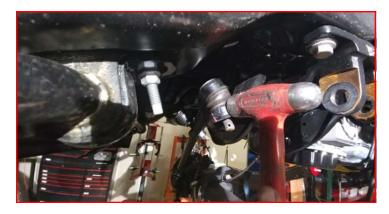
Remove the steering stabilizer from the frame.
