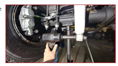
Loosen but do not remove the passenger side u-bolts. Remove the driver side u-bolts completely and lower the axle.
