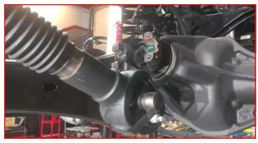
Remove the transfer case skid plate.
