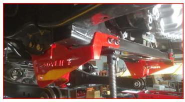
Rotate the axle by lowering the jacks under the tie rod ends until you can line up the radius arms into the ReadyLIFT drop brackets. Install using factory hardware. Do not tighten at this time. Torque the transmission cross member bolts to 40 ft-lbs, and the transmission mount to 65 ft-lbs if installing the 8" lift.
