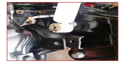
Lower the axle enough to remove the front springs. Remove the shock from the frame.
