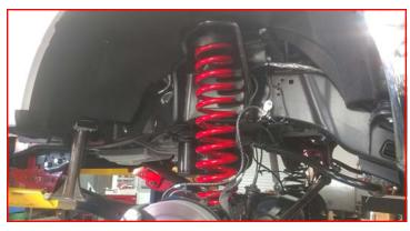
Install the ReadyLIFT sway bar brackets to the frame using factory hardware. Torque to 45 ft-lbs.
