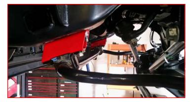
Install the ReadyLIFT sway bar end links to the sway bar using the supplied nuts. Torque to 45 ft-lbs.
