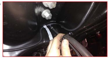
Remove the vacuum line clip from the passenger side engine cross member.
