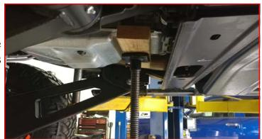
8" lift kit step only: Remove the transmission cross member from the vehicle.
