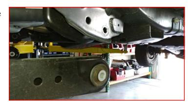
Install the ReadyLIFT radius arm drop bracket into the frame using M18 x 130mm bolts, washers, crush sleeve, nuts and the factory cross member bolts. Do not tighten at this time. Move the jack holding the cross member to the opposite side and repeat above steps.
