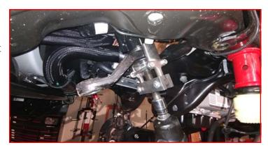
Install the ReadyLIFT pitman arm using the factory nut. Remove the nut, and clean off any lubricant from the sector shaft and pitman arm nut threads and apply a liberal amount of thread locker. Run tight. Use a chain or other suitable strap through the pitman arm tie rod mounting hole to the passenger side frame rail to keep gear box from turning. Torque the pitman arm nut to 450 ft-lbs.
