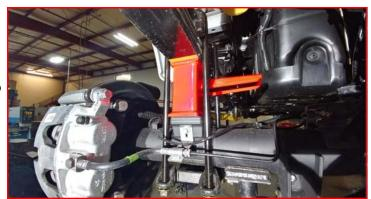
If the vehicle is equipped with the factory sway bar, install the ReadyLIFT rear sway bar brackets to the frame using factory hardware. Torque to 45 ft-lbs.
