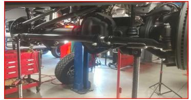
Remove the radius arms at the frame. Use the jack to rotate the axle up allowing the radius arms to drop out of the frame low enough to clear the ReadyLIFT radius arm drops.
