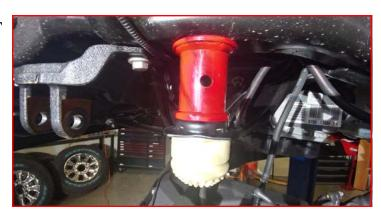
Remove the pitman arm nut. Using a pitman arm puller, remove the pitman arm from the gear box. Clean off any debris off the sector shaft. Coat the sector shaft splines with a light duty liquid based lubricant or oil.
