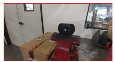
Re-install bump stop mount to the ReadyLIFT extension making sure the cut edge faces to the outside of the vehicle. Torque to 5 ft-lbs.
