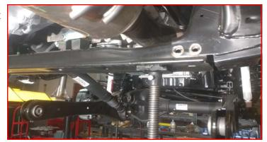
8" lift kit step only: Support the transmission with a suitable jack and a block of wood on the pan closest to the cross member. Make sure to not dent the pan. Remove the wiring harness clips from the cross member.
