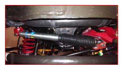
Make a mark 2.5" below the original vacuum line mount on the passenger side engine cross member. Drill a hole using 3/8" drill bit. DO NOT drill into the oil pan. Install the vacuum line clip into the newly drilled hole.
