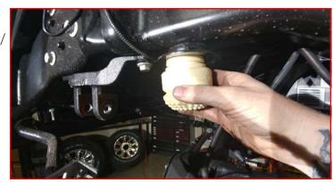
Remove the bump stop mount from the frame.
