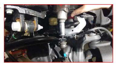
Remove the sway bar from the frame. Note orientation of the bar for re-installation.
