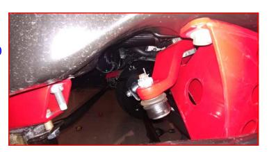
Install the ReadyLIFT steering stabilizer bracket to the frame using M12 x 35mm bolt and washer. Do not tighten until the stabilizer has been test fit so as to establish the brackets final orientation.
