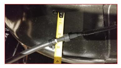
Locate the forward hole on the driver side spring mount on the bottom of the frame rail. Drill into frame rail using 3/8" drill bit. Install the differential vent line clip into the hole.
