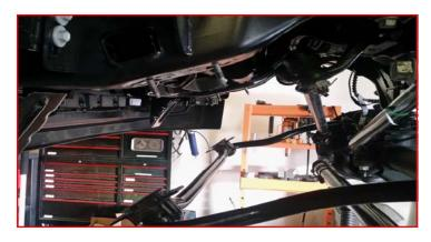
Remove the track bar at the track bar bracket. Let hang out of the way.
