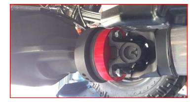
If equipped with a 2 piece driveline, remove the bolts holding the carrier bearing to the frame. Install the ReadyLIFT carrier bearing spacer between the carrier bearing and frame using 7/16" bolts, washers and a drop of thread locker. Torque to 50 ft-lbs.
