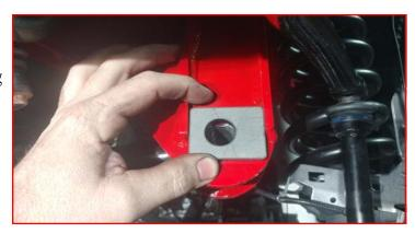
Install the factory isolator onto the ReadyLIFT springs, and then the springs onto the axle making sure to clock the dead end of the spring into the spring lock. Raise the axle enough to hold the springs into place. Install the front extended length shock to the frame using provided hardware and to the axle using factory hardware. Do not tighten at this time.
