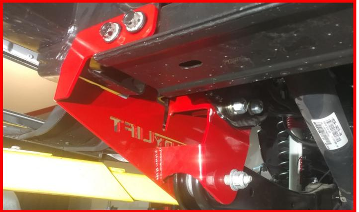
Remove the jacks from under the tie rod ends and place under the axle.
