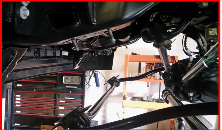
Remove the track bar at the track bar bracket. Let hang out of the way. Retain factory hardware.
