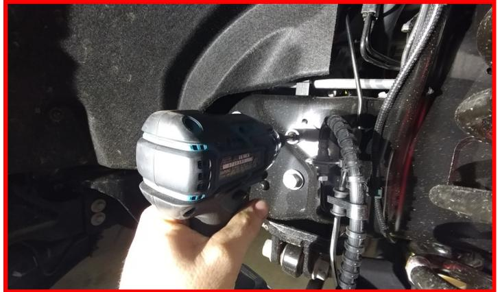
Remove the brake line bracket at the axle. Retain factory hardware.
