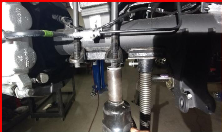
Install the ReadyLIFT driver side block (D is cut into the block under the bump stop tang) and raise the axle lining the center pins up. Install using the provided u-bolts and nuts but do not fully tighten at this time. Repeat steps for the passenger side. (P is cut into the block under the bump stop tang)
