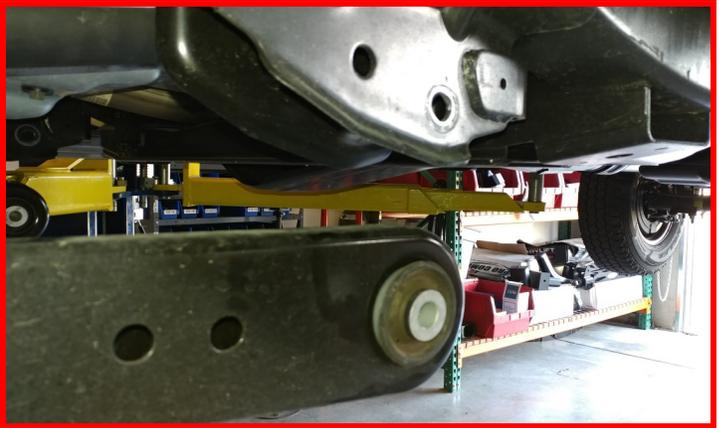
Support the transmission cross member with a suitable jack. Work on one side at a time, remove the cross member bolts. They will be used to mount the radius arm drops. Retain factory hardware.
