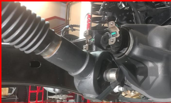
Remove the transfer case skid plate. Retain factory hardware.
