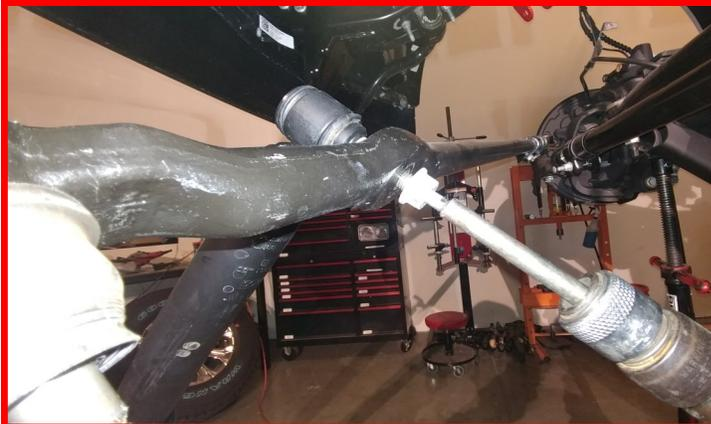
Remove the shock from the axle. Retain factory hardware.
