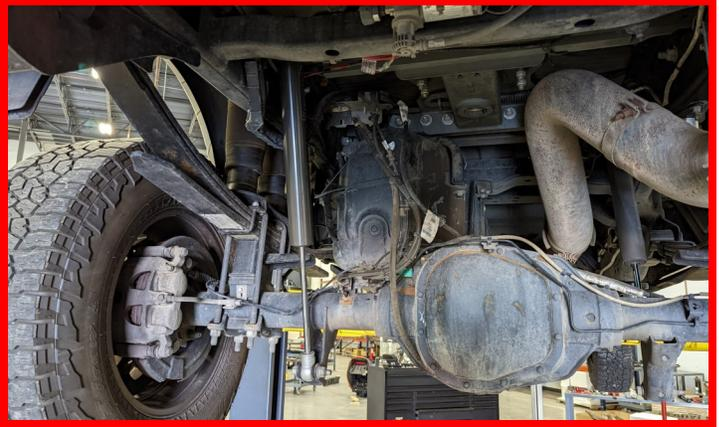
If the vehicle is equipped with the factory sway bar, install the ReadyLIFT rear sway bar brackets to the frame using **factory hardware**. Torque to **45 ft-lbs**.
