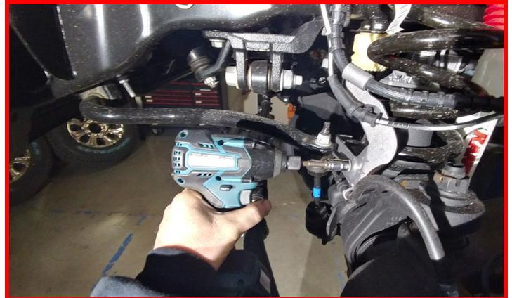
Remove the vacuum line clips from the driver side radius arm.
