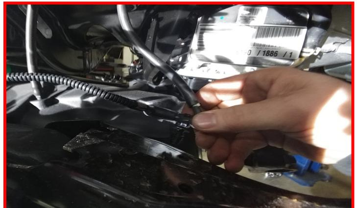
Remove the axle vent line tube from the top of the driver side shock and the inside frame rail.
