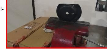
Re-install bump stop mount to the Ready-LIFT extension making sure the cut edge faces to the outside of the vehicle. Torque to 5 ft-lbs.
