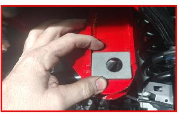
Loosen the tie rod adjuster and flip the tie rod 180 degrees and install to the Ready-LIFT pitman arm using factory hardware. Torque to 70 ft-lbs. Install the safety keeper and cotter pin.
