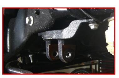
Install the ReadyLIFT pitman arm using the factory nut. Remove the nut, and clean off any lubricant from the sector shaft and pitman arm nut threads and apply a liberal amount of thread locker. Run tight. Use a chain or other suitable strap through the pitman arm tie rod mounting hole to the passenger side frame rail to keep gear box from turning. Torque the pitman arm nut to 450 ft-lbs.
