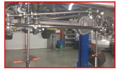
Remove the sway bar from the frame and let hang. Retain factory hardware.
