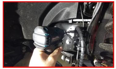
Remove the brake line bracket at the axle. Retain factory hardware.
