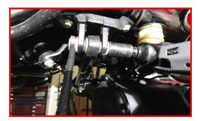
Remove the tie rod end at the pitman arm. Strike the pitman arm with a dead blow hammer to dislodge the taper. Retain factory hardware.
