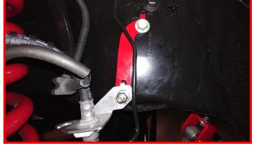
If your vehicle is equipped with a rear sway bar, remove the brackets from the frame and let the sway bar hang out of the way. Retain factory hardware.
