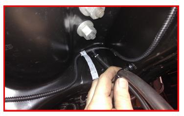
Remove the vacuum line clip from the passenger side engine cross member.
