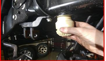
Remove the bump stop mount and use a suitable cutting device, trim off the marked edge. This is for spring clearance under suspension full droop and articulation. Paint the exposed metal with a guality rust preventative paint.
