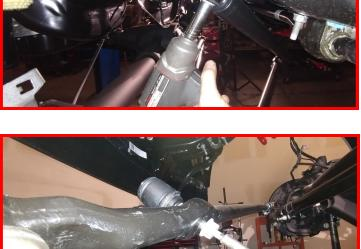
Lower the axle enough to remove the front springs. Remove the shock from the frame. Discard factory shocks and springs.
