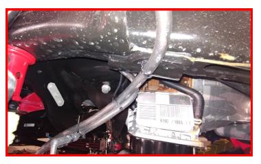
Install the ReadyLIFT brake line extensions to the factory brackets using 5/16" x 3/4" bolts, washers, and nuts. Install bolts facing outwards.
