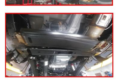
Leave the axle hanging from the shocks. Place a suitable jack under the tie rod ends close to the knuckles.
