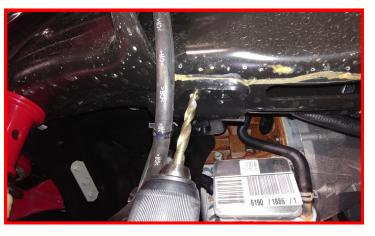
Zip tie the driver side vacuum line to the vent tube making sure that it can not be pinched by the bump stop when the suspension cycles.
