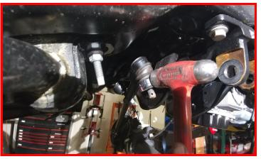
Remove the steering stabilizer from the frame. Retain factory hardware.
