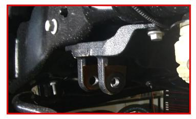
Remove the pitman arm nut. Using a pitman arm puller, remove the pitman arm from the steering gear box. Clean off any debris off the sector shaft. Coat the sector shaft splines with a light duty liquid based lubricant or oil.
