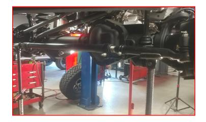
Remove the radius arms at the frame. Use the jack to rotate the axle up allowing the radius arms to drop out of the frame low enough to clear the ReadyLIFT radius arm drops.
