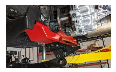
Use a jackstand to hold up one side of the crossmember and install ReadyLIFT Radius Arm Drop Bracket using provided M18 x 130mm bolts, washers, crush sleeve, nuts and the factory cross member bolts. Do not tighten at this time. Repeat for other side.
