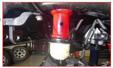
Remove factory track bar bracket by removing the 2 vertical bolts and 3 horizontal bolts. Retain factory hardware.
