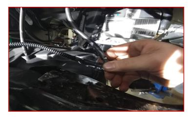
Remove the axle vent line tube from the top of the driver side shock and the inside frame rail.
