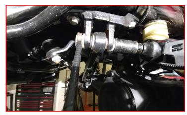
Remove the shock from the axle.
