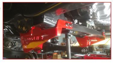
Install the provided M12 nuts and washers to the bottom transmission studs and torque to 65 ft-lbs.
