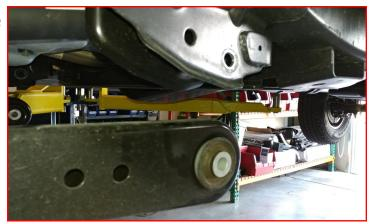
Using one bolt on each side, line up the ReadyLIFT Transmission Crossmember and put the bolts through. Do not install the nuts at this time.
