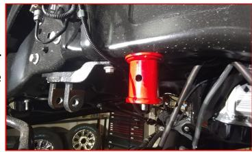
Remove the bump stop mount and use a suitable cutting device, trim off the marked edge. This is for spring clearance under suspension full droop and articulation. Paint the exposed metal with a quality rust preventative paint.
