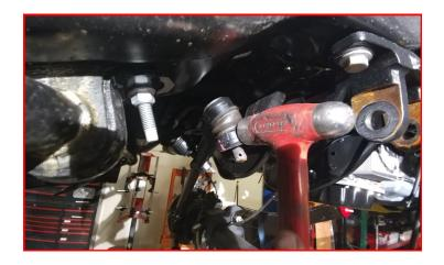
Remove the steering stabilizer from the frame.
