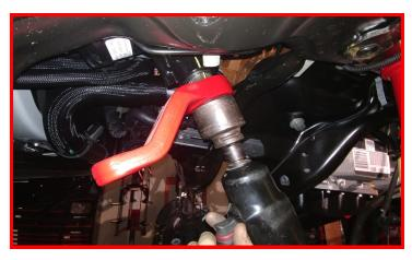
Install the ReadyLIFT track bar mount to the frame using factory hardware. Torque to 120 ft-lbs.
