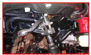
Install the ReadyLIFT pitman arm using the factory nut. Remove the nut, and clean off any lubricant from the sector shaft and pitman arm nut threads and apply a liberal amount of thread locker. Run tight. Use a chain or other suitable strap through the pitman arm tie rod mounting hole to the passenger side frame rail to keep gear box from turning. Torque the pitman arm nut to 450 ft-lbs.
