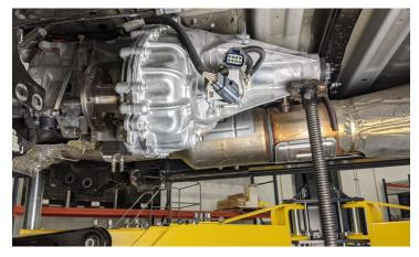
Using a transmission jack, support the transfer case and remove the 11 bolts attaching it to the vehicle. Making sure to keep the transfer case level, back it off the transmission output shaft and carefully lower it from the vehicle. Set aside in a safe location.
