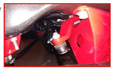
Install the ReadyLIFT steering stabilizer bracket to the frame using M12 x 35mm bolt and washer. Do not tighten until the stabilizer has been test fit so as to establish the brackets final orientation.
