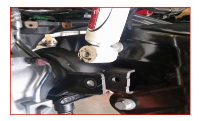
Lower the axle enough to remove the front springs. Remove the shock from the frame.
