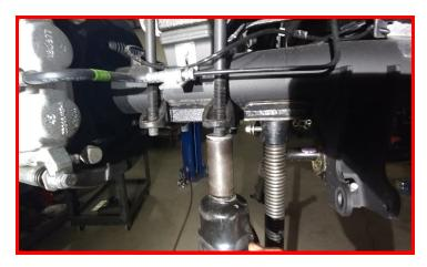
Take care as you are working with a spring that is under pressure. Use a suitable clamp around the leaf pack to hold the pressure, remove the center pin holding the leaf pack together. Undo the clamp and remove the lower overload from the pack. Discard the overload spring.
