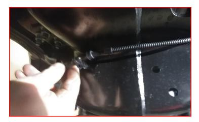
Remove transfer case skid plate. Retain factory hardware.
