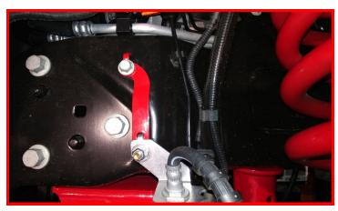
Passenger side: gently unbend the metal line until you can line up the ReadyLIFT bracket locking tang into the original bolt hole. Make sure to not kink the metal line. Install using factory hardware. Do not over tighten and strip the threads.
