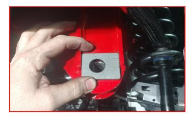
Install the factory isolator onto the Ready-LIFT springs, and then the springs onto the axle making sure to clock the dead end of the spring into the spring lock. Raise the axle enough to hold the springs into place. Install the front extended length shock to the frame using provided hardware and to the axle using factory hardware. Do not tighten at this time.
