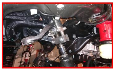
Install the ReadyLIFT pitman arm using the factory nut. Apply a liberal amount of thread locker. Run tight. Use a chain or other suitable strap through the pitman arm tie rod mounting hole to the passenger side frame rail to keep gear box from turning. Torque the pitman arm nut to 450 ft-lbs.
