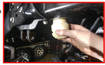
Remove the bump stop mount from the frame. **Discard factory hardware.**
