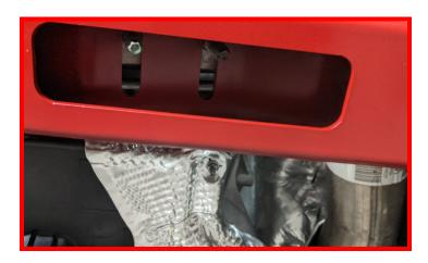
Remove the sway bar from the frame. Note orientation of the bar for reinstallation.
