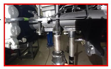
Take care as you are working with a spring that is under pressure. Use a suitable clamp around the leaf pack to hold the pressure, remove the center pin holding the leaf pack together. Undo the clamp and remove the lower overload from the pack. **Discard the overload spring.**
