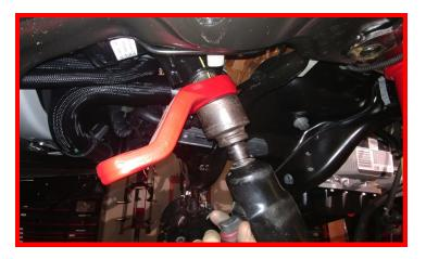
Install the ReadyLIFT track bar mount to the frame using factory hardware. Torque to 120 ft-lbs.
