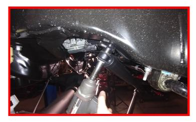
Remove the steering stabilizer nut from the drag link. Dislodge the taper to remove the steering stabilizer. **Discard factory steering stabilizer.**
