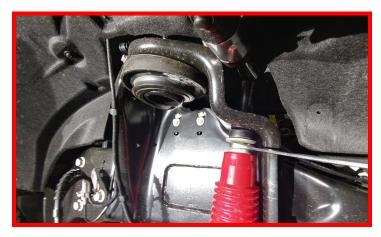
Install the Falcon front shock using the provided hardware on the top and the factory hardware on the bottom attachment.
