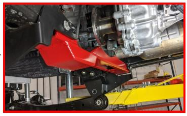
Install the provided M12 nuts and washers to the bottom transmission studs and torque to 65 ft-lbs.
