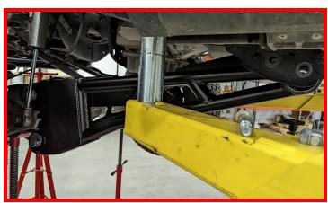
Torque radius arm pivot bolt to 200 ft-lbs.
