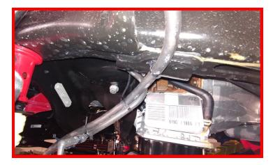
Install the ReadyLIFT brake line extensions to the factory brackets using 5/16" x 3/4" bolts, washers, and nuts. Install bolts facing outwards.
