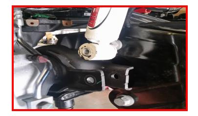
Lower the axle enough to remove the front springs. **Discard factory springs**.
