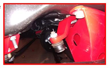
Install the ReadyLIFT steering stabilizer bracket to the frame using M12 x 35mm bolt and washer. Do not tighten at this time. The stabilizer must be test fit to establish the bracket's final orientation.
