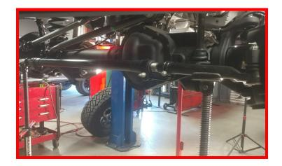
Unbolt the radius arms at the frame. Use the jacks to rotate the axle, allowing the radius arms to drop out of the frame. Lower the radius arms at least 7" from the pivot hole in order to allow for new arms to be installed.
