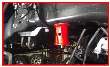
Mark a line across the edge of the outer lip of the passenger side bump stop mount parallel to the frame.
