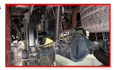
If equipped with a 2 piece driveline, remove the bolts holding the carrier bearing to the frame. Install the ReadyLIFT carrier bearing spacer between the carrier bearing and frame using 7/16" bolts, washers and a drop of thread locker. Torque to 50 ft-lbs.
