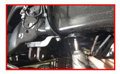
Install the ReadyLIFT bump stop extension to the frame by threading it into the existing bolt hole. Use a punch or similar tool in the holes of the mount and tighten. Install the driver side bump stop mount to the extension using M8 nut and washer.
