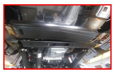
Support transfer case with jackstand near the output shaft. Remove factory cross member and discard.
