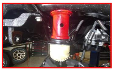
Remove factory track bar bracket by removing the 2 vertical bolts and 3 horizontal bolts.
