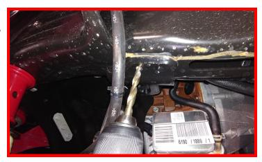
Zip tie the driver side vacuum line to the vent tube making sure that it can not be pinched by the bump stop when the suspension cycles.
