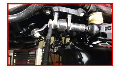
Remove the drag link at the pitman arm. Strike the pitman arm with a dead blow hammer to dislodge the taper.
