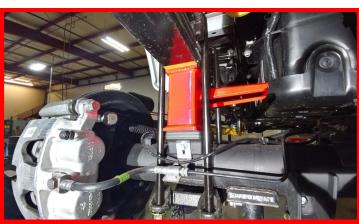
If the vehicle is equipped with the factory sway bar, install the ReadyLIFT rear sway bar brackets to the frame using factory hardware. Torque to 45 ft-lbs.
