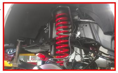
Loosen the tie rod adjuster and flip the tie rod 180 degrees and install to the Ready-LIFT pitman arm using factory hardware. Torque to 70 ft-lbs. Install the safety keeper and cotter pin.
