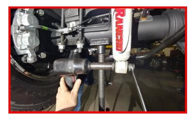
Loosen but do not remove the passenger side u-bolts. Remove the driver side u-bolts completely and lower the axle. **Discard factory hardware.**
