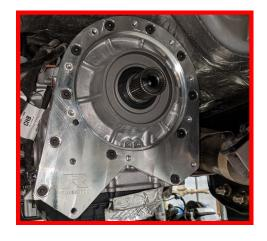
Re-install transfer case using the provide M10-1.5 x 35mm Hex Bolts. Using a star pattern, torque bolts to 50 ft-lbs.
