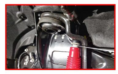
Remove the **shock** from the frame. **Discard factory shock and upper shock** hardware.
