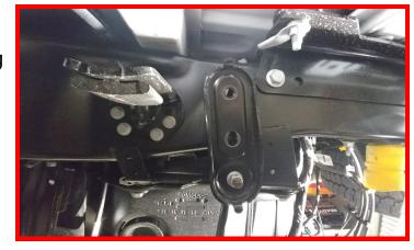
Support the axle with a suitable jack. Remove the rear shocks from the axle and frame.
