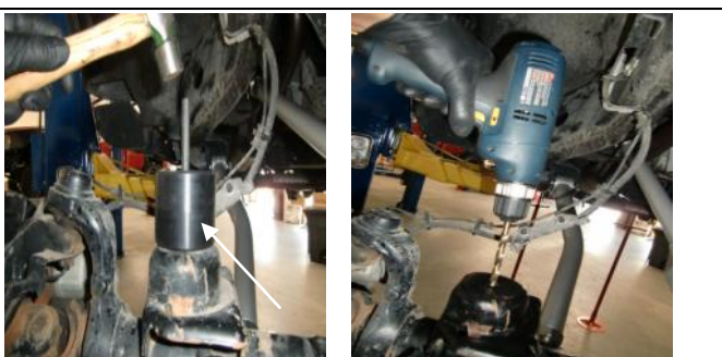
20. Center, mark and drill 11/32" hole.
