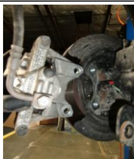
31. Unbolt and remove rear brake caliper and hang caliper out of the way.
