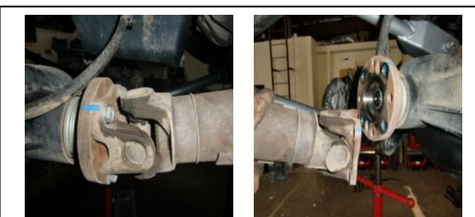
11. Mark drive shaft for re-alignment during reassembly. Unbolt the drive shaft from the front differential.
