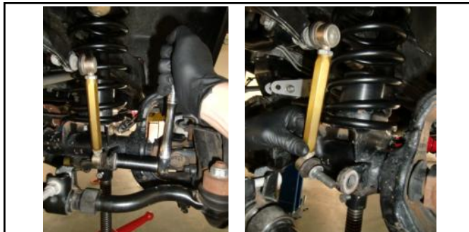
6. Unbolt and remove the sway bar end links from vehicle.
