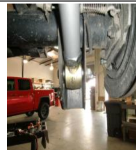
36. Install new lower arms and tighten down. The adjustable end should be installed on axle side.
