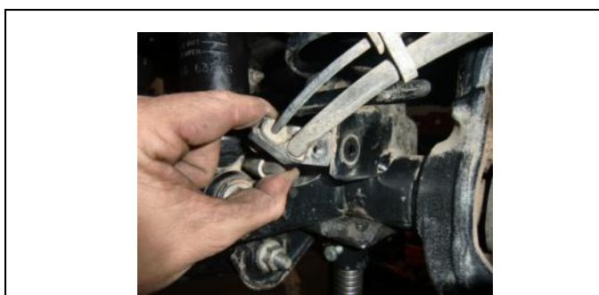
7. Unbolt and dislodge the brake line brackets from the axle.
