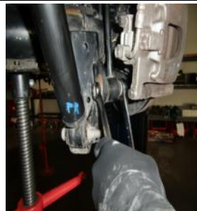
30. Unbolt the rear sway bar end links and remove.
