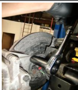
31. Unbolt and remove rear brake caliper and hang caliper out of the way.
