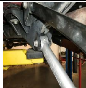
36. Install new lower arms and tighten down. The adjustable end should be installed on axle side.
