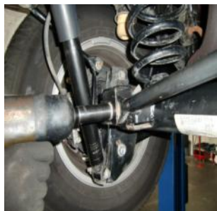
29. Unbolt and remove the rear track bar. Support the rear axle.
