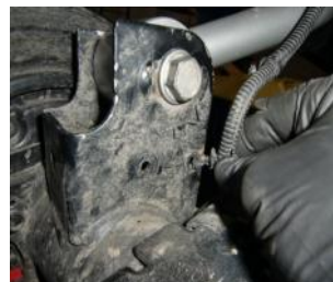
33. Remove ABS line clips from holes in rear axle. Put the back clip into the front hole.
