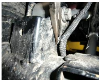
33. Remove ABS line clips from holes in rear axle. Put the back clip into the front hole.
