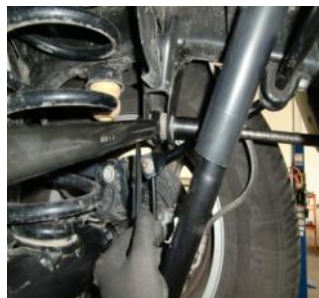
29. Unbolt and remove the rear track bar. Support the rear axle.
