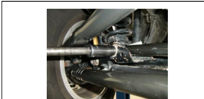
5. Next, unbolt the track bar from the axle and remove from vehicle.
