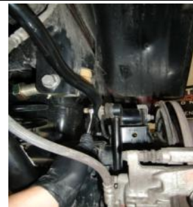
30. Unbolt the rear sway bar end links and remove.
