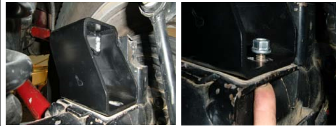
39. Install new bump with supplied hardware. Bump stop pad should be leaning towards front of vehicle.
