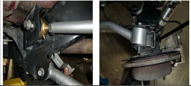
38. Install the new rear upper arms. Adjustable ends should be installed on frame side and the zerker fittings up on axle side.
