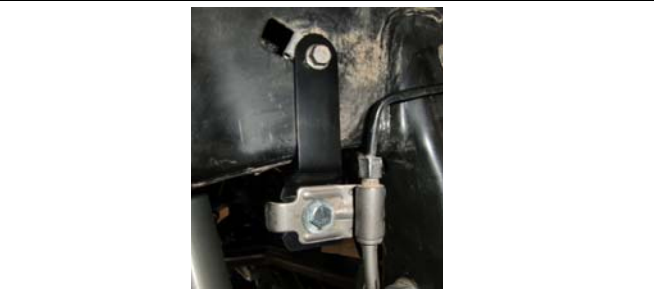
41. Unbolt the brake line brackets from the frame and install the brake line drop brackets with supplied hardware.
