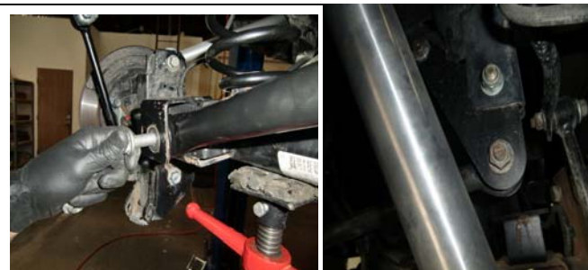
43. Install track bar into the frame pocket and axle mount.
