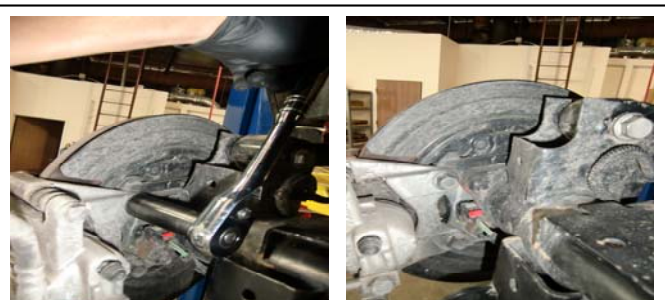
44. Re-install the brake calipers and torque.
