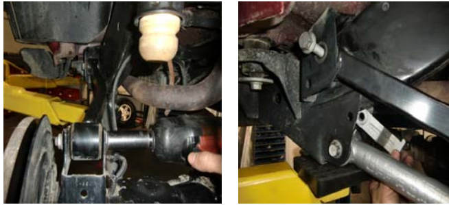
37. Unbolt both rear upper arms and remove from vehicle.
