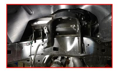
Install the supplied upper control arms using the factory hardware.
