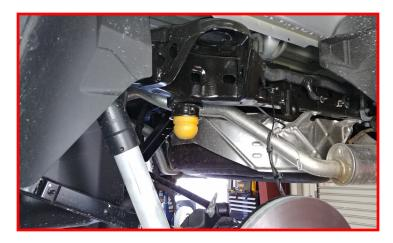
The rubber isolator has two locating nipples on it. Use a suitable cutting device, remove these flush with the isolator.
