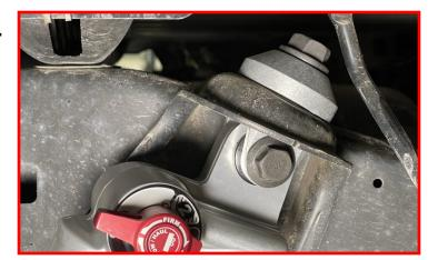
Before tightening, ensure the body cap has clearance to shock tower
