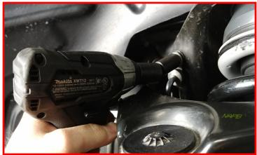
Remove the ABS wire harness from the upper control arm and frame rails. Cut the Christmas tree clip off the harness. Do not cut the ABS wire.
