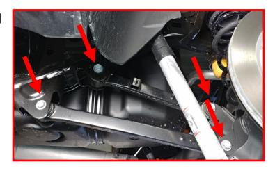
Loosen but do not remove the track bar hardware at the frame and axle ends.
