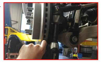
Strike the tie rod boss on the knuckle with a dead blow hammer to dislodge the taper.
