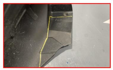
Install the fender liner back into the factory location.
