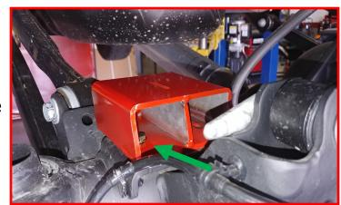
The passenger side you will use the bolt hole on the right inside hole of the bump extension. This will line up with the hole in the axle pad. The forward mounting hole is slotted to line up with the axle pad hole. Once the inside bolt is lined up, install the front bolt, washer, and nut.
