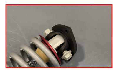
NOTE: AFTER INSTALLING THE TOP HATS, ENSURE YOU HAVE INN FACT ASSEMLED A LEFT AND A RIGHT COILOVER.
