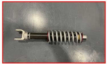
Install the coilover into the top hat using the supplied M16 Flange bolt and M16 locking flange nut.
