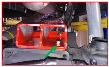
Install the ReadyLIFT spring spacer, factory isolator and then spring to the frame and axle.
