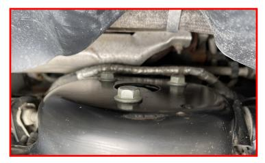
Raise the lower control arm up until you can install the supplied lower strut hardware.
