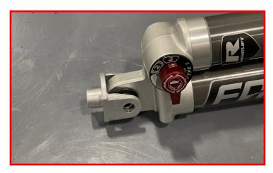
Install the M14 flanged bolt through the upper shock clevis from the outside in (from the dial side in). Install the locking flange nut.
