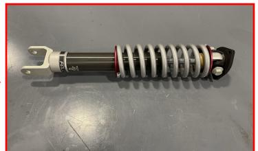
Install the completed coilover assembly into the vehicle. Be sure the lower mount is offset away from the cv axle.
