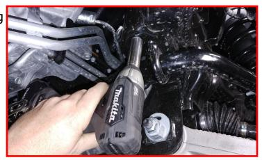
Install the front wheels and lower the vehicle to the ground. Torque the lug nuts to the wheel manufacturers specs.
