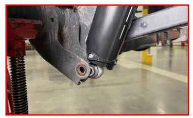
Install the sway bar end links to the frame rail using the factory hardware. Do not tighten at this time. Install the brake line brackets to the frame rail using the factory hardware. Torque to 5 ft-lbs.
