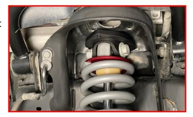
Install the coilover top hat adaptor plate, using the supplied thread locker and M10 flanged head bolts.
