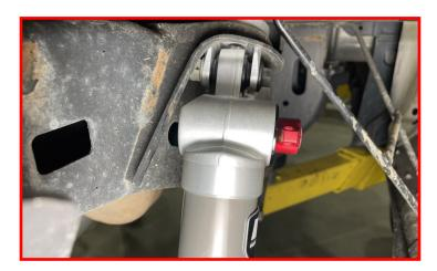
Raise the axle high enough to install the factory shock hardware.
