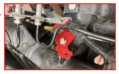
Install the supplied M6 x 16mm bolt, washer and locking nut through the bottom hole on the relocation bracket.
