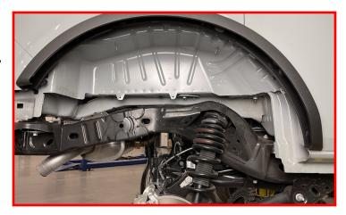
To aid in the removal and installation process, it is best to loosen the rear track bar at the frame.
