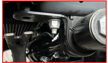
Install the driver and passenger rear sway bar retainer cap bolt.
