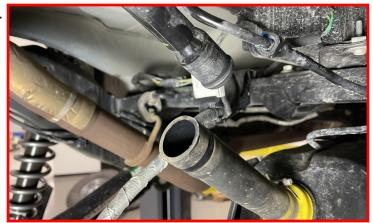
Remove the (2) bolt shield screws on the inside of the right frame rail. These are located on the rear lower control arm pivot bolt.
