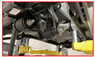
RAISE THE REAR AXLE FOR THE SERIES OF STEPS, THIS WILL ADD IN THE RE-MOVAL AND INSTALLATION ON THE REAR UPPER CONTROL ARM HARDWARE.
