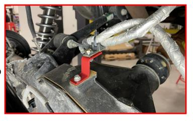
When opening the package with the rear shocks, you will notice that the lower eyelet may be rotated 90 degrees.
