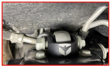
Raise the lower control arm up and guide the lower strut into place. Install the \*\*\*\* through the lower control and the coilover bar pin.
