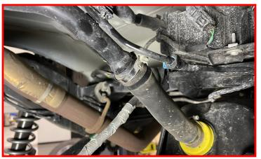
Remove the metal filler tube from the rubber coupler on the fuel tank.
