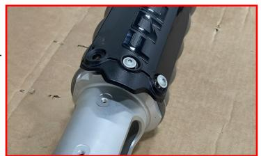
Install the last spacer between the coil carrier and roost guard.
