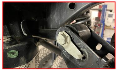
Install the factory nut onto the rear upper control arm pivot bolt.
