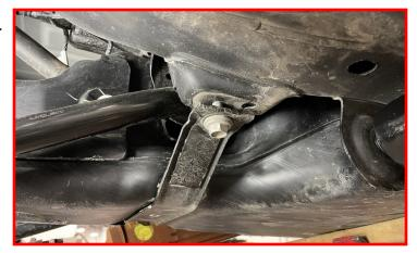
Remove the ABS harness bracket located on the top of the rear axle housing.
