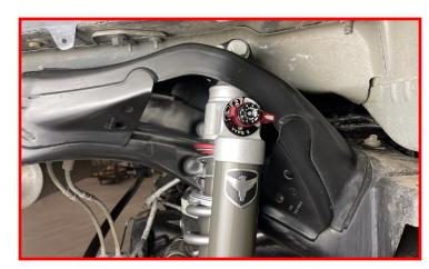
Install the supplied M16 through the top hat and the body cap bearing.
