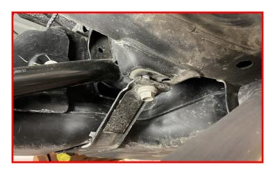
Loosen the hose clamp on the gas filler neck and slide up the metal filler tube.
