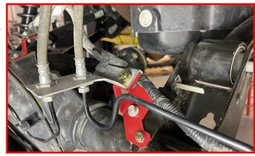
Install the ABS relocation harness bracket on the top of the rear axle housing in the factory orientation using the factory hardware.
