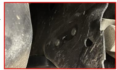
Remove the rear lower control arm mounting hardware.
