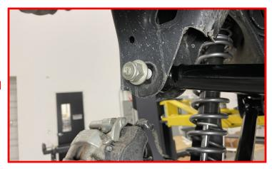
Using an appropriate jack, support the axle.
