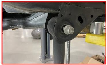
Carefully support the fuel tank with an appropriate jack.
