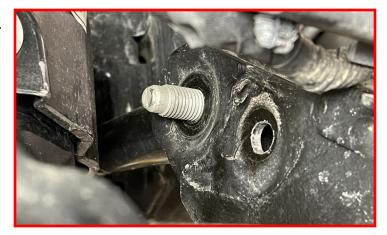
Remove the factory bolt from the rear upper control arm mount.
