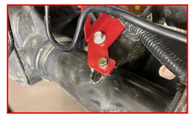
Install the supplied M8 x 20mm bolt, washer and locking nut through the factory brake line bracket and top hole on the relocation bracket.
