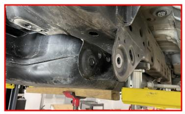
Using the factory hardware, install the replacement real lower control arm.
