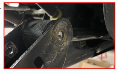
Install the factory bolt into the rear upper control arm mount from inside to outside. Ensure the flag bolt is inserted into the hole that was drilled out.
