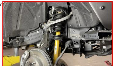
Install the coilover top hat adaptor plate, using the supplied thread locker and M10 flanged head bolts.
