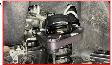
Install upper ball joint to knuckle using the supplied hardware.
