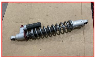
The lower coil carrier has (4) mounting holes used to mount the supplied roost guard.
