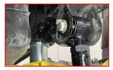
Using the factory the pivot bolt install the rear lower control arm into the factory lower control arm pocket.
