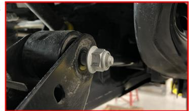
Remove the factory nut from the rear lower control arm pivot bolt.
