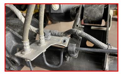
Unclip the brake line from bracket.
