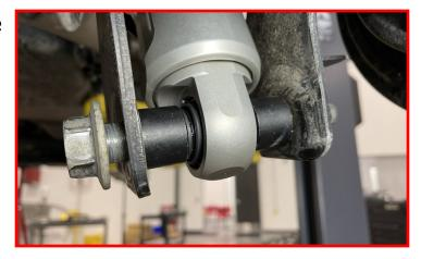
Install the factory flag nut onto the lower shock bolt.
