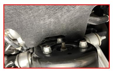
Remove the lower strut nuts.
