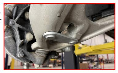
Install the provide M14 locking flange nuts.
