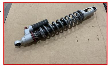
Rotate the lower eyelet 90 degrees to align with the upper mount.
