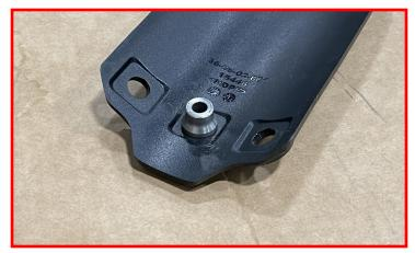
Using thread locker and the supplied M6 button screw, install the roost guard on the second from the right for the driver side and second from the left for the passenger.
