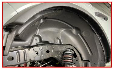
Remove the rear fender liners.
