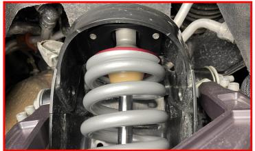
Install the provided M16 Flange bolt through the top hat and coilover from front to rear.
