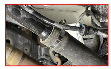
Install the rear tank strap using the factory hardware.
