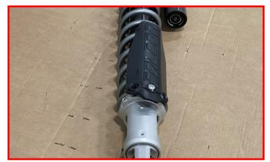
Install the second spacer between the coil carrier and roost guard.
