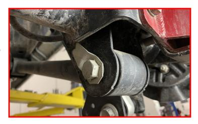
Remove the factory nut from the rear lower control arm frame pivot bolt. Carefully let the control arm swing down out of the way.
