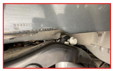
Install the lower coilover mount using the factory bolt and supplied spacers.
