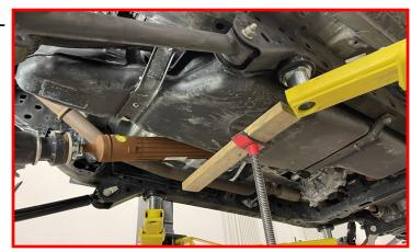
Loosen but do not remove the front tank strap.
