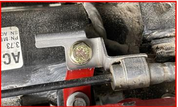
Install the center brake line relocation bracket on the axle using the factory bolt.
