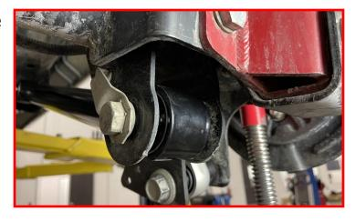
Install the factory nut onto the rear lower control arm pivot bolt.
