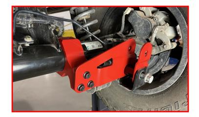
Install the rear track bar into the track bar bracket using the supplied M16 x 90mm hex flange head bolt.
