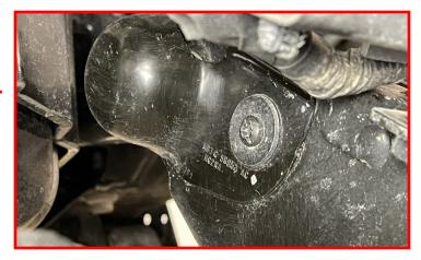
Using a 1/2" drill bit drill out the existing hole used to mount the shield.
