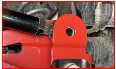
Torque the factory bolt to 120 ft-lbs.
