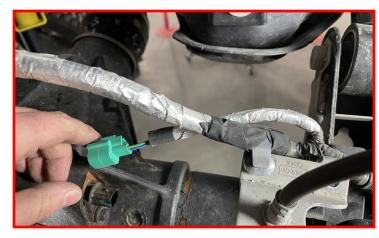
Lastly, reinstall the locker harness connector to the axle housing.
