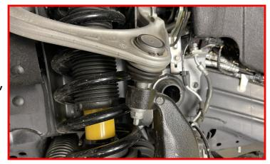
Remove the upper control arm pivot bolt.
