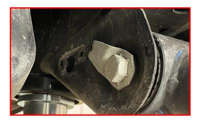
Remove the factory rear lower control arm.
