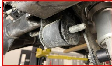
Remove the factory bolt from the rear lower control arm mount.
