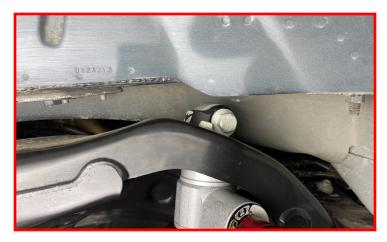
Install the supplied flag nut so the bent ear is to the rear of the vehicle.
