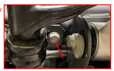
Install both the driver and passenger rear sway bar skid plate bolts.
