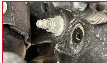
Remove the factory nut from the rear upper control arm pivot bolt.
