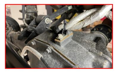
Vehicles equipped with factory rear Elocker will need to disconnect the locker plug.
