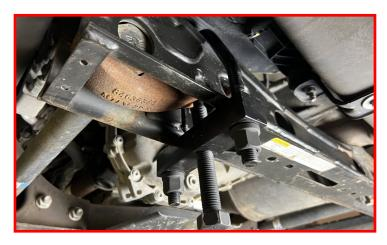
Once the keyway is adjusted high enough, remove the cross pin. DO NOT push it through with your finger. Always pull it out away from the keyway. Once the cross pin is out, remove the torsion bar unloading tool.
