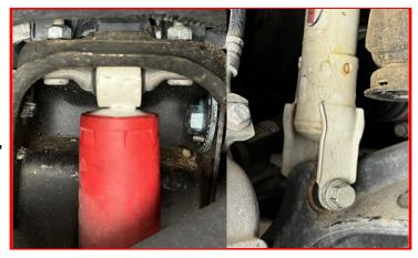
Loosen but do not remove the ball joint nut.
