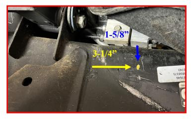
Debur the hole and coat with some type of anti-corrosion coating such as undercoating or paint.
