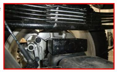
Raise the axle with the ReadyLIFT block installed to the leaf pack. Install the provided U-bolts and hardware. Ensure the lock washer is located between the nut and thick washer. Only snug the U-bolts up enough to hold the axle in place. Repeat all steps on the passenger side. Final torque will be done when the vehicle is on the ground.
