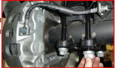
Trim off excess u-bolt length with a suitable cutting tool if desired.
