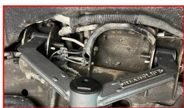
Install the upper control arm ball joint to the factory knuckle using the provided hardware.
