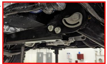
Using factory bolts, install ReadyLIFT rear cross member.
