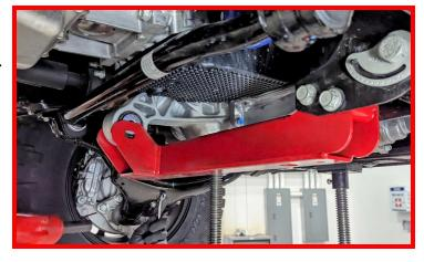
Install factory differential rear support pinion hardware.
