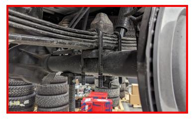
Lower the axle enough to provide space between the leaf spring and the axle mount.
