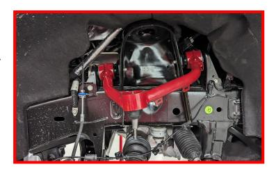
Install Falcon front coilover into the frame using the provided M10 flange nuts.
