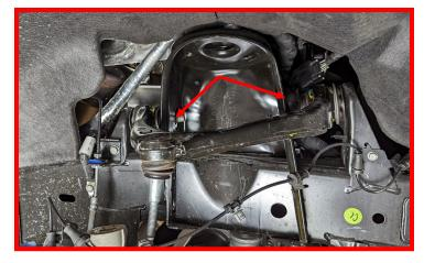
Install ReadyLIFT Upper Control Arm using factory hardware.
