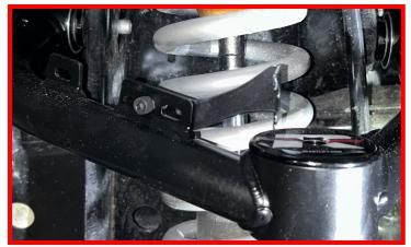
Install oval fir tree zip ties into slots on ABS bracket and control arm bracket and tighten around ABS Line. Cut off excess length of zip tie.
