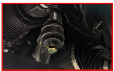
Remove two front bolts holding the plastic brush guard to the crossmember.
