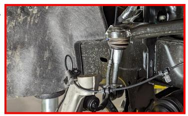
Remove strut assembly from vehicle.
