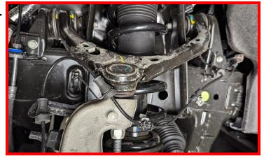
Remove upper control arm to knuckle nut. Allow knuckle to hang out of the way.
