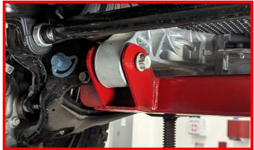
Remove lateral support bolts on either side of the differential.
