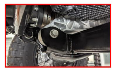
Remove 4 bolts holding factory rear crossmember and remove crossmember from vehicle.
