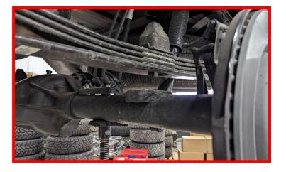
Install the ReadyLIFT rear block between the leaf spring and axle.
