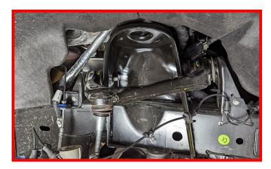
Remove fasteners holding the upper control arm to the frame and remove the upper control arm from the vehicle.
