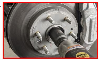
Using a dead blow sledgehammer, strike the end of the axle until it moves back and forth freely. Remove axle nut at this time.
