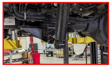
Remove U-bolt nuts and nut plate. Retain nut plate, but discard factory nuts
