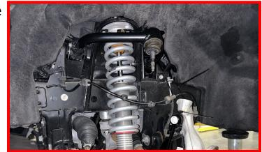
Install Falcon Coilover to lower control arm using provided hardware.
