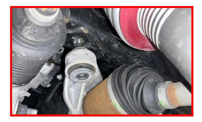
Install ReadyLIFT differential spacers in between differential and frame using the provided M14 bolt and washer.
