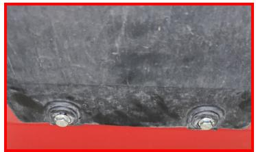
Using the seven provided M8 bolts and washers, install the ReadyLIFT front skid plate. Loosely install the bolts to ensure that ever bolt is able to be installed.
