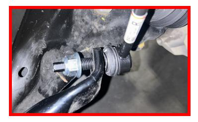
Install ReadyLIFT sway bar link to sway bar using provided hardware.
