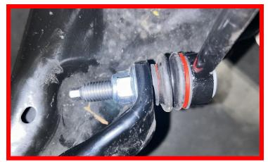
Install ReadyLIFT sway bar link to knuckle using provided hardware.
