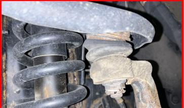
Remove the upper control arm pivot bolt and nut. Remove upper control arm from vehicle.
