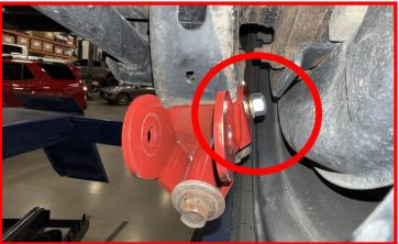
Install the factory lower shock bolt. Torque bolt to 65 ft-lbs.
