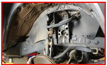
Install the Falcon Upper Strut Mount into the factory strut tower using the supplied nuts. Falcon logo should be facing outward.
