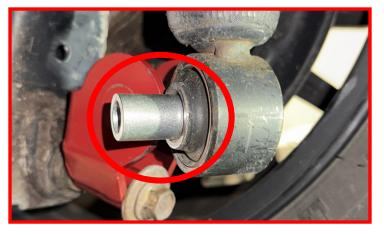
Install the lower shock eye into the ReadyLIFT Rear Shock Extension using the provided M12 x 75mm bolt, M12 locking nut and washers. Ensure that the ReadyLIFT Rear Shock Crush Sleeve is retained.
