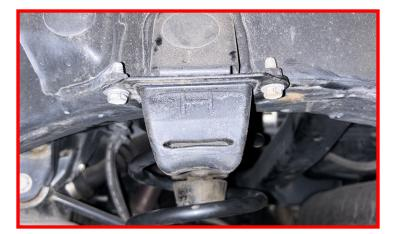
Install the ReadyLIFT Bump Stop Spacer using the provided M8 bolts and washers.
