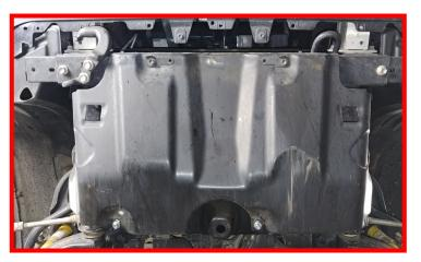
Install the rear of the front gravel guard using the provided M8 x 40mm hardware and spacers. Torque front and rear hardware to 25 ft-lbs.
