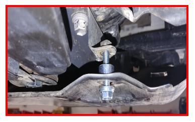
Install the ReadyLIFT skid plate spacers using provided M8 bolts.
