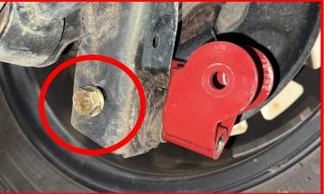
Use the provided M12 locking nut and washers to fix the stabilizing ear to the axle shock bracket.
