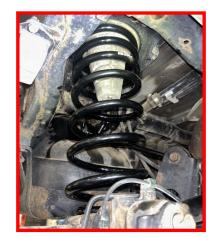
Install ReadyLIFT Rear Shock Extension onto the Lower shock stud.
