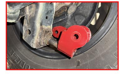
Place the provided M12 x 110mm bolt with a washer all the way through the hole in the axle shock bracket and through the ear on the ReadyLIFT Rear Shock Extension. The bolt will point towards the outside of the vehicle.
