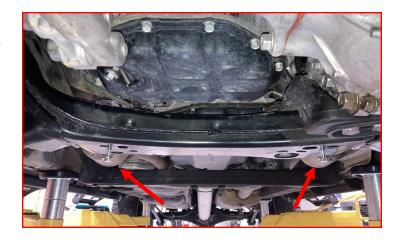
Slide the ReadyLift Skid Plate between the frame and washers.
