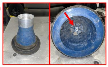
Install the ReadyLift coil spring with the factory isolator and bump stop extension in place.
