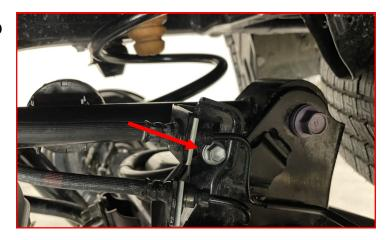
Remove the end link nut and let the end hang out of the way.
