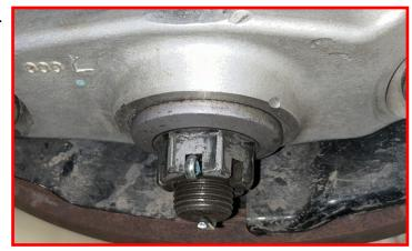
Using the appropriate tool, dislodge the ball joint taper from the steering stop.
