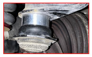
Using factory hardware (installed front to back), install the ReadyLift upper control arm.
