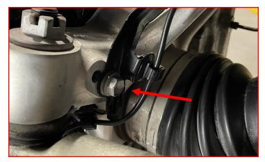
Start the two supplied M8 bolts and washers in the rear crossmember. Leave them loose to slide the slotted holes on the skid plate into place.
