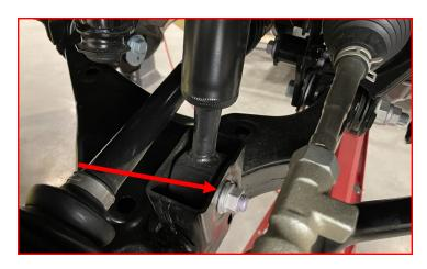
Loosen but **DO NOT** remove the four (4) upper strut bolts.
