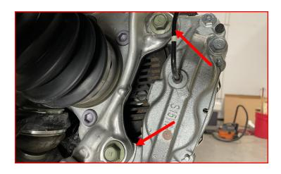
Remove the upper ball joint retaining clip by pushing in on the clip nub.
