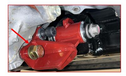
Attach the ReadyLIFT passenger side differential drop bracket to the chassis using factory hardware.
