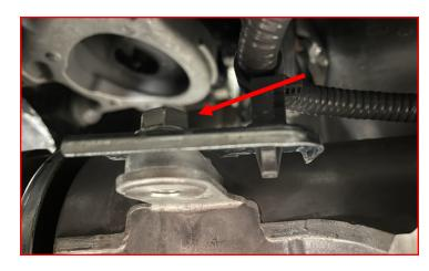
Prepare the front differential drops by pressing the supplied bushings into the differential drop tubes.
