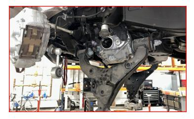
Locate the replacement axle assembly. The axle is etched with the part number on the shaft. The 68-52420CVL is the Left (driver) side and will be the shorter of the two.
