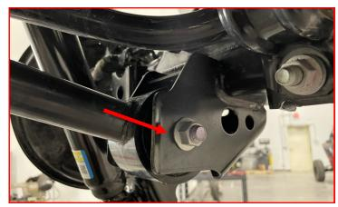
Support the axle using an appropriate jack.
