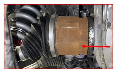
DO NOT TRY TO PRY THE AXLE FROM THE DIFF HOUSING, THIS WILL DAMAGE THE HOUSING AND SEAL.
