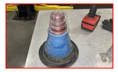
Secure the ReadyLift bump stop extension to the plastic holder using the supplied M10 Bolt and Washer.
