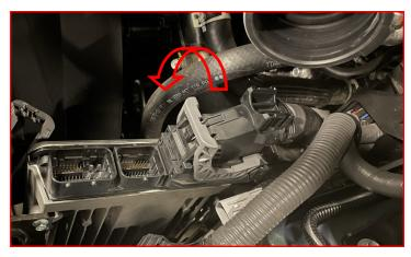
Plug the center plug into the accumulator.
