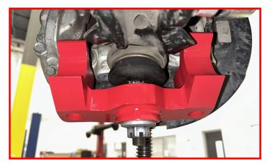
Install the Falcon front coilover top mount using the supplied flange nuts.
