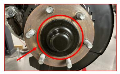
Remove the cotter pin, sleeve, and nut.
