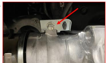
Relocate the bracket from the bottom on the mounting point to the top of the mounting point and attach using the factory hardware.
