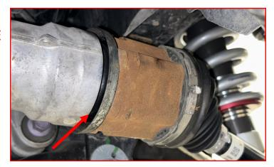
Remove the CV axle assembly from the vehicle.
