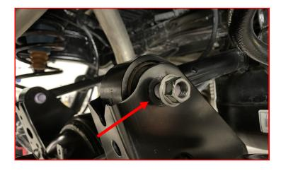
Ensure upper shock mount is assembled with the anti-rotation plate followed by the thick black washer, bushing, and steel shock centering ring as seen in the photo.
