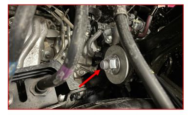
Remove the upper control arm bolt and remove the upper control arm.
