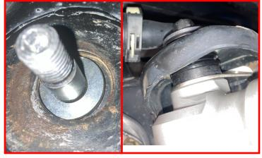
Slide the rear shock over the shock mount and secure using the factory hardware.
