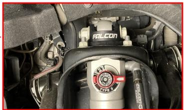
Using the two M6 button head screws, attach the frame mounting tab to the reservoir clamp.
