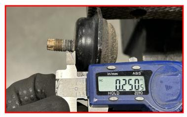
Using an appropriate tool, cut the threads off beyond the 1/4" mark.
