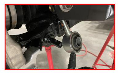
Remove the four (4)(two on each side) sway bar bolts and remove the sway bar from the vehicle.
