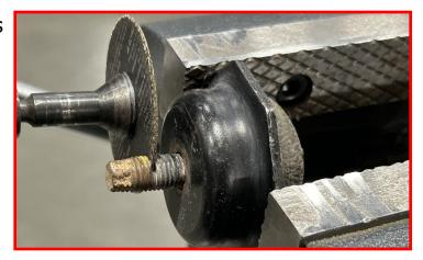
Apply thread locking compound and thread the bump stop extension onto the bump stop.
