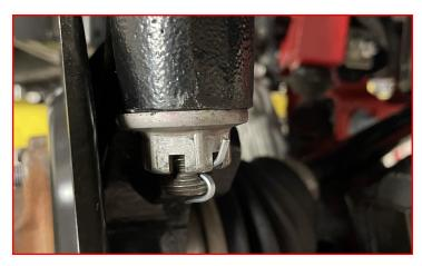
Lower the upper control enough to insert the ball joint stud into the knuckle using the supplied M12-1.75 flange nut and hardened washer.
