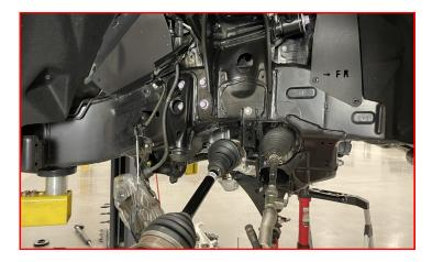
Remove the factory bump stop by unscrewing it from the chassis mount.
