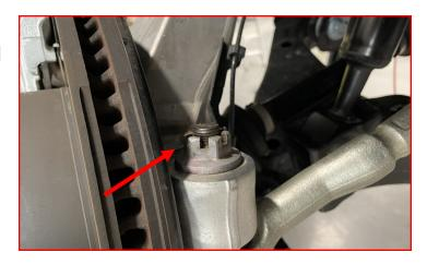
Remove the CV axle dust shield.
