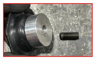
Apply thread locking compound on the supplied bump stop set screw and thread it into the bump stop extension.
