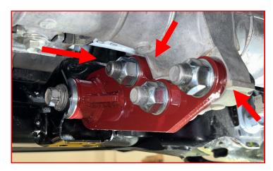
Torque both chassis to differential drop bracket hardware to 110 ft-lbs.
