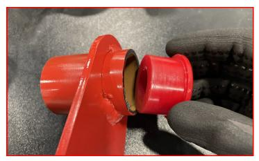
Press the supplied crush sleeve into the bushings and slide the spacers over the sleeves. The sleeve should be about flush with the spacers.
