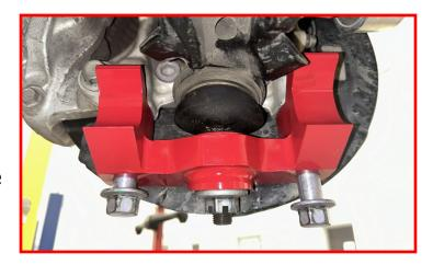
Slide the CV shaft through the hub and install the supplied axle nut.
