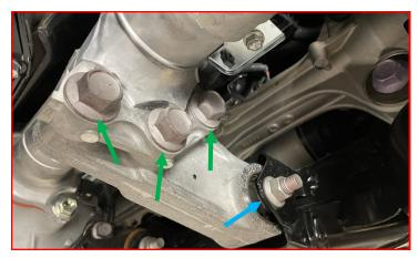
Remove the two bolts holding the driver side bracket to the differential.
