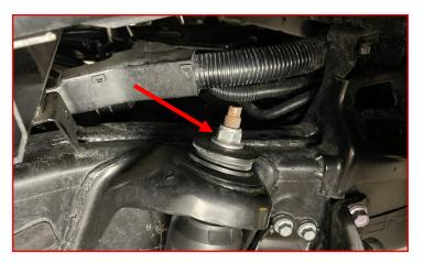
Lower the axle enough to remove the rear springs.
