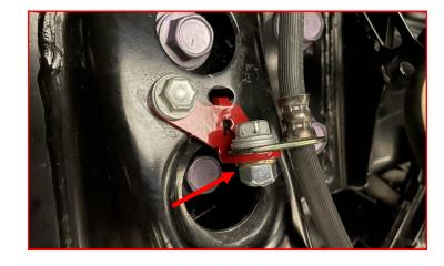
Using factory hardware, attach the ABS sensor wire at the middle of the knuckle.
