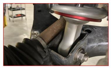
Attach the knuckle to the steering stop using the two factory bolts.
