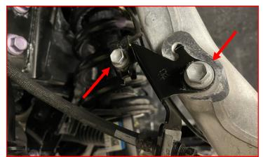
Secure the ABS wire to the ReadyLift upper control arm buy using the supplied fir tree zip ties.
