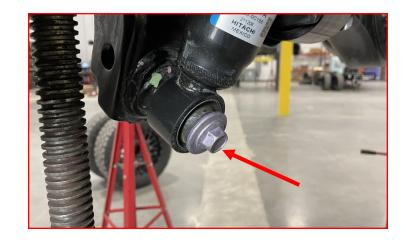
Remove the upper shock nut and bushing.
