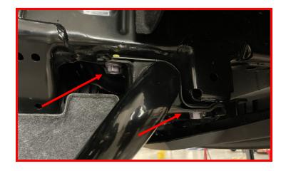
Remove the ABS wire from the factory bracket by gently prying open the 4 retaining tabs.
