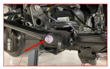
Loosen but **DO NOT** remove the **DRIVER** upper control nut at the axle.
