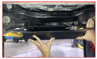
Use the two supplied M8 bolts and washers to secure the front of the skid plate to the crossmember.
