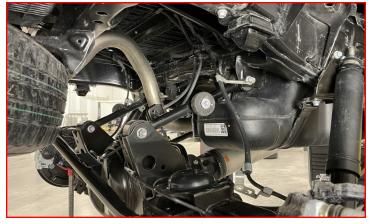
Remove the factory bump stop from the upper spring isolator by prying it out of the plastic holder.
