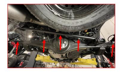
Remove the **bolt** (one on each side) holding the brake line to the axle.
