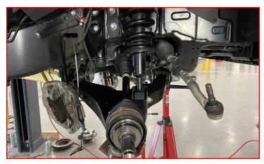
Remove the lower shock bolt, let the lower control arm hang out of the way.
