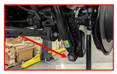
Ensure axle is supported and remove upper shock nut from frame. Remove lower shock bolt and remove shock from vehicle.
