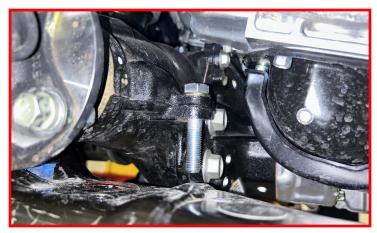
Raise the differential up to allow the install of the replacement diff drop.
