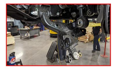
With the aid of a helper, carefully remove the (4) top strut.
