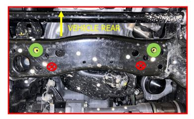
Thread the M8 bolts and washers into the threaded holes indicated in the previous step. Leave enough thread out of the crossmember to slide the skid plate onto the bolts.
