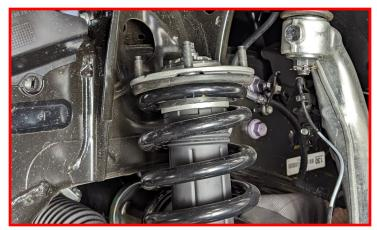
Install Falcon Front Strut top hat into the strut tower using the provided hardware. Install top hat with Falcon logo point out.
