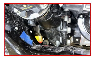
Lower the diff back down, this will allow clearance for the bolt to be remove.
