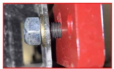
Install the sway bar onto the sway bar extension using the supplied M12 x 20mm hex head bolts, M12 washers and thread locker.
