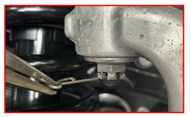
Remove the upper control arm ball joint nut.
