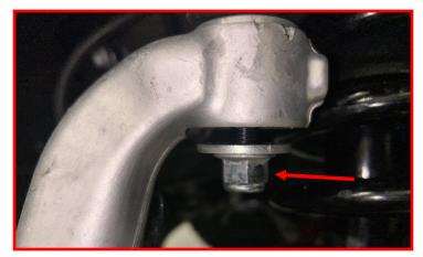
Remove bolts holding lower ball joint cradle to knuckle.
