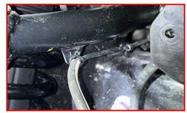
Remove the two bolts holding the dust cover to the front crossmember.
