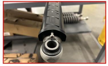
Install Falcon Rear Shock into frame side and loosely install provided nut. Ensure that the tuning knob is pointing toward the rear of the vehicle.
