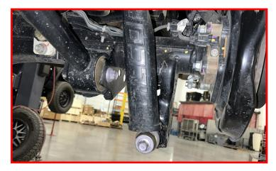
Remove factory bump stop and factory bump stop mount.
