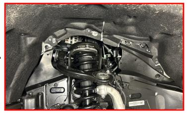
Loosen but do not remove upper control arm bolt.
