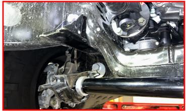
Support the differential with a suitable transmission jack.
