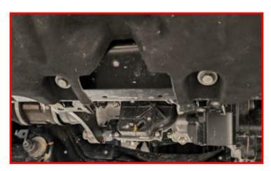
Find the threaded holes in the rear crossmember. M8 bolts will be installed into the rearward, outboard threaded holes. (Avoid installing in the forward, inboard holes).
