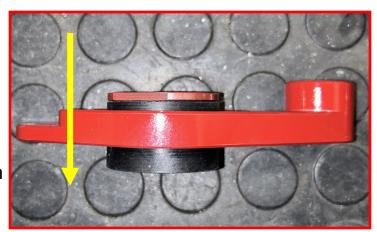
Install the ReadyLIFT rear diff drop using the supplied M12 x 25mm and thread locker.
