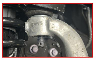
Remove the upper control arm pivot nut.
