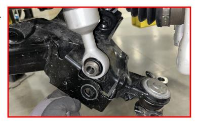
Install the factory lower shock bolt.
