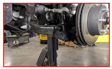
Carefully swing lower control arm out of the way.
