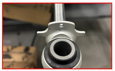
Install dust shield as shown, using provided bolt.
