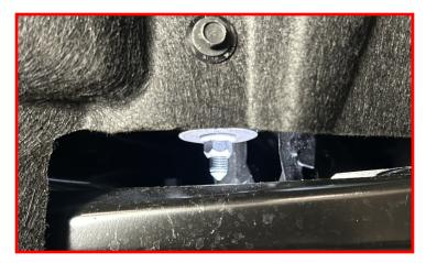
Install the inner fender liners.
