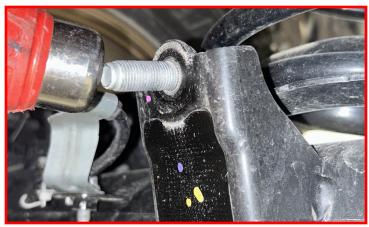
Install the sway bar bracket into the axle using the factory washer and nut on the bottom stud and the supplies M12 x 30mm flat head allen bolt in the top.
