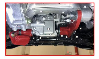
Lower the knuckle assembly down the other knuckle adaptor. Install the factory knuckle adaptor bolts.
