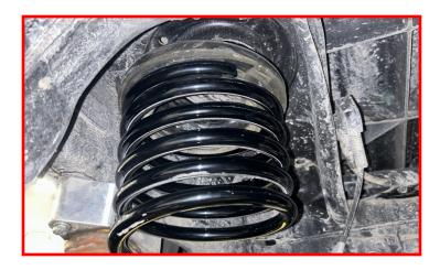
Install spring assembly into the axle side mounting point.
