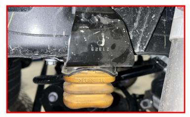
Remove the factory bump stop bracket from the frame.
