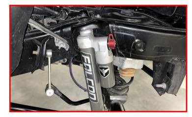
Install lower shock bushing onto factory axle stud. Install factory bolt into stud.
