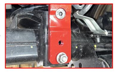
Install the supplied M12 washer and locking nut onto the backside of the factory sway bar mount.
