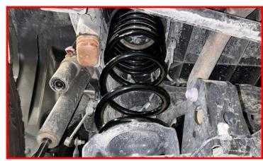
Falcon rear shock is provided with dust shield.
