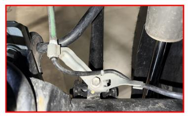
Remove the brake line bracket that is attached to the backside of the axle.
