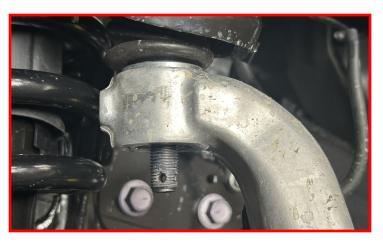
Remove the upper control arm pivot nut.
