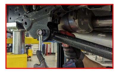
Disconnect sway bar from the axle on both the left and right hand sides.
