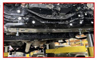
Slide the slots in the rear of the skid plate onto the exposed bolts.
