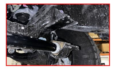
Install the core support nut.
