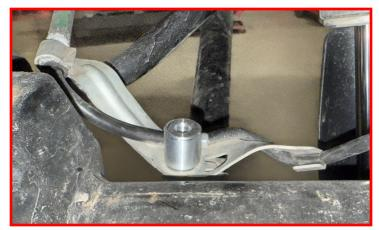
Install the appropriate bump stop pad on top of the axle housing and bump pad spacer.
