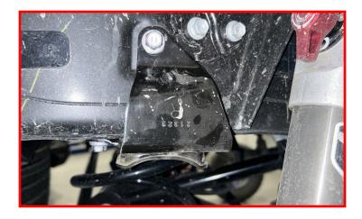
Install ReadyLIFT rear bump stop extension using the provided M8 X 45mm bolts, M8 washers and thread locker.
