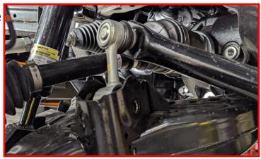
Guide the lower strut mount into the lower control arm pocket.
