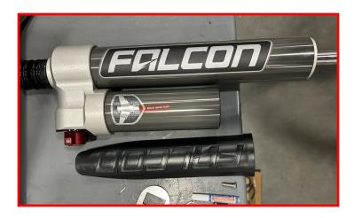
Dust shield will be installed on the bracket shown in the image. Dust shield will point away from shock lower eye.
