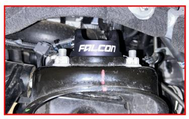
Install Falcon coilover assembly into Falcon top hat. Insert M16 bolt into the top hat and through the top of the coilover.
