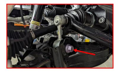
Loosen the inner lower control arm pivot bolts.
