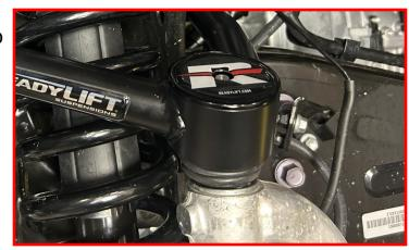
Install the supplied hardened washer onto the ball joint stud.
