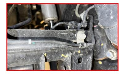
Place the bump pad spacer on top of the abs bracket on the front of the axle housing.
