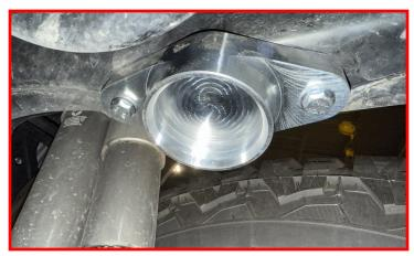
With the bump stop extension installed. Press the supplied bump stop into the extension.
