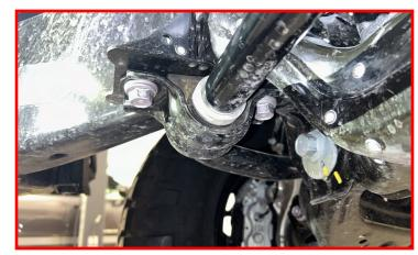
Carefully lower the sway bar down and out of the way.
