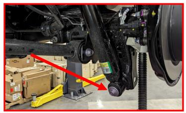
Ensure axle is supported and remove upper shock nut from frame. Remove lower shock bolt and remove shock from vehicle.
