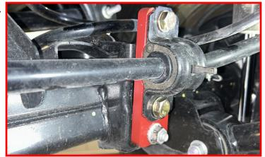
Install the brake line drop bracket into the factory location using the factory hardware.
