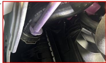
Remove the left (driver) side core support nut.
