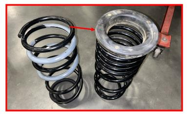
Install spring assembly into the top of the frame side factory mounting.
