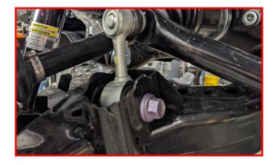
Remove the sway bar bolts from the frame.
