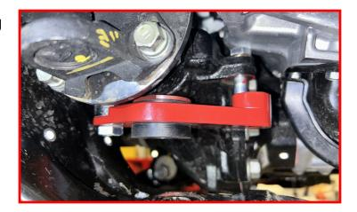
Lower the diff drop down and install the rear diff drop spacer between the rear diff drop and the diff housing.
