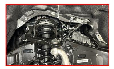
Use a flat blade screw driver or similar tool to pry the (3) upper control arm ABS brackets open.
