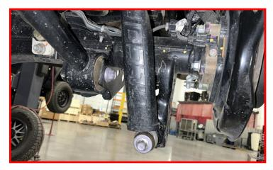
Remove factory bump stop and factory bump stop mount.
