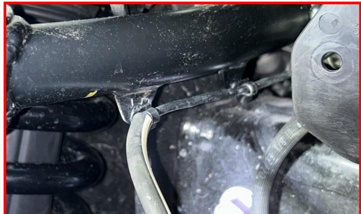
Install two of the **skid plate bolts** (removed on page 15) into the factory threaded holes in the transmission cross-member.
