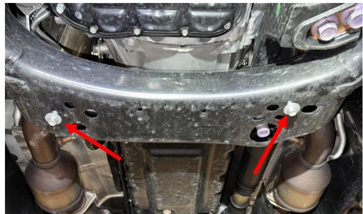
Make sure there is enough space between the washer and the crossmember surface to slide the skid plate in between.
