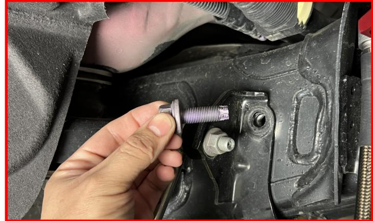
Using the factory sway bar bracket bolt and bolt hole, install the Falcon reservoir using the hole in the bracket. Ensure that the **reservoir mount spacer** is installed.
