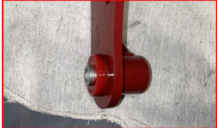
Install the **front diff drop spacers** on either side and ensure the large side of the spacer is touching the bushing.
