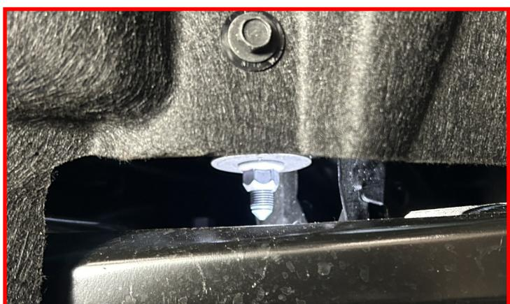
Install the supplied **M14 flange nut** onto the ball joint.
