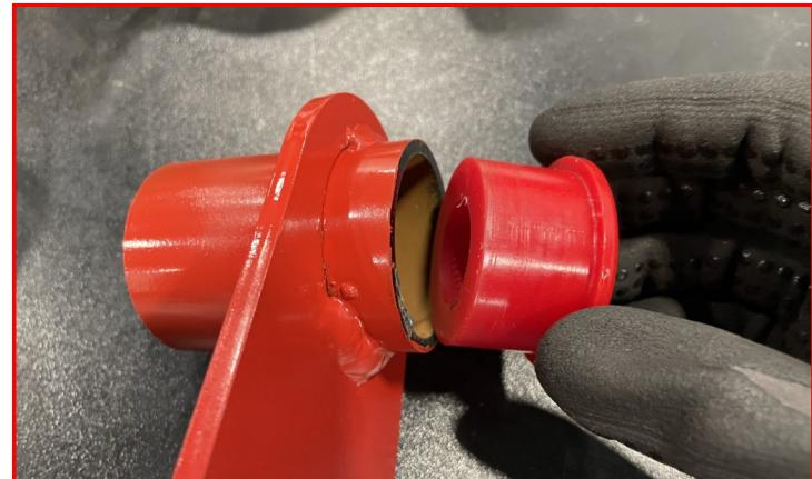
Press the **supplied crush sleeve** into the **bushings** and slide the **spacers** over the **sleeves**. The sleeve should be about flush with the spacers.
