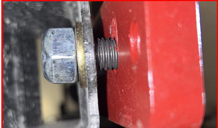
Install the sway bar onto the sway bar extension using the supplied M12 x 20mm hex head bolts, M12 washers and thread locker.
