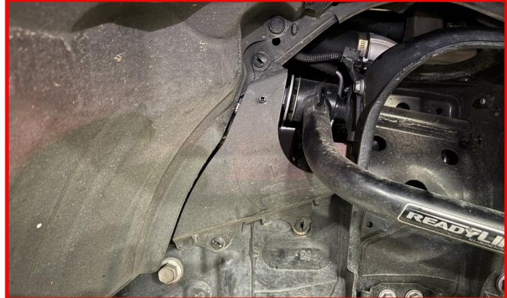
Loosen but do not remove upper control arm bolt.
