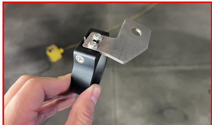
Install the reservoir into the reservoir clamp in the orientation shown. There should be roughly **3.25"** between the top of the reservoir and the reservoir clamp.
