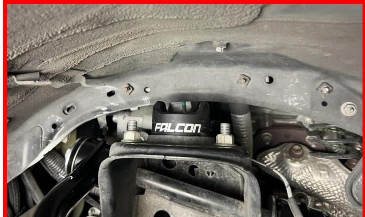
Install the Falcon Strut into the Falcon upper strut mount using the supplied bolt and nut.
