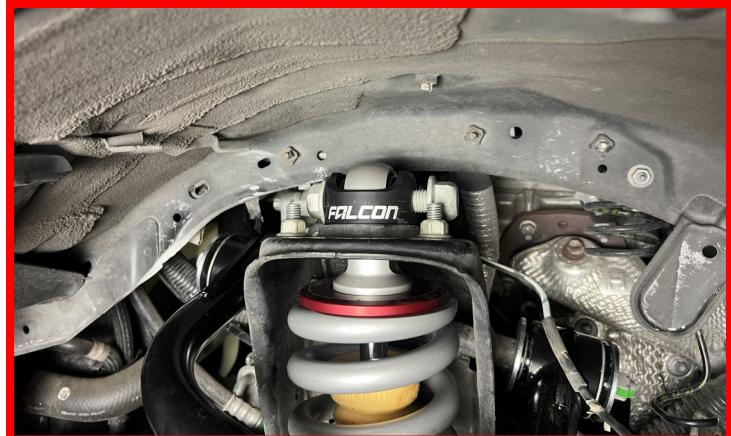
**NOTE:** the lower shock spacer has one chamfered edge. This edge will be installed facing the control arm.
