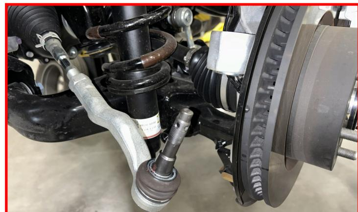
Remove lower control arm to strut bolt.
