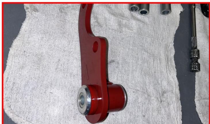
Install the diff drop into the frame side pocket in the factory orientation using the factory hardware.
