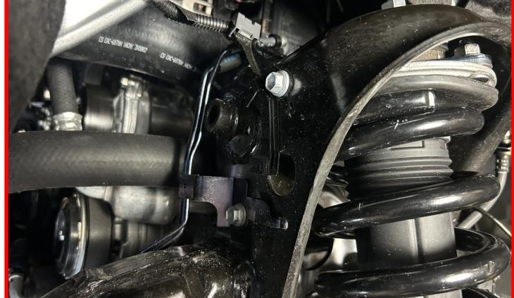
Install the ReadyLIFT upper control arm using the factory pivot hardware.
