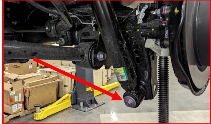
Loosen, but DO NOT REMOVE **upper shock nut**. Ensure axle is supported, and disconnect shock from axle stud.
