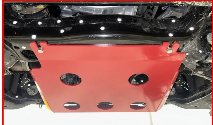
Use the two other factory bolts (saved from page 15) to secure the front of the skid plate to the front crossmember.
