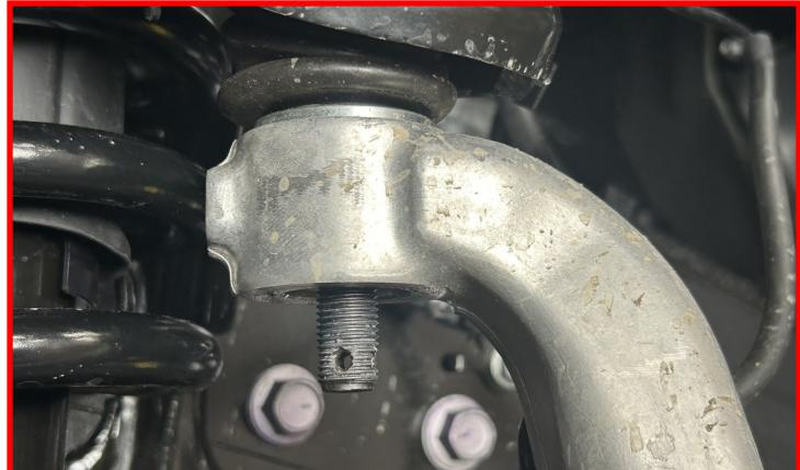
Remove the upper control arm pivot nut.
