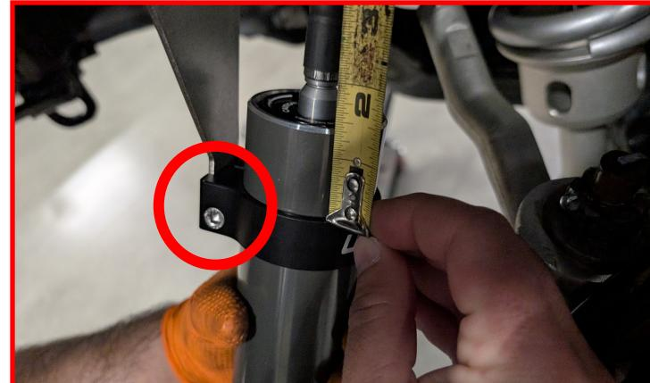
Install the reservoir mounting plate using the provided screws. Torque to **5 ft-lbs**.
