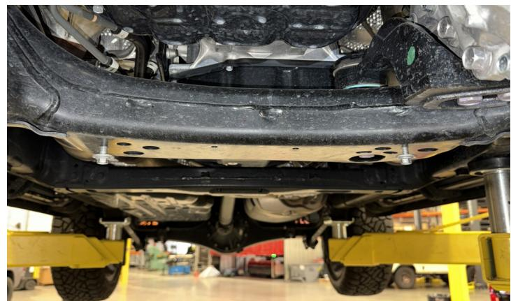
Slide the slots at the rear of the skid plate onto the loose bolts on the crossmember until the front of the skid plate rests against the front crossmember.
