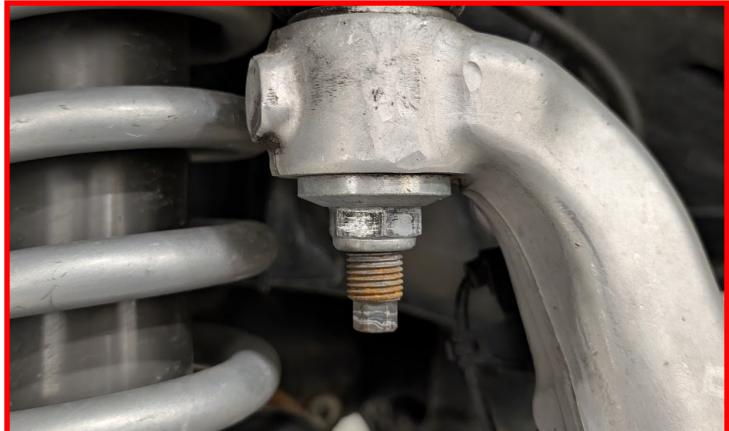
Remove the lower bolt from the sway bar link.
