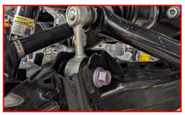
Remove the sway bar bolts from the frame.
