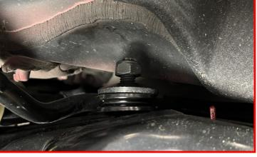
Install the Falcon shock onto the lower shock stud using the factory bolt.
