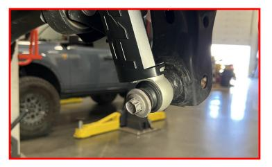
Remove the horizontal bolt holding the factory sway bar bracket to the frame.
