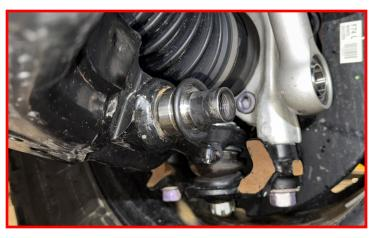
Install the lower strut eye onto the control arm stud, ensuring not to pinch the O-ring. The lower shock eye should fit over the small radius on the misalignment spacer.
