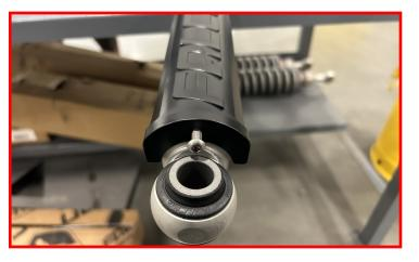
Install the alignment tab onto the Falcon rear shock using the provided hardware.
