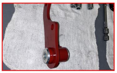
Install the diff drop into the frame side pocket in the factory orientation using the factory hardware.
