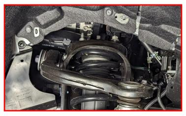
Slide lower strut off of the stud and remove strut from vehicle.
