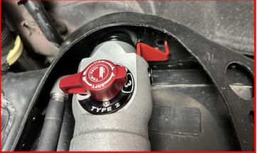
Install the upper shock bushing and washer onto the stud of the Falcon shock. The washer should be placed above the bushing, with the cupped side point down.
