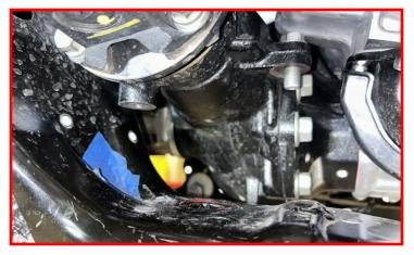
Lower the diff back down, this will allow clearance for the bolt to be remove.
