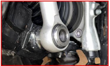
Install the factory bolt into the lower control arm stud.
