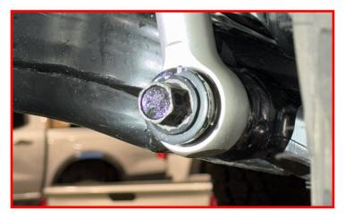
Install the tie rod into the knuckle. Torque nut to 65 ft-lbs. Install cotter pin.
