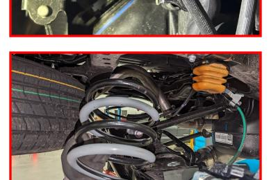
Install spring assembly into the top of the frame side factory mounting.
