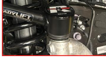
Install the supplied hardened washer onto the ball joint stud.
