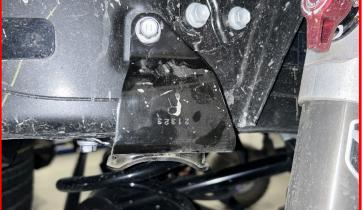
Install the supplied Falcon bump stop into the ReadyLIFT bump stop cup. Ensure that the bump stop is fully seated into the cup.
