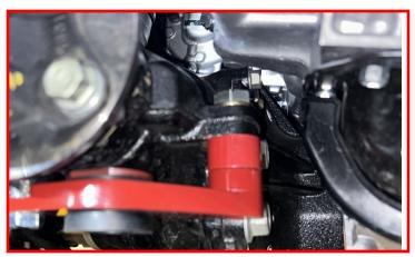
Place the 1/8" thick laser cut washer under the rear diff drop and lower the differential down on top of the washer.
