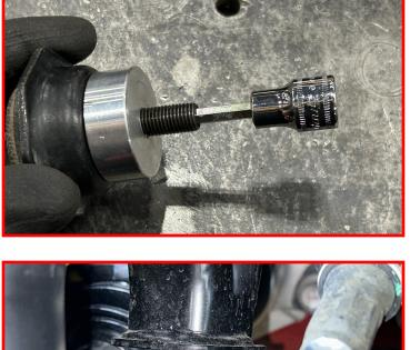
Install bump stop with extension back into vehicle.
