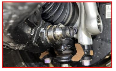
Install the O-Ring into the groove on the misalignment spacer. The two O-rings are interchangeable.
