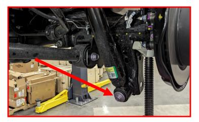
Loosen, but DO NOT REMOVE upper shock nut. Ensure axle is supported, and disconnect shock from axle stud.
