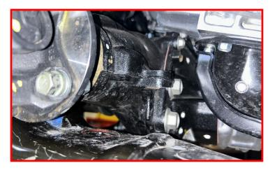
Install the supplied M12 x 60mm hex head bolt , washer and thread locker through the diff from top to bottom.
