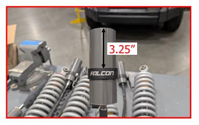
Install the Falcon Rear shock into the hole in the frame shock mount. Ensure that the alignment tab goes into the appropriate hole.
