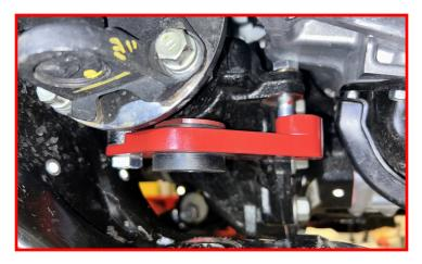
Lower the diff drop down and install the rear diff drop spacer between the rear diff drop and the diff housing.
