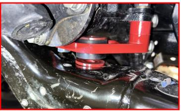
Install the supplied M14 x 40mm hex head bolt, flat washer, 3/8" thick laser cut washer and thread locker through the crossmember and into the rear diff drop.
