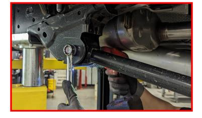
Disconnect sway bar from the axle on both the left and right hand sides.
