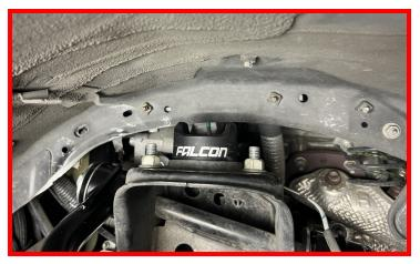
Install the Falcon Strut into the Falcon upper strut mount using the supplied bolt and nut.
