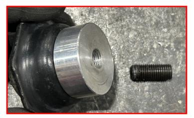
Install stud using internal hex.
