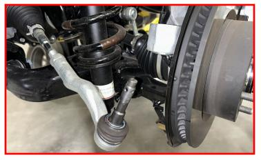
Remove lower control arm to strut bolt.
