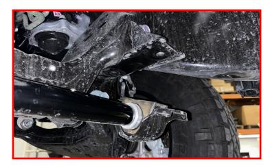
Install the core support nut.
