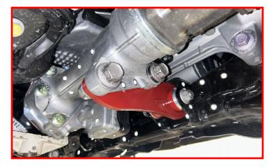
Install the supplied M16 locking nuts and washers.
