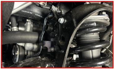
Install the ReadyLIFT upper control arm using the factory pivot hardware.
