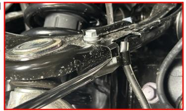
Remove the wire from the bracket.
