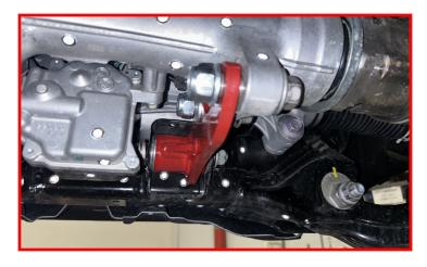
Remove nut holding rear differential mount to frame crossmember.
