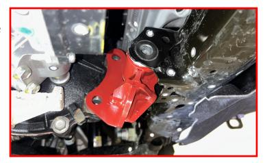
Install the supplied M14 x 55mm hex head bolt, flat washer and thread locker.
