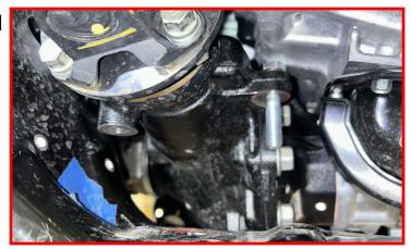
Assemble ReadyLIFT rear differential mount as shown.
