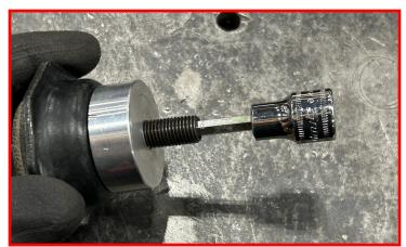
Install bump stop with extension back into vehicle.
