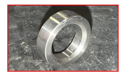
On the control arm stud, install the spacer with the chamfered edge toward the control arm, covering the radius on the base of the stud.
