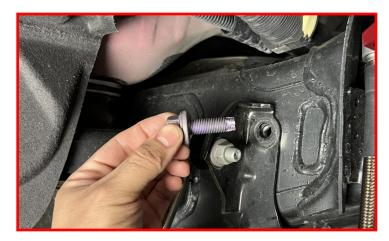
Using the factory sway bar bracket bolt and bolt hole, install the Falcon reservoir using the hole in the bracket.
