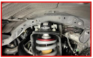
NOTE: the lower shock spacer has one chamfered edge. This edge will be installed facing the control arm.
