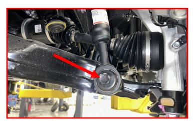
Remove the four (4) upper strut nuts and remove strut from vehicle.
