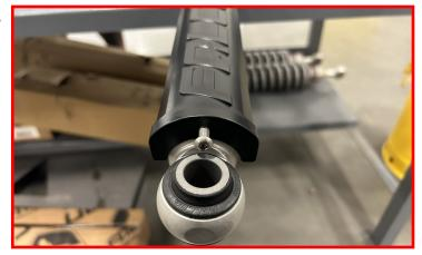
Install the reservoir attachment clip to the reservoir clamp as shown, using the provided bolts. Ensure that the bent portion of the bracket is angled toward the clamp.
