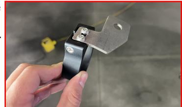
Install the reservoir into the reservoir clamp in the orientation shown. There should be roughly 3.25" between the top of the reservoir and the reservoir clamp.
