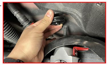
Install the nut onto the stud of the Falcon rear shock.
