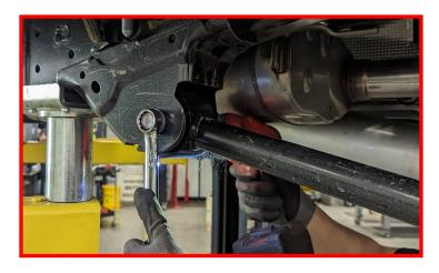
Disconnect sway bar from the axle on both the left and right hand sides.
