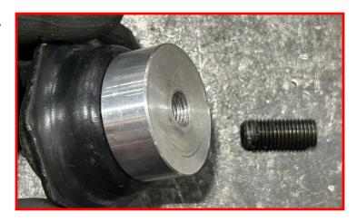
Install stud using internal hex.
