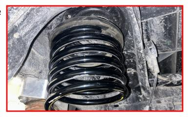
Install spring assembly into the axle side mounting point.
