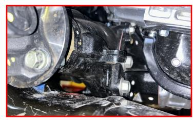
Install the supplied M12  $\times$  60mm hex head bolt , washer and thread locker through the diff from top to bottom.
