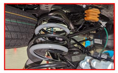
Remove the isolator from the factory spring and install isolator onto ReadyLIFT spring.
