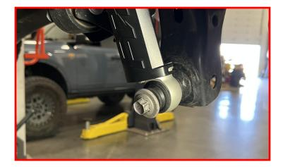
Remove the horizontal bolt holding the factory sway bar bracket to the frame.
