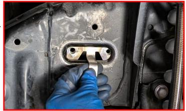
Install the reservoir mounting plate to the backing plate using the provided bolts.
