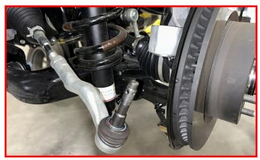
Remove lower control arm to strut bolt.
