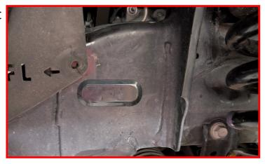
NOTE: The reservoir will be mounted in this slot as shown in the image. When completing the following steps, ensure that the reservoir can be mounted in this position without twisting or straining the oil line.
