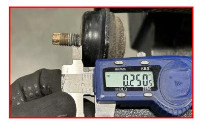
Thread bump stop into bump stop extension until it sits flush against the aluminum.
