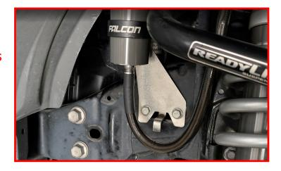
Install Falcon clamp ring onto the shock reservoir. The "U" shape should be pointed towards the oil line extending out of the reservoir.
