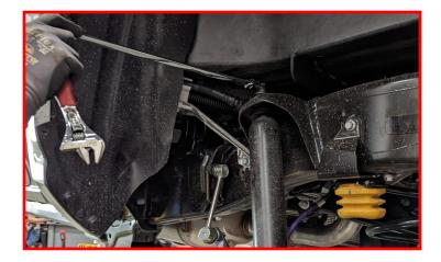
Remove the bolt holding the brake line bracket to the axle.
