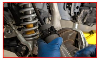
Measure 1.5" from the edge of the reservoir to the edge of the falcon clamping ring.
