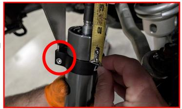
Install the reservoir mounting plate using the provided screws. Torque to 5 ft-lbs.
