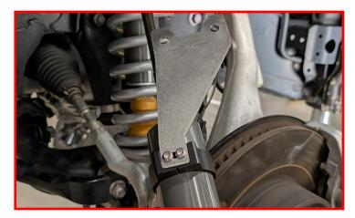
Insert the backing plate into the slot on the frame. The tongue portion should be sticking out of the frame. Be careful to ensure you don't drop the bracket into the frame.
