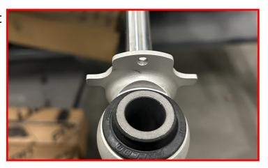
Install dust shield as shown, using provided bolt.
