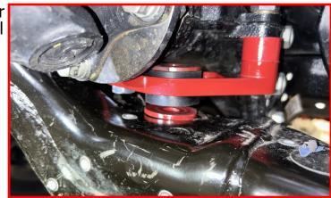
Install the supplied M14 x 40mm hex head bolt, flat washer, 3/8" thick laser cut washer and thread locker through the crossmember and into the rear diff drop.
