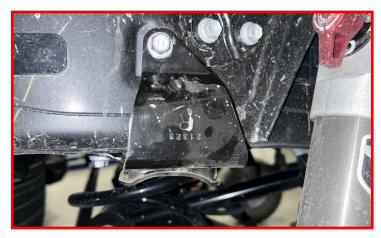
Install the supplied Falcon bump stop into the ReadyLIFT bump stop cup. Ensure that the bump stop is fully seated into the cup.
