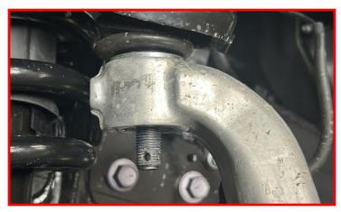
Remove the upper control arm pivot nut.
