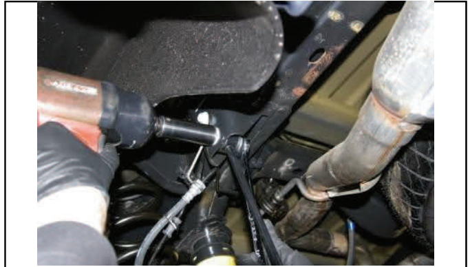
Disconnect upper sway bar end links.
