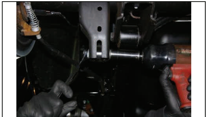
Remove lower shock mounting hardware.
