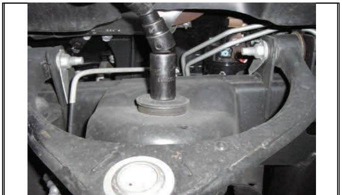
Disconnect upper shock mount and bushing
