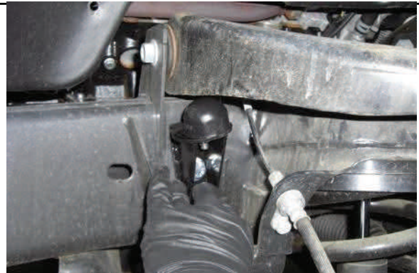
Note: pass/dr side brackets are specific. Tighten once aligned
