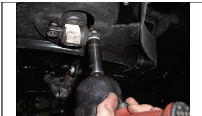
Disconnect lower shock mounting bolts.
