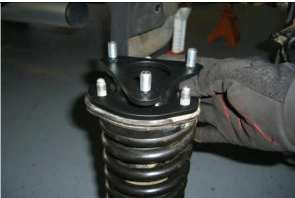
Lower suspension, remove strut, install extension w/OE nuts
