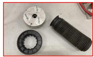
Install the ReadyLIFT leveling spacer between the top hot and spring isolator.
