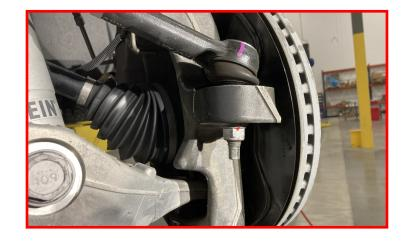
Install the sway bar link in the control arm using the factory hardware.
