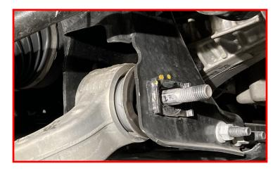
Remove the lower shock mount nut.
