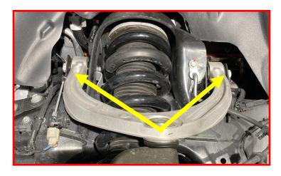
Loosen the nuts retaining the upper shock mount. Do not remove at this time.
