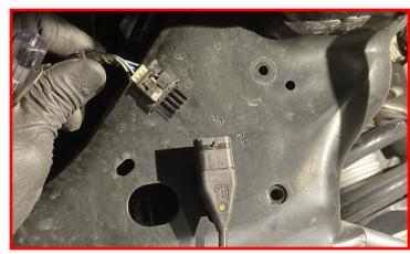
Remove the Active Terrain pigtail from the crossmember.
