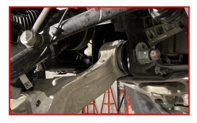
Press the Active Terrain pigtail into the crossmember and plug in the Bilstein Active Terrain wire. Reinsert the safety clip.
