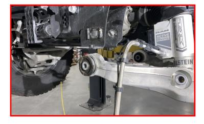
Remove the lower shock bolt.
