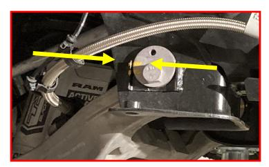
Remove the lower control arm nuts.
