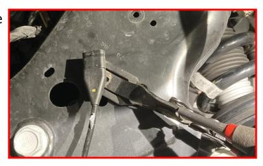
Remove the bolt securing the shock reservoirs.
