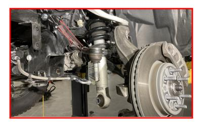
Remove the reservoir and shock assembly from the vehicle.
