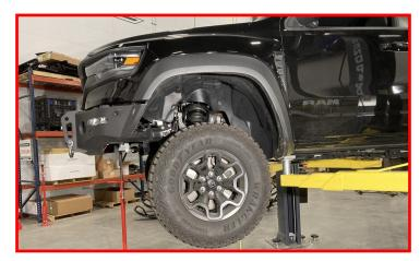
Lower the vehicle and move the steering wheel side to side to settle the front suspension. Then, begin tightening the following bolts:
