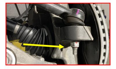
Strike the knuckle with a dead blow hammer or similar to dislodge the taper from the knuckle.
