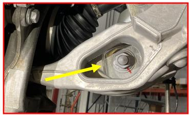
At this point, support the knuckle/lower control arm at or near the ball joint and remove the lower control arm bolts.
