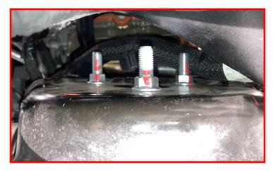
Lower shocker mount bolt Torque to 102 lb ft.
