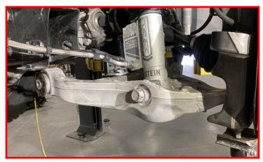
Install the factory lower control arm cam spacer and nut.
