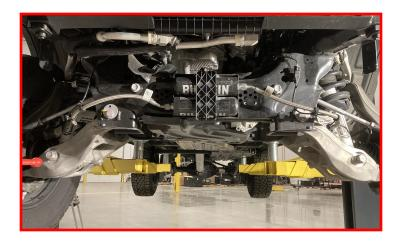
Unplug the Bilstein Active Terrain wire by first releasing the safety clip followed by the plug.
