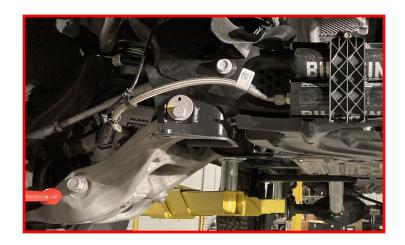
With the steering wheel centered, turn the tie rod ends until the tires are straight. If the steering wheel is not centered properly, the ABS/traction control lights may activate. Reconnect the battery ground terminal. Start the vehicle and turn the steering wheel lock to lock and verify all clearances between tire, body and suspension components. Adjust as necessary.
