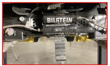
Install the factory lower shock bolt and nut. Do not tighten at this time.
