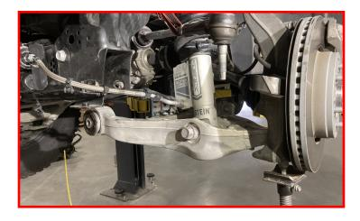
Install the factory lower control arm bolts.
