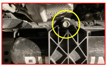
Loosen the upper control arm mounts.
