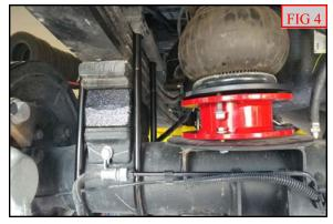
Install the lower shock mount. Do not tighten at this time. Install the rear wheels. Lower the vehicle to the ground. Torque the lug nuts to the wheel manufacture specs. Jounce the vehicle a few times to settle to the new ride height. Torque lower shock mount to 65 ft-lbs.
