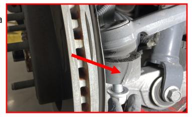
Remove the ABS wire harness from the upper control arm and the brake line. Cut the Christmas tree clip off the harness.
