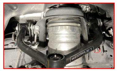
Install the upper ball joint to the knuckle using the supplied nut spacer followed by the castle nut. Torque the nut to 65 ft-lbs and install the cotter pin.
