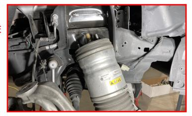
Install the air strut spacer and torque the factory nuts to 30 ft-lbs.
