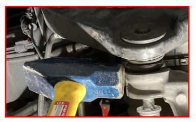
Remove the two bolts and nuts securing the upper control arm at the frame.
