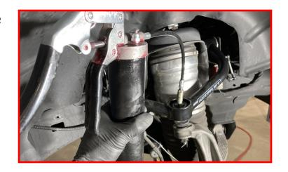
Install the outer tie rod and torque the nut to 60 FT-LBS.
