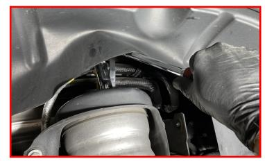
Remove the lower air strut nut and bolt from the control arm.
