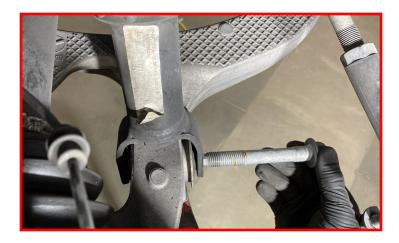
Remove the air strut from the vehicle.
