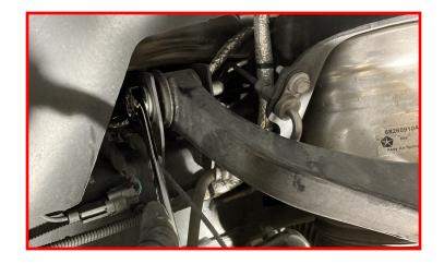
Remove the three nuts securing the air strut to the frame.
