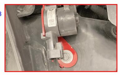
Attach the ride height sensor link to the ball stud on the ReadyLIFT upper control arm.
