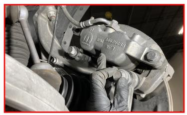
Install the nut on the cv shaft and torque to 185 FT-LBS.
