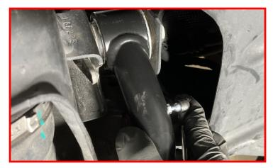
Plug the factory harness into the ride height sensor and replace the red safety clip.
