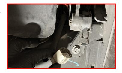
Remove the three push-in zip ties holding the air line to the frame and cut them off the air line.
