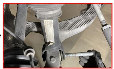
Install the supplied ReadyLIFT upper control arm using the factory hardware at the frame. Leave the hardware loose.
