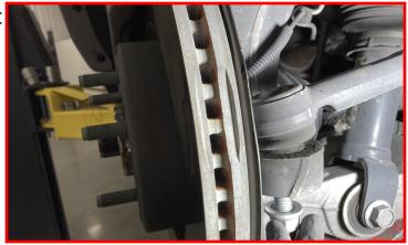
Install the rotor and torque the factory retaining bolt to 7 FT-LBS.
