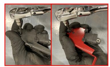
Install the ride height sensor and relocation bracket using the factory bolt using 8 FT-LBS.
