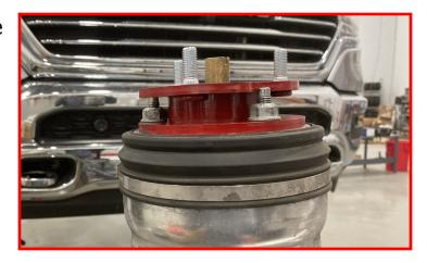
Install the air strut by inserting the studs through the upper mount. Loosely install the supplied nuts on the air strut spacer studs.
