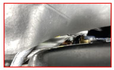
Use a couple cable ties to secure the air line and remove stress at the fitting/ pressure relief valve interface.
