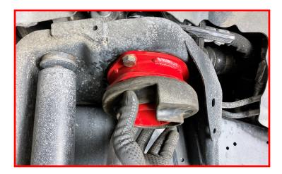
Reinstall the spring into the isolator. Make sure to seat the end of the coil to the backstop on the isolator to maintain the correct spring position. Once the spring is reinstalled raise the jack again to compress the system.
