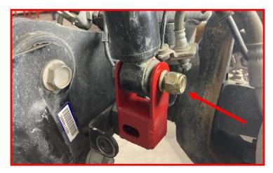
Install the lower bolt of the shock extension using the factory 21mm bolt.
