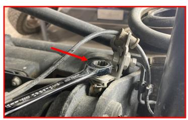
Loosen and then re-tighten the track bar bolts at the frame and axle ends.
