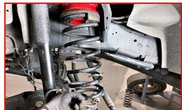
Install the front shock extension to the lower mount of the shock. Rotate the shock 90 degrees to allow for install.
