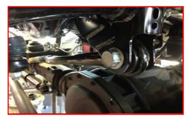
Loosen and re-tighten the rear radius arm bolt.
