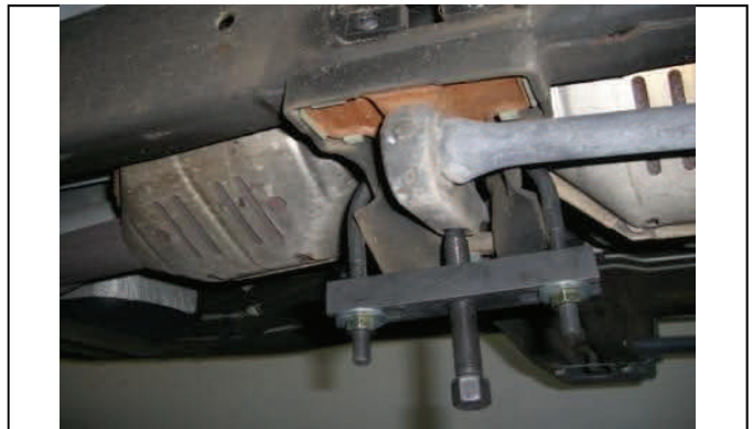
Attach u-bolt over cross member and install tool
