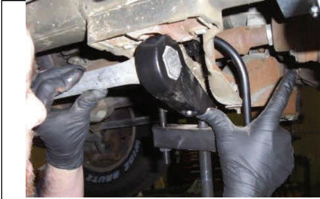
Install new torsion key and reload tool
