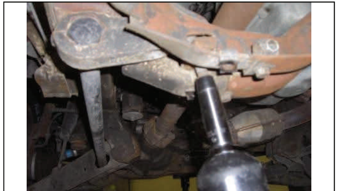
Remove torsion key adjuster bolt
