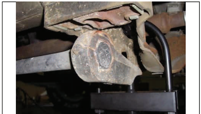
Unload tool and torsion bar will lower, remove torsion key
