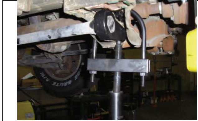
Adjust torsion key tool enough to replace keeper block
