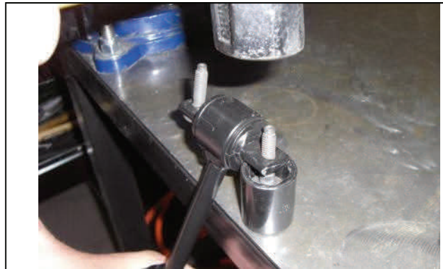
Hammer out OE mounting bolts
