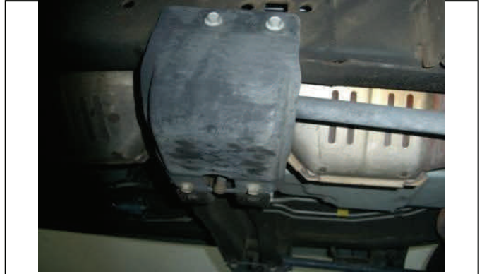
Locate cross member cover and remove bolts
