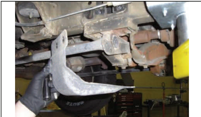
Cover will expose torsion keys
