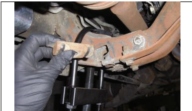
Adjust tool enough to remove keeper block
