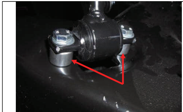
Install shock spacers as shown
