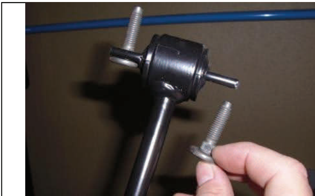
Remove both bolts and use new provided hardware
