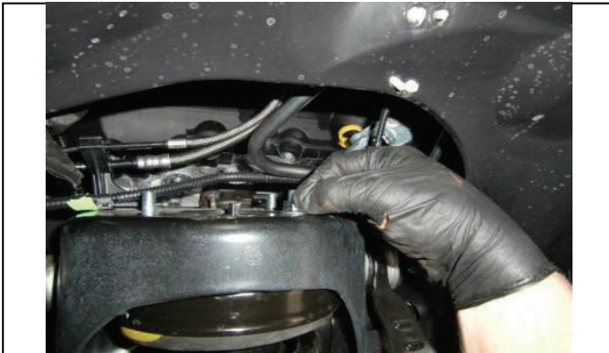
Use provided hardware to re-attach top of strut to vehicle.
