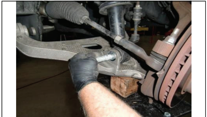
Reconnect lower strut mount and torque to spec.
