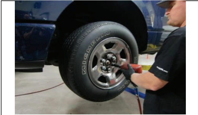
Lift vehicle securely and remove wheels/tires.
