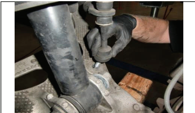
Reconnect lower sway bar end links and torque to spec.
