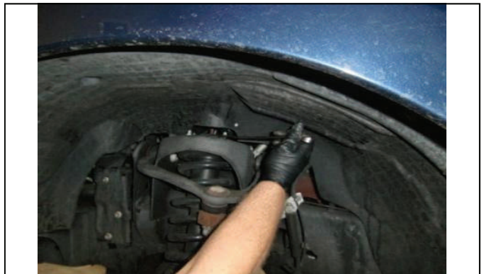
Loosen upper strut mount nuts.
