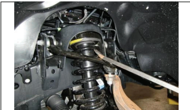
Use jack and pry bar to reattach upper ball joint to spindle.
