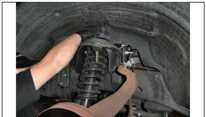
Remove top strut mount nuts and remove assembly.
