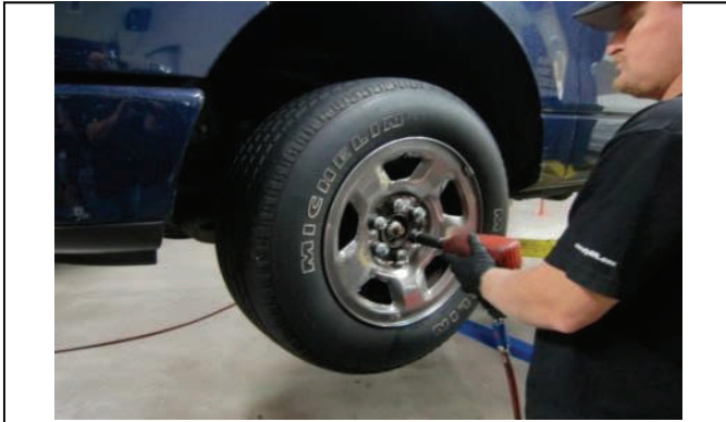
Lift vehicle securely and remove wheels/tires.
