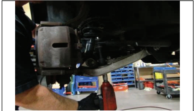
Remove lower sway bar end link hardware.
