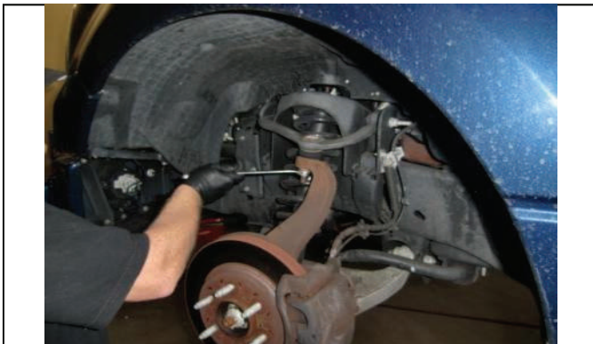
Loosen upper ball joint nut, but do not remove.
