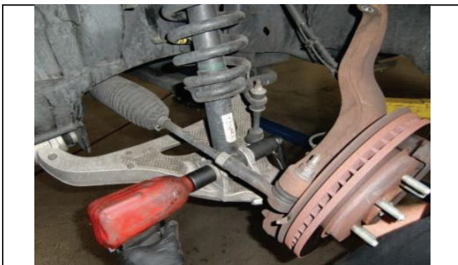
Loosen lower strut bolt/nut and remove.
