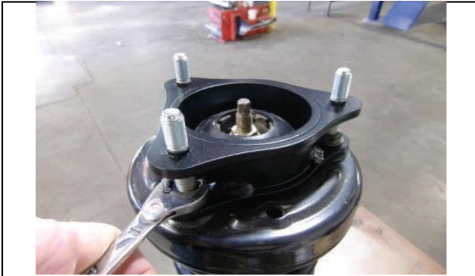
Shown 66-2058 studs line up w/ OE strut. Attach w/ OE nuts
