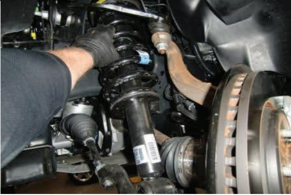
Remove strut assembly from vehicle
