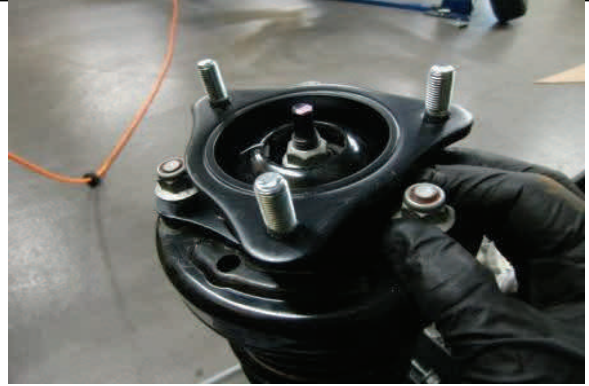
Install new strut extension with OE hardware and tighten.
