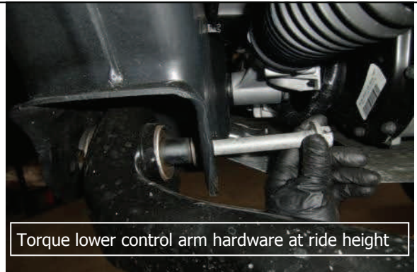
Lift lower control arm into position and reinstall bolts.
