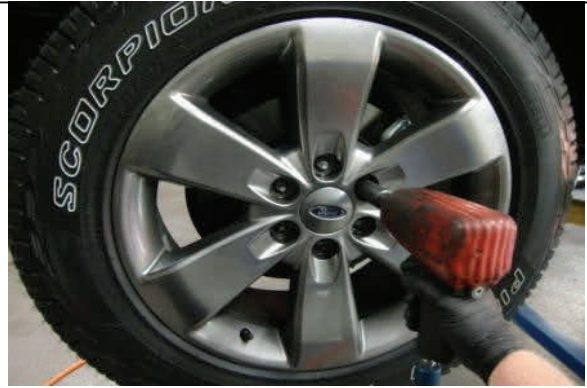
Remove front wheels/tires, support suspension with jack.
