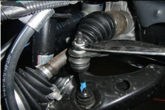
Disconnect upper sway bar end links.
