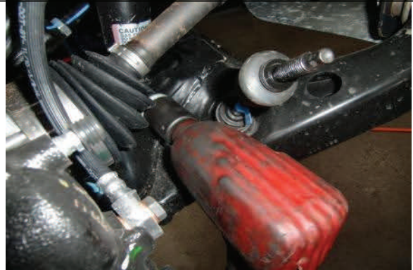
Disconnect and remove lower shock bolt and nut.
