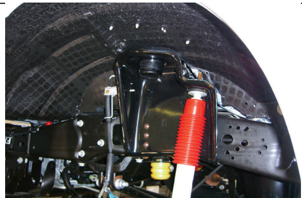
Carefully lower axle and remove coil spring
