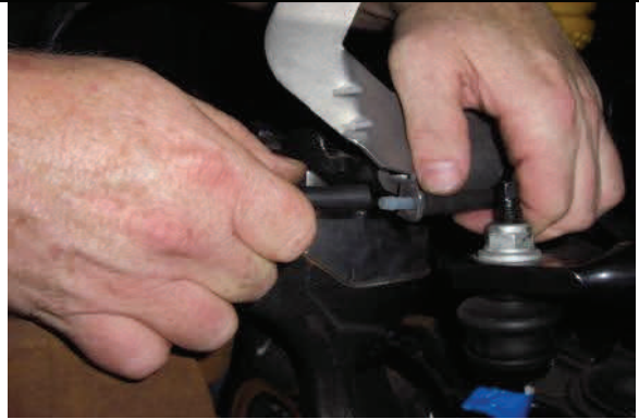
Disconnect vacuum line and clip from brake bracket
