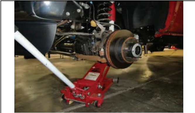
Support front axle with floor jack(s).
