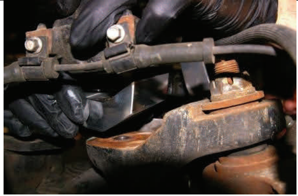
Place billet spacer on axle under spring perch
