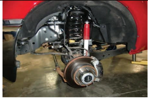
Remove front wheels and tires.
