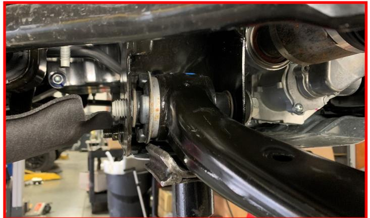
Install the supplied alignment cam plate over pivot bolt so pin fits in existing small hole in frame and then install alignment eccentric cam nut by threading bolt into nut.
