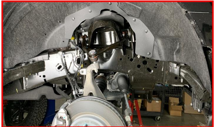
Install the top strut spacer onto the strut assembly using the factory nuts.
