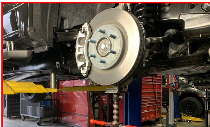
Remove the **sway bar end link** from the knuckle. Retain the factory mounting hardware.
