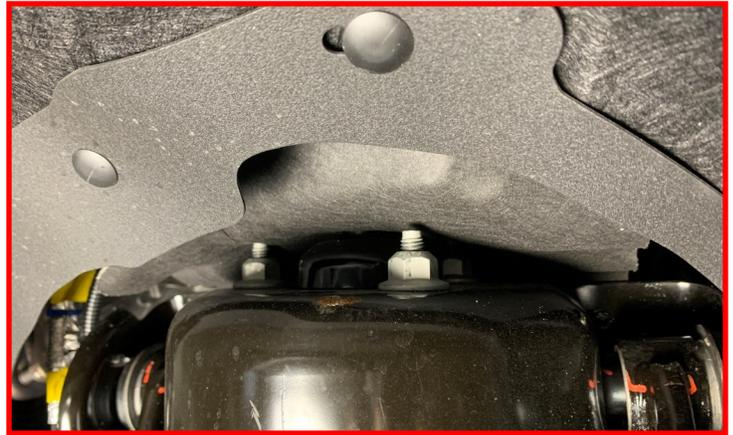
Remove the **lower strut nuts**. Retain the
