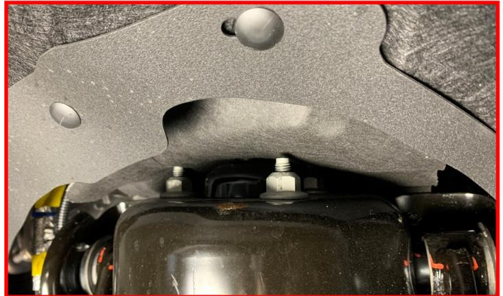
Remove the **lower strut nuts**. Retain the
