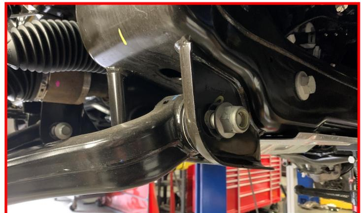
Remove the lower control arm pivots from the frame side pivot pockets.
