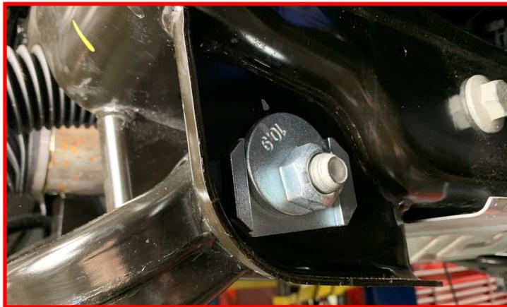
Tighten the top strut nuts.
