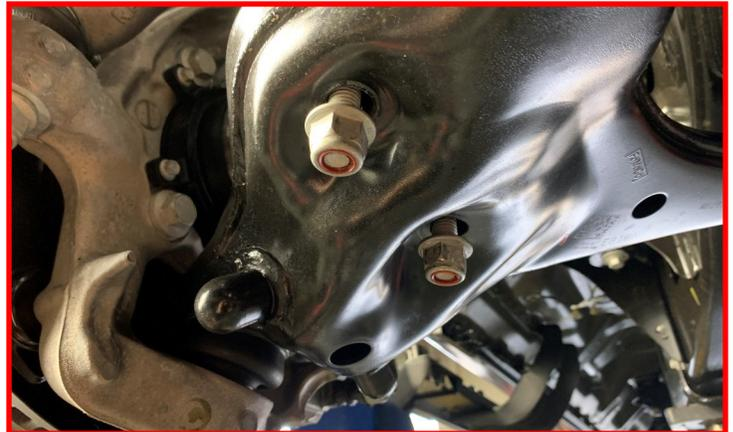
Loosen and remove the **lower control arm
