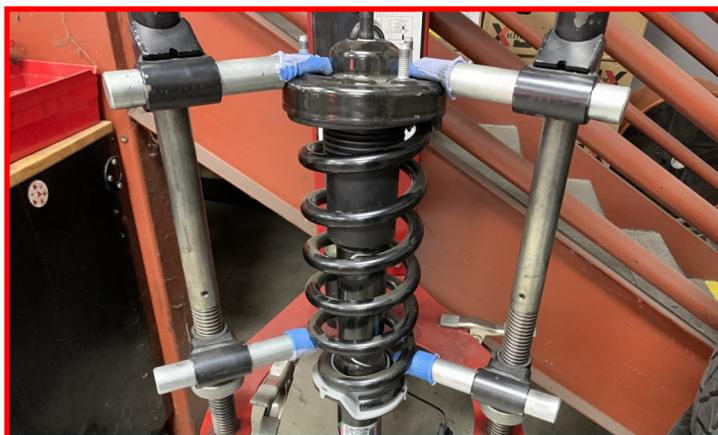
Torque the top strut hardware to **35 ft-lbs.**
