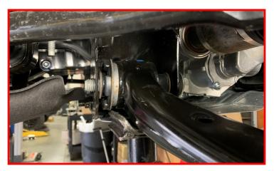
Install the supplied alignment cam plate over pivot bolt so pin fits in existing small hole in frame and then install alignment eccentric cam nut by threading bolt into nut.
