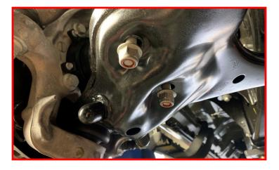
Loosen and remove the lower control arm pivot bolts. Retain the factory bolts.
